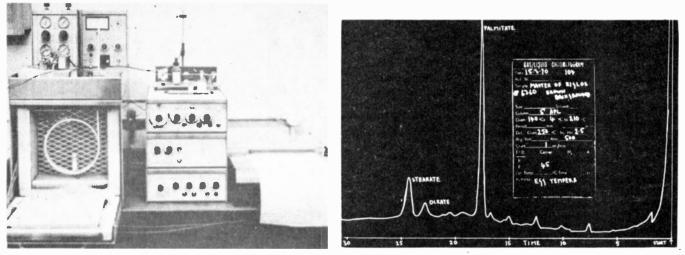
Fig.5. This Pye gas-chromatograph is used to provide chemical analyses of painters' mediums. Its chart output for egg tempera is given here (as recorded for an analysis of 'The Crucifixion'' by the Master of Ruglos).
