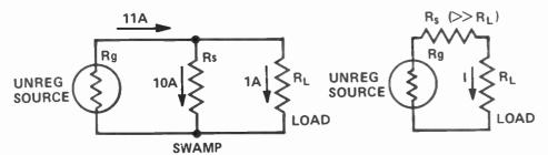
Fig. 1. Regulation can be slightly improved by: (a). Voltage regulation – an additional shunt load.
