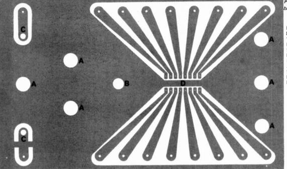
Printed circuit layout for basic unit. (shown full-size)
