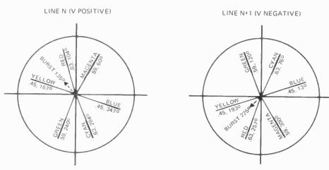
Fig. 29. Chroma and burst vectors on successive lines for colour bar pattern.
