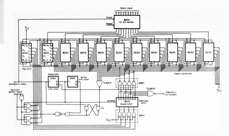
capacity of the memory is 80-bits (8 x 10), eleven CAMs are employed which together have a capacity of 88-bits (11 x 2 x 4). The eleventh CAM has been called the tag CAM because it keeps track of the locations within the memory which are occupied, and allocates a new address for acceptable information.
