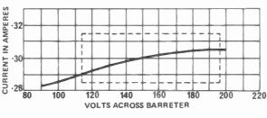
Fig. 2 (a). The barretter tube regulates by the increase in resistance with temperature (and hence current) of an iron-wire filament.
