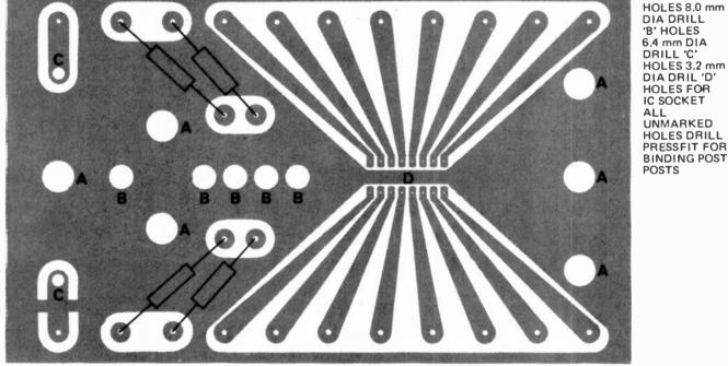
Printed circuit layout for modified (BCD) unit (shown full-size). Note resistors. These should be about 470 ohms (330 - 1k will do) and connect the LED's to the appropriate binding posts.
