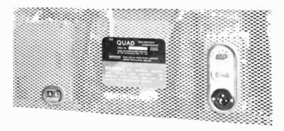
The warning is needed — there's 5000 volts behind the mesh panel.
