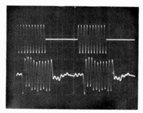
Tone burst 8 kHz – 94 dB peak sound pressure level.
