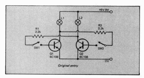
THIS CIRCUIT was thought up by Mr T. Tuck of Salisbury, South Australia. It's purpose is to indicate which of two switches is first depressed.
