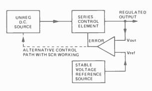
Fig. 9. Generalized diagram of active feedback type regulator.
