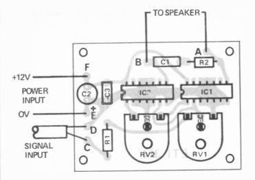
Fig. 3. Component overlay.
