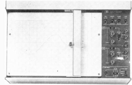
Model 7015A Laboratory X-Y Recorder.
