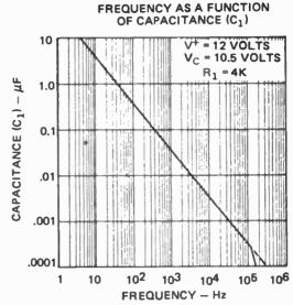
capacitor  $C_1$  should be switched to provide a number of ranges. A value of 100 pF will allow a frequency of 1 MHz to be reached if  $R_1$  is near the minimum of its permitted range. The values of  $C_1$  may be increased by factors of ten; for example,  $0.1\mu$ F may be used to obtain an output at about 1 kHz and  $10\mu$ F may be used to obtain a frequency of 10 Hz or less. The writer has used a  $10\,000\mu$ F capacitor to obtain a frequency of less than 0.001 Hz.
