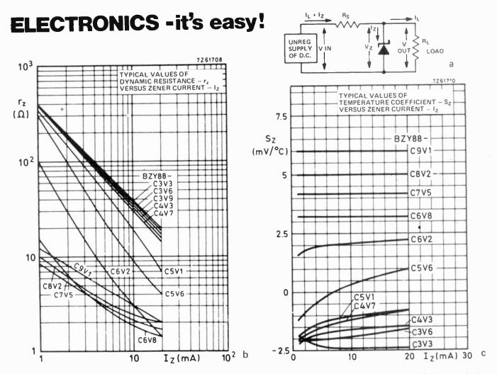
Fig. 6. (a) Typical Zener diode regulator. (b) dynamic resistance of BZY88 series Zeners. (c) temperature coefficients of BZY88 series diodes.
