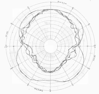
Horizontal pattern at two metres (input, one-third octave filtered pink noise). [ 1 kHz ----- ], [ 4 kHz - . - . - . ], [ 8 kHz - .. - .. ], [ 16 kHz - 0 - 0 - 0 ].
