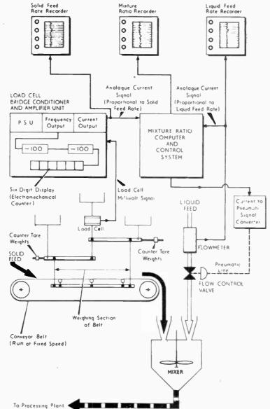
ratio value and the desired pre-set value generates a corrective feedback signal, which is used to adjust a liquid flow control valve and thus restore the solid/liquid proportion to the correct value at all times.
