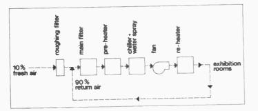
Fig.3. Block diagram of arrangement used to clean and correct humidity and temperature of air.
