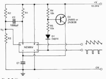
Fig. 6. Falling ramp generator.
