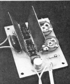
Fig. 4. Heatsink (two required) to be attached to either side of both IC's as shown in main picture.
