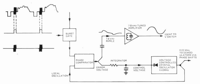
Fig. 25. The phase lock loop by which the reference oscillator phase is controlled by the burst.
