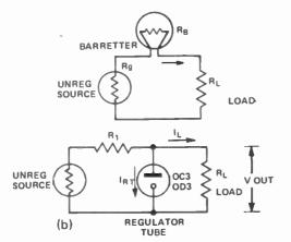
If a constant current through the load resistance is required a similarly crude method is to place the load in series with a resistor that is much greater than the load value – as shown in Fig. 1b. It can be seen (from Ohms law) that I will now remain constant over a wider range of  $R_{\perp}$  variation.
