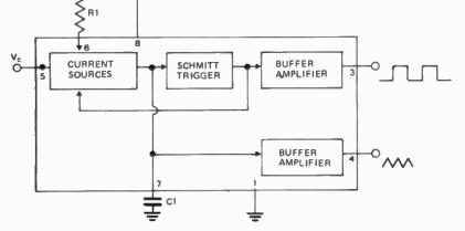
Fig. 2. Basic circuit of the NE566V in block form.
