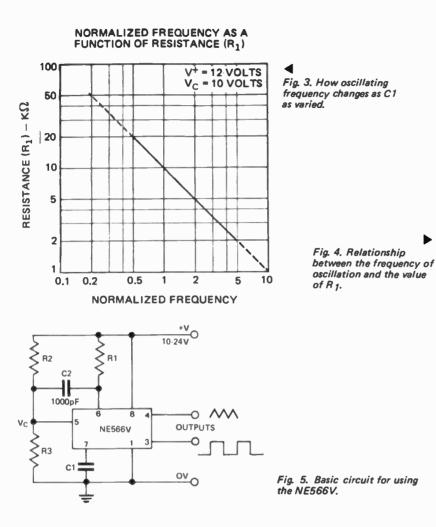
this range the frequency of oscillation is proportional to the difference between the voltage at pins 5 and 8. When  $V_{\rm c}$  becomes very close to V+, however, oscillation ceases.
