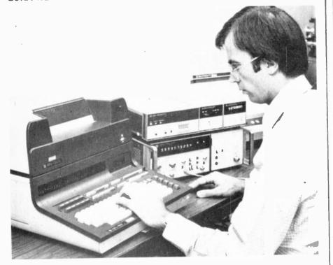
A quiet new thermal printer, Model 5150A from Hewlett-Packard, accepts data from BCD (binary coded decimal) or ASCII sources and prints up to 20 columns of alphanumeric information. Modular in construction, it is available in many different configurations including some in which it functions as an instrument-system controller.
