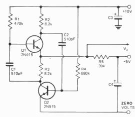
Fig. 1. This circuit supplies well-shaped square-waves.
