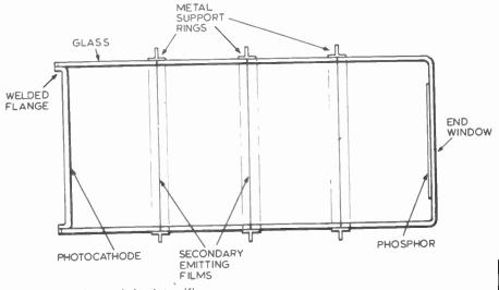
Fig. 6. Secondary emission intensifier.
