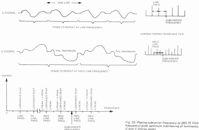
A PAL COLOUR television signal is similar to a monochrome signal except that it includes a high frequency subcarrier on which the colour-difference signals are
