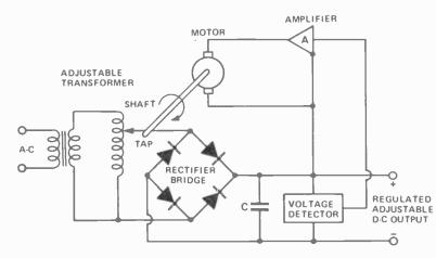
Fig. 8. Superior regulation is obtained by using feedback – as demonstrated by this electromechanical form of regulator.
