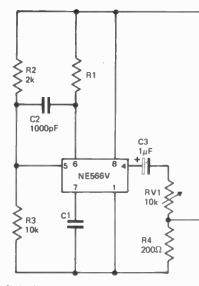
Fig. 10. A circuit for converting triangular waves to sine waves. The only active devices required are a Signetics NE566V and a Signetics NE511B.
