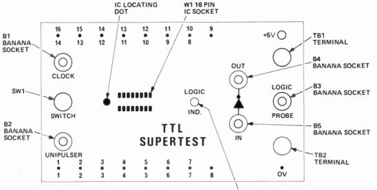
Front panel layout of basic unit – the associated printed circuit board is shown page 5. Scale approx 70% – use pc board as guide for marking out hole centres etc.
