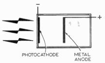
Fig. 3. Construction of a simple photocell showing photocathode and anode.
