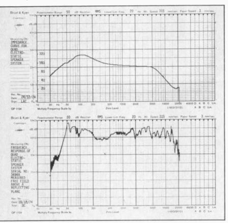
deviation of less than  $\pm 5$  dB. It would be regarded as being flat by most purists. Obviously, off-axis in either the vertical and to a much lesser extent in the horizontal plane, the frequency response drops with increasing frequency but this is true of most other speaker systems as well.
