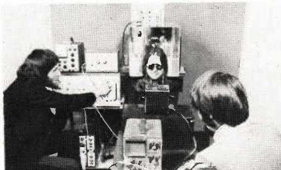
Fig. 9(b). Recording the change in VECP when viewing a flashing stimulus through various additional lenses. Subject is using her left eye (the right is covered). Metal shield prevents stray pick up. Xenon Strobe Stimulus is directly in front of subject. Bottom left is X-Y chart recorder and above it is the response averaging computer (being adjusted).
