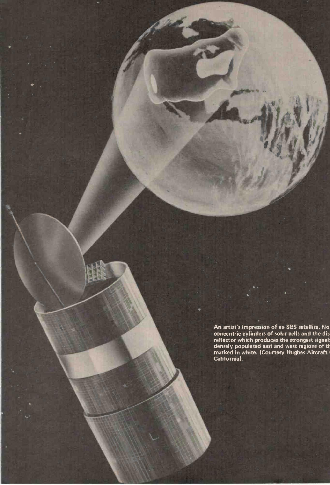
An artist's impression of an SBS satellite. Note the concentric cylinders of solar cells and the dish reflector which produces the strongest signals in the densely populated east and west regions of the USA, marked in white. (Courtesy Hughes Aircraft Co., California).
