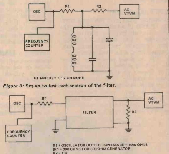
Figure 3: Set-up to test each section of the filter.
