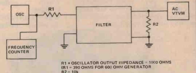
Figure 4: Set-up required to plot overall response of the filter.
