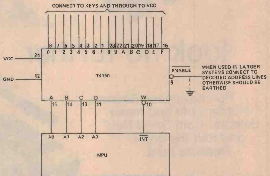
plexers, 16 lines each and using more address lines to enable each multiplexer one at a time (i.e. short form ASCII-6 bits can be encoded by four multiplexers, four lines address all multiplexers and the other two lines select only out of four multiplexers to be enabled).
