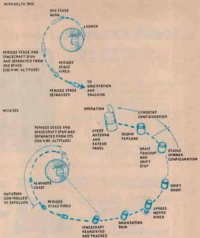
Figure 3: It is hoped to launch the SBS craft using the Shuttle, but as the Shuttle may not be available early enough for the first launchings, provision has been made for a rocket launch. In both cases the satellite will take up a geosynchronous orbit.
