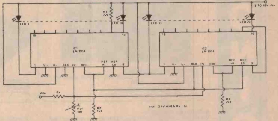
Figure 8. Dot mode voltmeter with 20 LEDs. Full scale is 2.4 V when Rx is zero.
