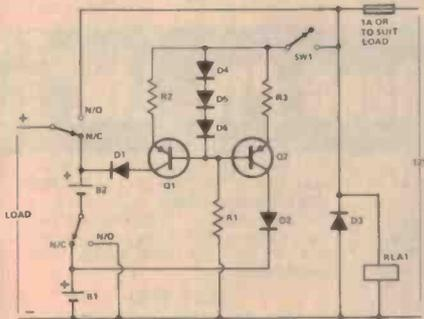
Quite a number of portable appliances use battery supplies for which NiCad batteries are ideally suited. This circuit, from Ron Smith of Rockhampton QLD, charges two sets of 6 V NiCads from a 12 V source. This allows a 12 V NiCad battery supply to be charged from the 12 V supply in a car or boat, and used as an emergency power source. It would be useful for charging NiCad batteries used in handheld transceivers.
