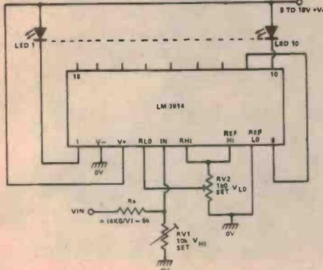
Figure 5. Expanded scale dot mode voltmeter for the 10 - 15 V range.
