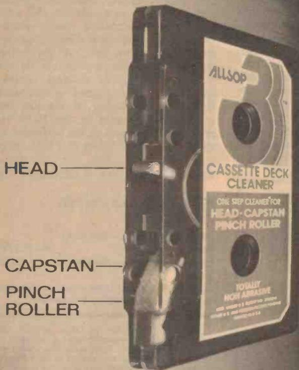
The ALLSOP 3 not only restores fidelity to the head, but cleans the two major trouble spots, the capstan and the pinch roller, at the same time. Dirt build-up on the pinch roller and capstan are the leading causes of 'tape-eating' and slippage. ALLSOP 3 efficiently does the lot with a new patented, totally non-abrasive scrubbing and wiping action, not by scraping with abrasive tape. It's surprisingly simple and very effective.
