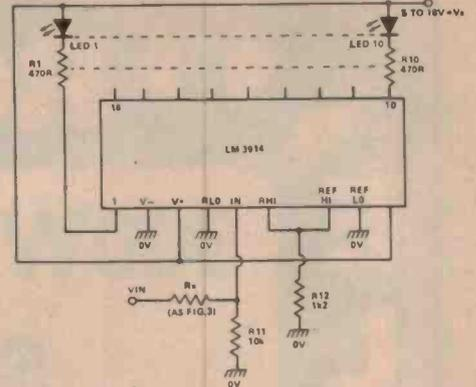
Figure 7. Bar display voltmeter with common LED supply.
