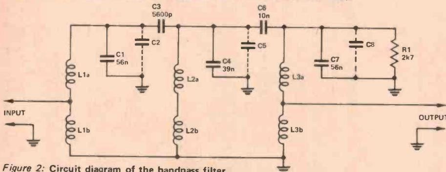
Figure 2: Circuit diagram of the bandpass filter. The inductors, L1, L2, L3 are 88 mH toroids or pot cores (see text). Refer to text for C2, C5 and C8.
