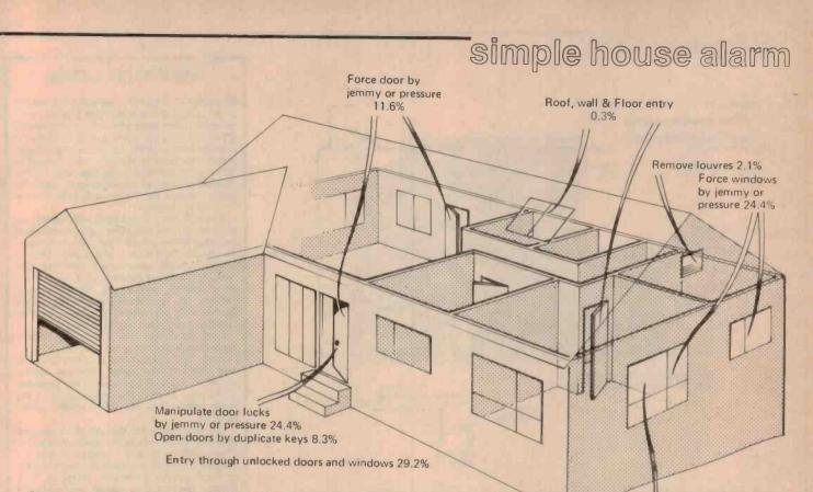
Figure 1. This illustration shows the various ways in which criminals will enter a house. In particular, note the high percentage of entries made through locked doors and windows. The necessity for adequate locking arrangements is obvious. ETI acknowledges the assistance of the Crime Prevention Dept. of the NSW Police in making these statistics available.
