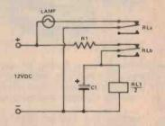
When the power is first applied, the capacitor charges through R1. When the voltage across the capacitor has risen sufficiently, the relay operates. Power is then disconnected from the relay coil, and C1, by the relay contacts in series with the supply and the capacitor starts to discharge through the relay coil. When the voltage across the coil falls below the 'hold in' voltage, the relay drops out. This is one flash cycle.
