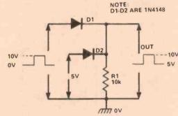
Figure 6. The effect of feeding a pulse to one input and a dc voltage to the other input of a two-input dlode OR gate.
