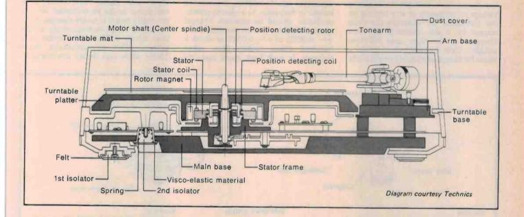
THE BASIC REQUIREMENT of any record player assembly is that the turntable shall rotate noiselessly, at the required speed without any short-term or long-term variations in this speed. This sounds a simple enough requirement, yet sophisticated, modern players contain quite complex circuitry with large numbers of integrated circuits and discrete components; indeed, the circuitry is too complex for us to reproduce in full for any of the latest players mentioned in this article!
