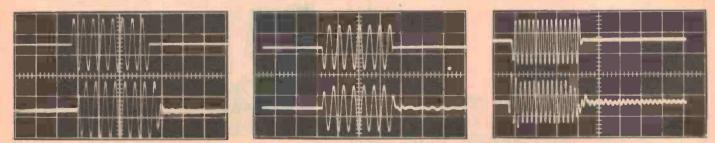
Tone burst response oscillographs of the Model A-2375 loudspeakers, measured with respect to 90 db steady-state spl at 2m on axis, LEFT: at 100 Hz, (20 ms/div, 80 dB spl). CENTRE: at 1 kHz (2 ms/div) and RIGHT: at 6.3 kHz (0.7 ms/div).
