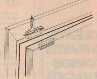
Door protection - the reed switch is set into the architrave.
