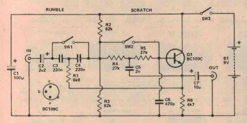
Circuit of the Scratch and Rumble filter. This unit may be mounted on matrix board and mounted inside your amplifier — don't forget two will be needed for stereo. If you construct it as an outboard unit it should be mounted in a metal box and connected into your amplifier system with short lengths of shielded cable. It may be connected between the "preamp out" and "main in" sockets.
