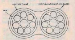
POLYURETHANE COATEO COPPER WIRE 0.55mm DIA x 16 Figure 6. The Trio-Kenwood low capacitance tone arm wire. in these models consists of 'Penta-Litze' wire of the cross section shown in Figure 6; this has a very low capacitance and therefore signal losses and cross talk are minimised.
