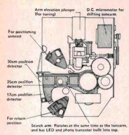
Figure 7 (a). The automatic mechanism of Trio-
