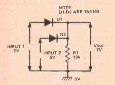
Figure 5. When a dlode OR gate is used in the linear mode, Vout equals the greater of the two inputs.
