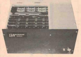
11 slot backplane, fully card guided. 15 amp power supply, fan, key switch, bench mount, rack mount, annodised aluminium. 5 edge connectors standard. S 100 Bench Kit \$345. S 100 Rack Kit \$306. 6800 Bench Kit \$370.00. 6800 Rack Kit \$330, Assembled prices add \$100.
