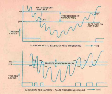
ABOVE: Trigger Window Diagram. The width of the trigger window will greatly affect the accuracy of measurement when attempting to take a reading on a signal having a high frequency component. Set the trigger window wide for best results.
