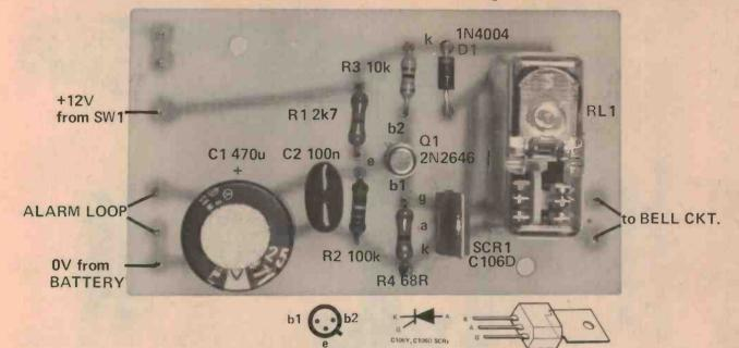
switches gets moist — a leakage path may develop in parallel with the switch (that's why you keep those leads apart) and if this happens when the control unit can tolerate more than a few hundred ohms, that switch can be opened without triggering the alarm !
