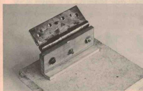
attached to the moving wing of the hinge by three clamping screws tapped into the wing.
