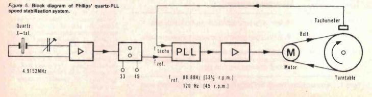
positioning, variable pitch controls with a LED speed display, etc. The AF877 offers lower wow and flutter (see Table 1) and completely silent operation is achieved by the use of touch control switches; at the end of each disc, a photoelectronic sensor detects the acceleration of the arm as it follows the run-out groove and the arm is automatically returned to its rest. The AF977 employs a quartz stabilised speed system.
