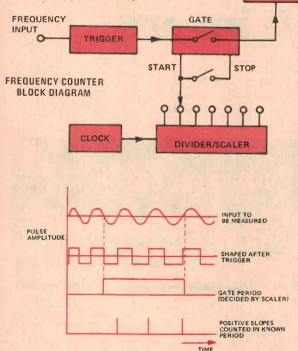
determined by the output from a divider/scaler driven by a very stable, accurate clock oscillator. A number of outputs from the divider/scaler may be selected to vary the period the gate is open. Usually, a number of decade steps are provided.
