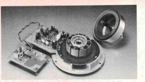
The Hall Effect dc drive motor and control electronics from Pioneer's model PL-560 turntable.
