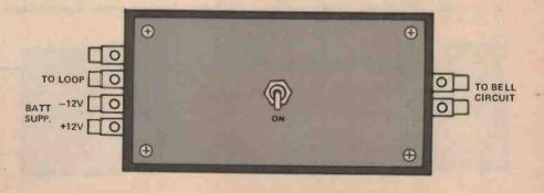
External connections to the unit are made via the two plastic screw-terminal blocks.
