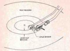
Figure 10. The Sharp Optonica 'APLD' sensor system is mounted on a separate arm adjacent to the tone arm.
