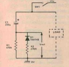
Figure 14. A basic variant of the Figure 12 circuit.
