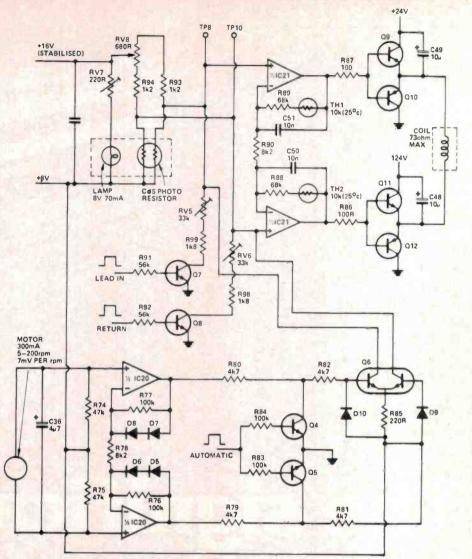
Figure 13. The Pioneer PL-L1000 turntable has a tangential tracking tone arm employing an optical tracking system. This is the optical sensor circuitry.
