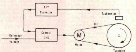
Figure 4. The Philips 'direct control' system employs belt drive for the platter and servo feedback to the motor control circultry via a tachometer sensing the platter speed.
