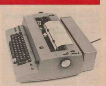
The typewriter that talks. Two researchers at Macquarie University have modified this IBM Selectric to provide a speech output corresponding to each key depressed. The box houses the electronics. All mechanical work, including modifications to the typewriter, was carried out by Ingram Paterson of the School's mechanical workshop.
