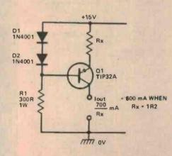
Figure 11. A simple and very useful current generator.
