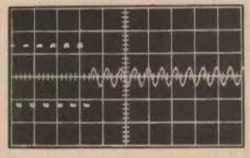
Transient overlaad recover test results for the RX1000. Overload of 10 dB re rated power into 8 ohm load, both channels driven. Overload duration: 20 ms; rep. rate: 512 ms.
