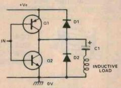
Figure 17. An example of the use of diodes to protect the complementary emitter follower output stage of a power amplifier that is used to drive an inductive load.
