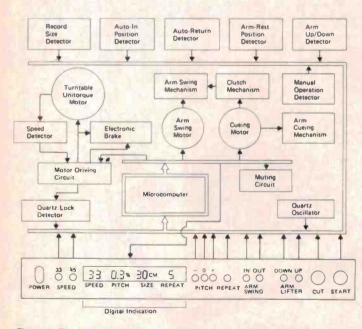
Figure 8. Block diagram of Hitachi's HT-860 microcomputer controlled deck.
