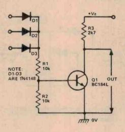
Figure 2. The diode OR gate can be converted to a NOR type by feeding its output through a translstor, as in (a) above, or through an IC inverting stage, as in (b) below.
