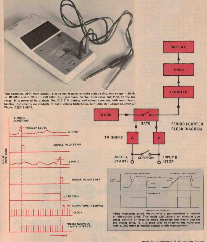
usually provided with a 'slope selection' control which determines whether the trigger operates on the positive or negative slope — (a), or (b) respectively in the diagram.
