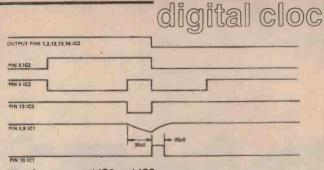
Waveforms around IC2 and IC3.
