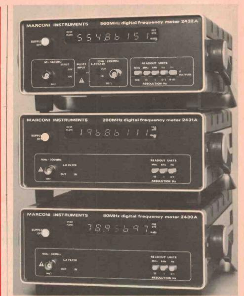
These three counters were recently added to the range of instruments offered by AWA. Made by Marconi Instruments, each features an eight digit display and a switchable low-pass filter. First in the range is the low cost model 2430A. It covers 10 Hz to 80 MHz and has three selectable gate times. The model 2431A (middle) covers 10 Hz to 200 MHz while the top-line 2432A includes a prescaler that permits measurements to 560 MHz, plus five selectable gate times.
