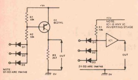
Figure 4. The diode OR gate can be converted to a NAND type by feeding its output through an inverting stage using either a transistor, as In (a) at left, or an IC as in (b) at right.
