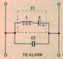
Figure 3. The large value capacitor, C1, will effectively bypass low frequency interference but its high series inductance, L, will prevent the bypassing of high frequency interference. A smaller value capacitor, C2, usually a ceramic type with a low series inductance, will bypass the high frequencies effectively. 2N2646 BOTTOM VIEW
