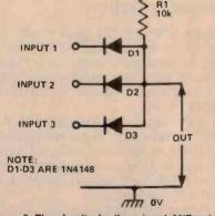
Figure 3. The circuit of a three-input AND gate. The number of inputs can be increased by adding extra diodes.
