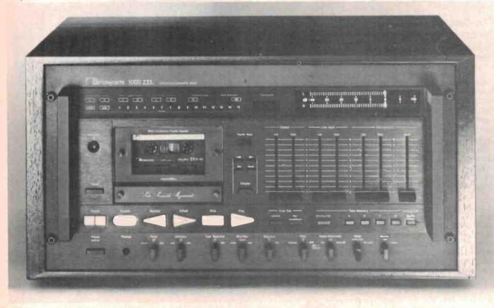
The 1000ZXL has a microprocessor which independently controls tape head azimuth, bias, recording level and equalisation to optimise these parameters for the particular tape actually running in the machine.
