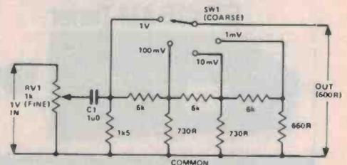
Figure 9. Practical 600R output attenuator network for a modern sine/square generator. RV1 gives fine control. SW2 gives coarse control.
