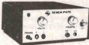
Just the thing for the hobbyists and experimenters bench. A handy kit featuring a 1.25V. to 16V. @ 1A. power supply, a 1 watt amplifier with HI & LO inputs. Comes with a sturdy metal case, easy to build.
