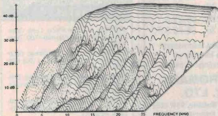
Spectral decay plot to 25 kHz.
