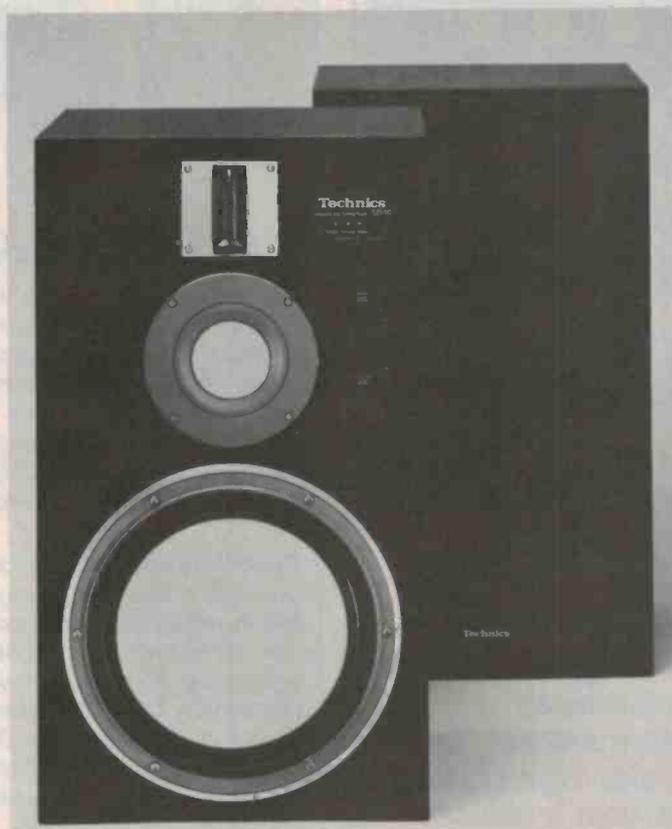
and this shows how the resonance problems were minimised and the total voice coil power dissipation rating increased as a result. The 80 mm mid-range driver is built on the same principles but the voice coil here is a more conventional 50.5 mm in diameter. The mid-frequency driver covers the frequency range 450 Hz to 5 kHz, and the top end of the response is provided by a leaf tweeter whose frequency response extends to beyond 100 kHz.
