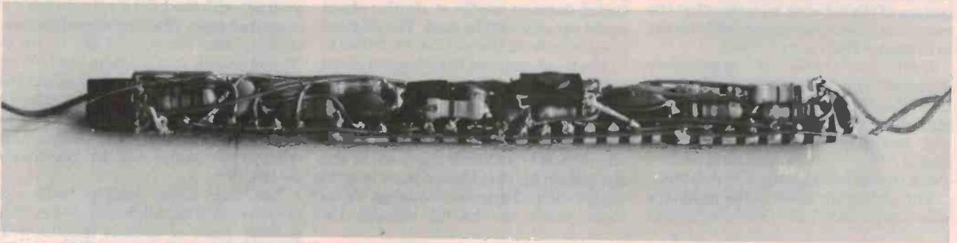
Close-up of the completed unit. Connections to the probe tip and the touch contact pins are to the left, power supply connections to the right. All the components are wired directly in place and small gauge insulated hookup wire used for interconnections. The ICs are glued end-to-end to form a solid
