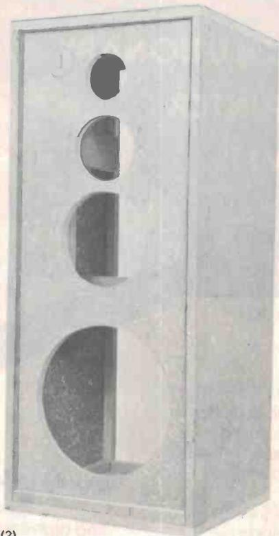
(2) The baffens for the midrange-tweeter enclosure are fitted to the box next, followed by the first (larger) front panel.
