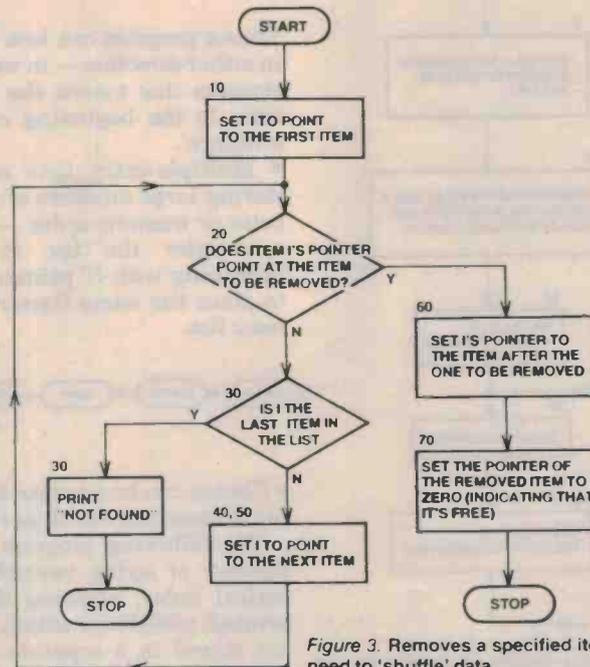
Figure 3. Removes a specified item — without the need to 'shuffle' data.
