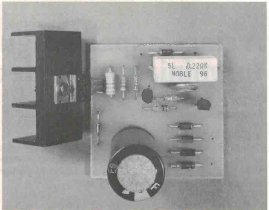
Construction is very simple — as you can see! The pc board is not absolutely essential, but convenient. The trimpot, RV1, visible just adjacent to the 0.22 ohm 5W resistor (R3), is adjusted to provide a nominal 12 Vdc at the output terminals under no load. Adjustment is relatively non-critical.
