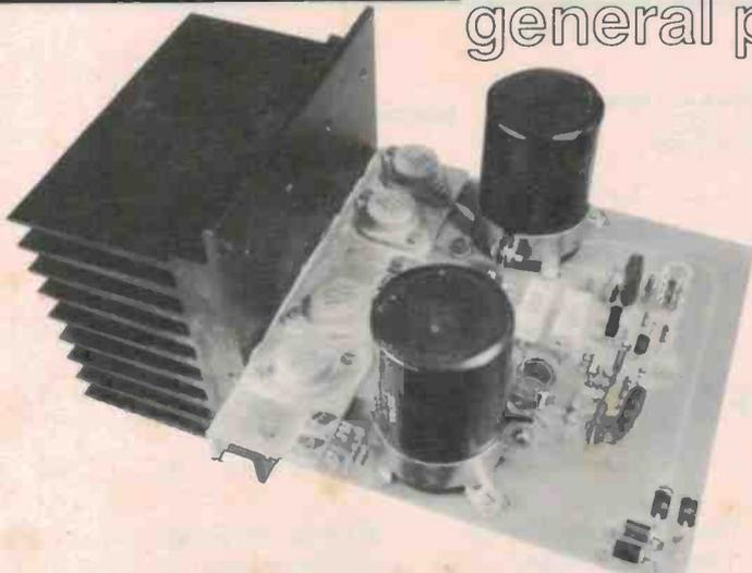
temperature of the device is increased the collector-emitter current will increase if the base-emitter voltage is held constant. The increased current causes further heating and a further increase in current. This condition is called *thermal runaway* and results in the destruction of the output device.
