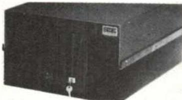
business and industry. 4MHz Z80 CPU, 64K dynamic memory with bank select to allow multi-tasking multi-user through 8 pages of 64K each, and up to 256K of RAM on a single board.
