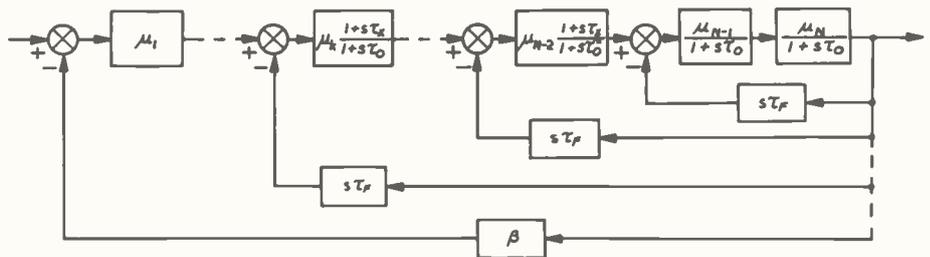
Figure 5. Block diagram of an NDFL amplifier.
