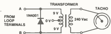
Beware of the high voltage pulses on the secondary of the transformer in this circuit.
