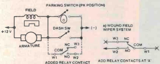
Figure 11. Wiper operation.
