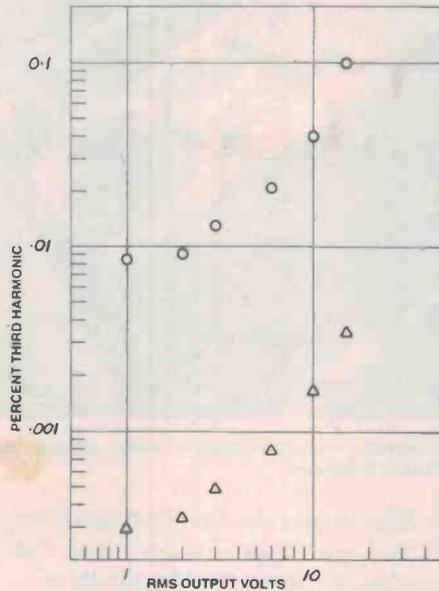
Figure 13. 1 kHz third harmonic distortion
