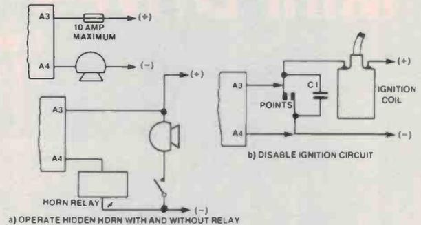
Figure 6. A3 and A4 alarm relay contact; giving extra protection.
