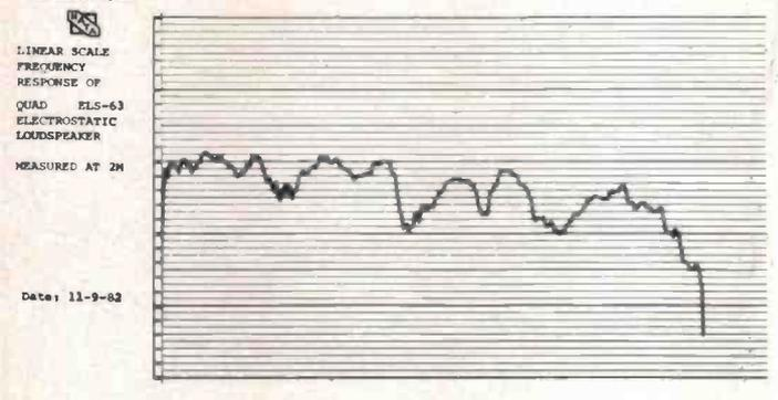
This was confirmed with the Swedish (Svenska) Hi-Fi Institute Test Record which revealed traces of mid-band colouration from the speakers which I had not previously detected in my A-B testing procedure. This was confirmed in part with white noise signals where the signal was not as 'neutral' as I would like.
