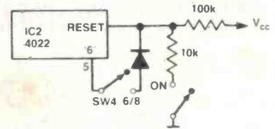
Only SW4, one diode and the 10k resistor are needed to modify the unit. Closing SW4 connects output '6' via the diode to the reset input. When the counter counts to '6' (i.e. on the seventh beat) a pulse is sent to the reset input, resetting the counter to zero, and the counter starts again. The 10k allows the ON switch to function without interfering with the reset action for 6/8.
