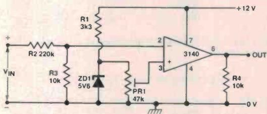
Figure 5. High value (0 — 130 V) under-voltage switch.
