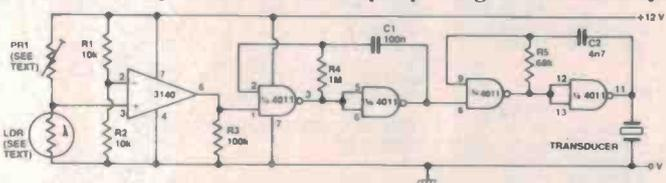
Figure 15. Dark-operated switch with low-power pulsed-tone output.
