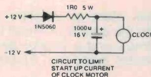
Figure 13. Clock circuit modification to prevent tripping of alarm.
