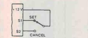
Figure 8. Wiring a hidden switch.
