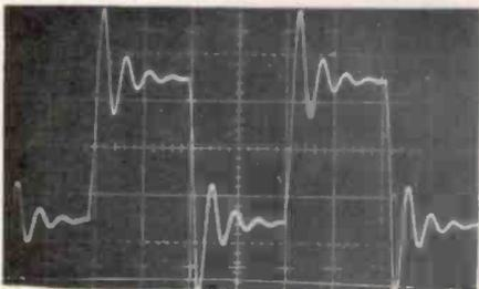
(b) 8 ohm and 2 uF parallel load
