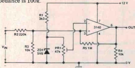
Figure 6. High value (0 — 130 V) regenerative over-voltage switch.
