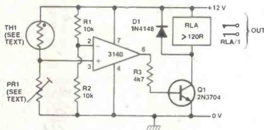
Figure 12. Precision over-temperature switch with transistor/relay output.
