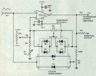
Figure 15. A triangle-to-sine waveshaping circuit employing a CA3140 op-amp and a CA3019 diode array. 128 - September 1983 ETI R1 = R2 = R 50 Hz, R = 3M3 10 Hz, R = 16k 1
