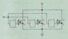
TO PREVENT SPURIOUS OSCILLATIONS, A 500 11 IN 12 RESISTOR OR FERRITE BEAD (FOR HIGHER SPEED) SHOULD BE CONNECTED IN SERIES WITH EACH GATE
