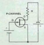
Figure 13. A p-channel device requires supplies of the opposite polarity to those used with n-channel devices.
