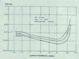
Figure 19. Distortion characteristics of the circuit in Figure 18.
