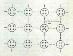
Fig 5c. N-type lattice structure.
