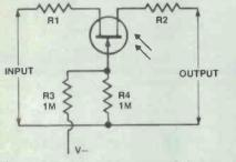
Figure 10. Example of a light-controlled attenuator (Teledyne Crystallonics).
