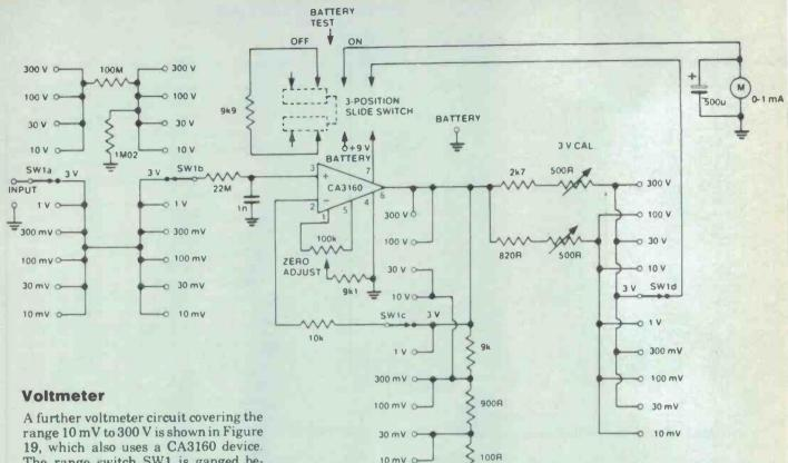
A further voltmeter circuit covering the range 10 mV to 300 V is shown in Figure 19, which also uses a CA3160 device. The range switch SW1 is ganged between the input and output circuitry to enable the proper output voltage for feedback to terminal 2 through the 10k resistor to be selected.
