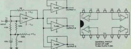
Figure 11. An audio 'distribution' amplifier for 'slaving' several pieces of equipment from a single source. Pinout for the quad op-amp is shown at right.
