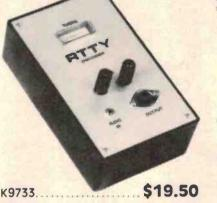
Display RTTY encoded messages on your Video Monitor. Receive up to date weather information, international News before the Papers, all sorts of coded military Info. Simple circuit uses PLL techniques  $\Rightarrow$  Single PCB Construction  $\Rightarrow$  Kit includes DB15 Piug and backshell for connection to microbee  $\Rightarrow$  Sheided pretinned PCB.
