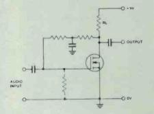
Figure 16. General circuit of a simple class-A audio amplifier using a power MOSFET.
