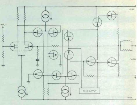
Fig. 16 Simplified Yamaha VFET amplifier diagram.
