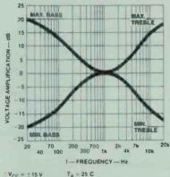
Figure 9. Response characteristics of the Figure 8 circuit.
