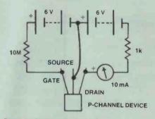
Figure 15. Testing a p-channel device.
