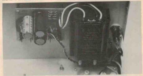
Rear panel assembly. View of the rear panel showing placement of the various pieces of the power supply. I used a different transformer from the 6672 specified as I had one on hand but no 6672. Note the rear edge of the ETI-1520 output amplifier module.
