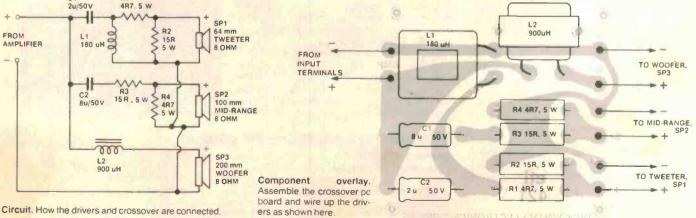
Circuit. How the drivers and crossover are connected.
