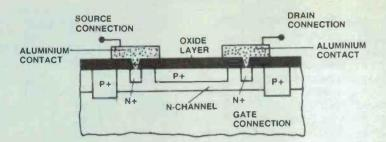
Figure 12. Structure of a silicon planar device (Mullard).
