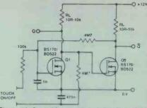
Figure 10. Capacitive touch switch will cycle on and off if finger is held on the sensor.
