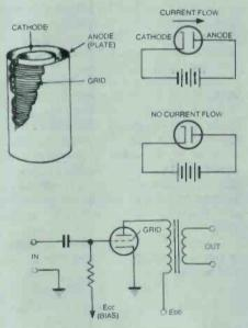
Fig 2. Triode construction, circuit and characteristics.
