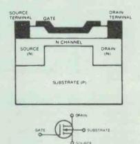
Fig 9a. N-channel depletion horizontal MOSFET construction and symbol.
