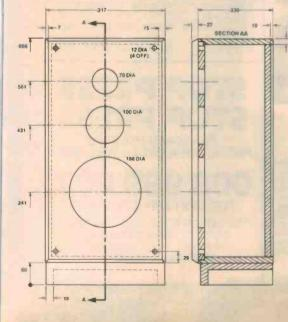
Cabinet details. All the cabinet dimensions are shown on the left and an exploded view of the assembly is shown at right. Dick Smith Electronics supplies precut panels with kits, which makes the assembly job a breeze. The front grille is an open weave black cloth stretched over a polycarbonate frame.
