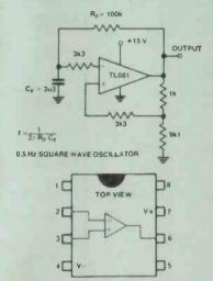
GENERAL PINOUT SINGLE OP-AMP TL060,TL071,TL070,TL071,TL080,TL081, CA3080.CA3140,CA3160. Figure 2. Half-Hertz oscillator using a TL081 plnout below.
