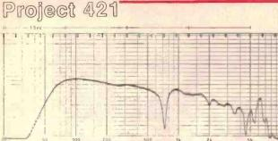
Woofer. The piston operating range extends over at least three octaves. The 'dip' near 700 Hz does not show up in the overall response. Vertical scale: 1 dB/increment.
