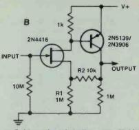
Figure 7. (a) a unity gain buffer stage with high input impedance and (b) similar stage, with gain (National Semiconductor).
