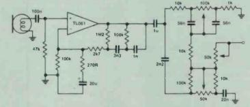
Figure 10. Moving-coll mlc preamp with tone controls, using an Internally compensated TL061 device (same pinout as TL071).
