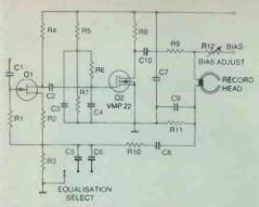
Fig. 13 Tape recording amplifier.
