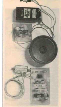
Set to go. The completed decoder and pitchpipe, before housing in Jiffy boxes.
