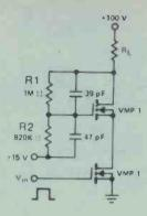
Fig. 8 Diagram for series operation (Siliconix).
