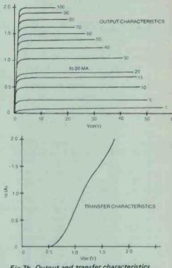
Fig 7b. Output and transfer characteristics of the 2N3054.
