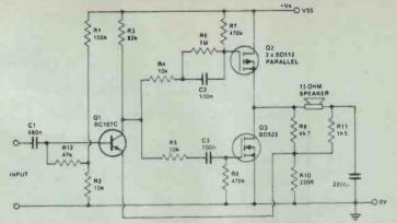
Figure 17. Class ABC amplifier circuit from ITT Semiconductors is simple but has 31/2% distortion at 1.75 W and is only suited to general applications.
