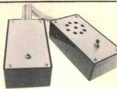
Housing. Two small jiffy boxes served admirably to house the decoder (left) and pitchplpe (right). The ribbon cable goes to the DB15 plug which plugs into the Microbee user port.
