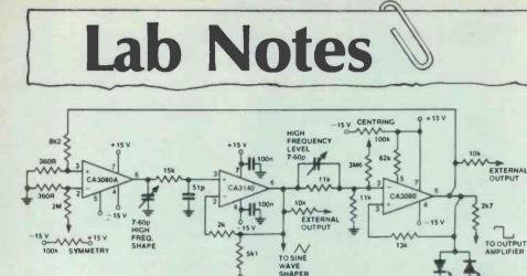
Figure 4. Function generator circuit. Sourcing or sinking current from pin 5 of the left hand CA3080 will vary the frequency.
