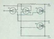
Fig. 3 Series output arrangement
