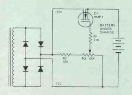
Fig. 18 Tapered current voltage limited battery charger.
