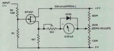
Figure 9. High input impedance voltmeter. Note that a BFW10 could substitute for the BFW61 (Mullard).
