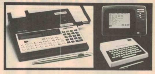
The PC-4 measures just 1 x 16.5 x 7 cm and has a typewriter-style keyboard of 53 keys for alphabetic input, plus a 10-key numeric data-entry keypad. A 12-character LCD scrolls horizontally to up to 62 characters, including lowercase.
