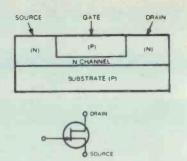
Fig 8. N-channel JFET construction and symbol.
