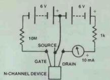
Figure 14. Testing an n-channel device.
