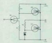
Fig. 4 Single ended output with current source.
