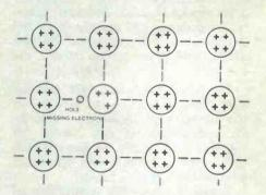
Fig 5b. P-type lattice structure.
