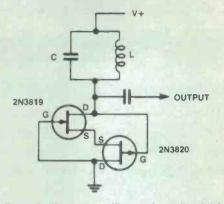
Figure 6. Sinewave oscillator using a 'Lambda' circuit.
