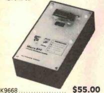
Versatile, low cost and easy to build. Plugs straight into the microbee I/O port. Suitable for 2716, 2732, 2532, 2732A and 2764 Eproms. Burn your games programmes and eliminate cassette
