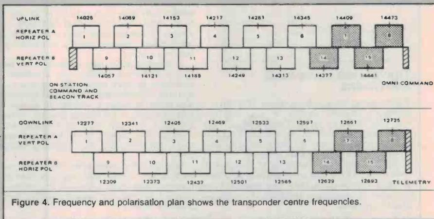
Figure 4. Frequency and polarisation plan shows the transponder centre frequencies.
