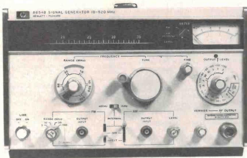
**Signal generator.** This run-of-the-mill signal generator, the Hewlett-Packard 6854B, provides all the fundamental features required of a modern unit. It covers 10-520 MHz and +13 dBm to -130 dBm and can be either internally or externally AM or FM modulated.
