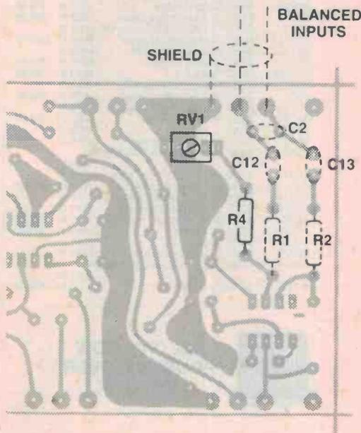
CMRR trimmer. Alternative overlay showing the positions of RV1 and R4. With a normal vertically mounted miniature trimpot, the screwdriver adjustment slot should face away from the rotary post (towards rear of board). ▶
