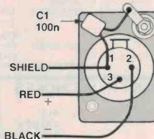
Input wiring. Suggested input wiring. Pin 1 of the Cannon socket goes to the board common track, which should not be connected to the chassis. C1 ties the chassis to the common for ac signals, avoiding 'earth loops' via chassis connections.
