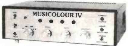
Combination Colour Organ and Light Chaser. Four channel colour organ. Internal micro-phone or connect to speakers for colour organ operation. (The lights connected to each channel pulse in beat to the music proportional to portion of frequency spectrum concerned.) Four chaser modes forward and reverse. Output lamp load capacity a massive 2400 watts — that's 100 party globes. Full instructions and every last nut and bolt included. Great for parties, shop signs, display windows etc.
