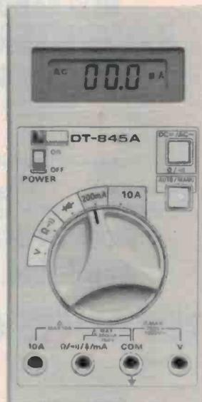
the volts and resistance functions. The 14 mm high display shows the mode of operation, range and polarity of the measurement, along with the value.
