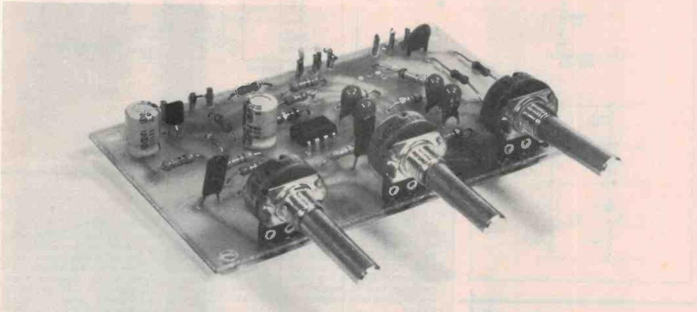
THE LAST balanced input preamp described in ETI was the ETI-461, published in December 1982. The '461 is a full instrumentation amplifier and has very good specifications suitable for virtually all balanced transducers. For most microphone work however, the simpler differential amplifier is generally adequate and is what I've chosen to use in this project. The ETI-461 article is recommended reading to clarify the pros and cons of each approach.
