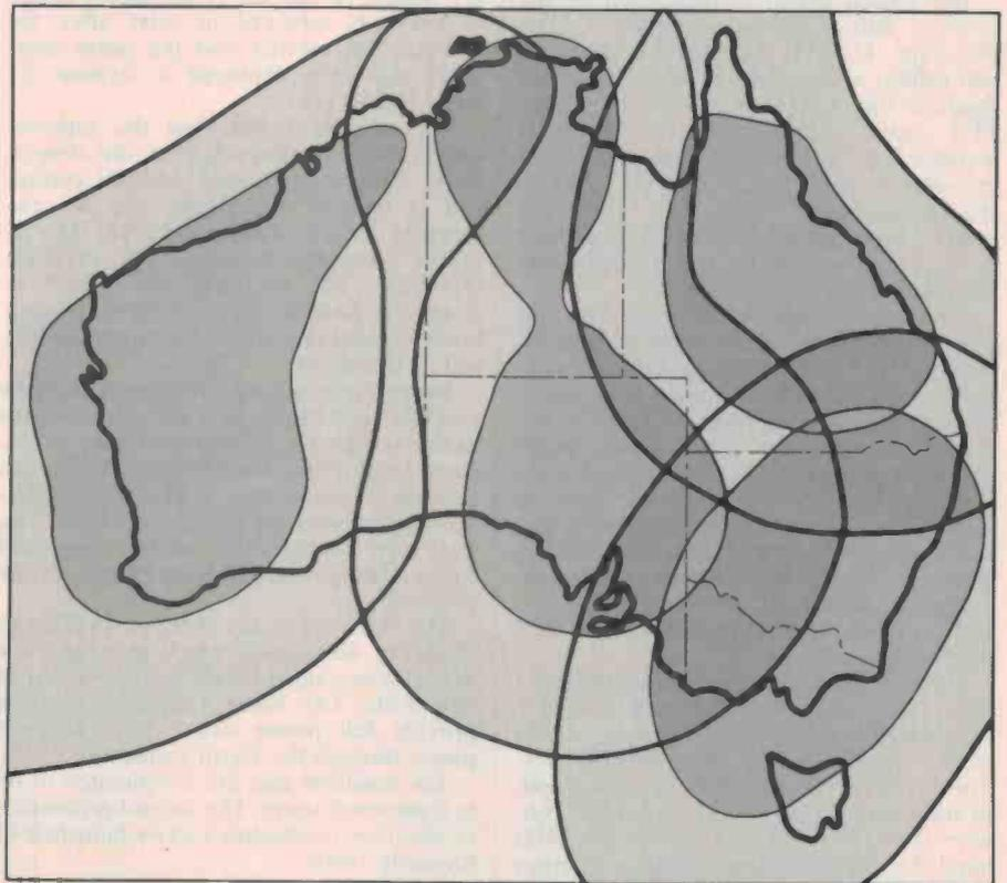
Map 2. Typical EIRP performance (dBW) for the 30 W channels in each spot beam at 160°E. The shaded area shows the 47 dBW primary coverage and the 42 dBW secondary coverage is shown covering the larger area.
