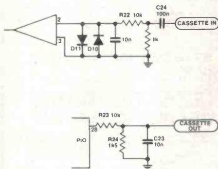
With this modification your optimum record/playback level will need to be re-established. For most low cost cassette machines, a setting between a third and a half of maximum has been found satisfactory.
