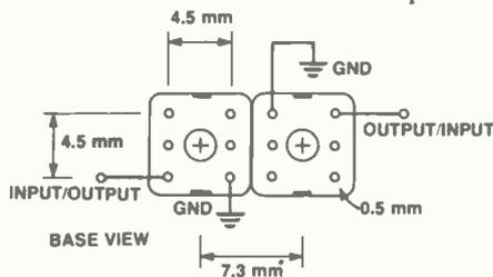
Filter pinout. Pin connections and layout of the Toko helical filter set.
