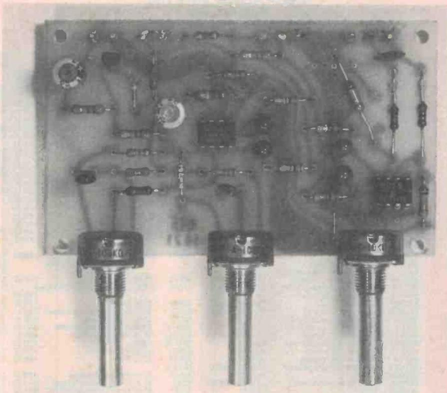
the screwdriver side towards the rear where it is accessible. The electrolytic capacitors are polarised and their orientation should be checked before soldering, as should the semiconductors. The two 8-pin IC sites on
