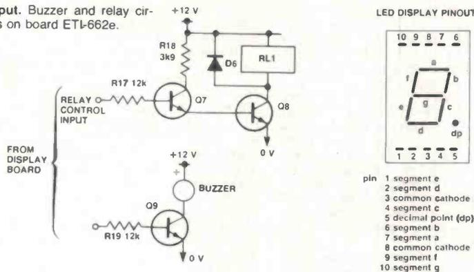
LED DISPLAY PINOUT
