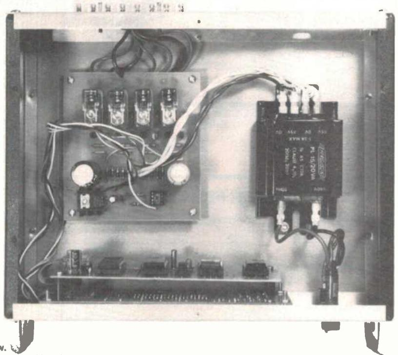
**Inside view.** Showing the general location of the output board and power supply, prior to installing the mains wiring.
