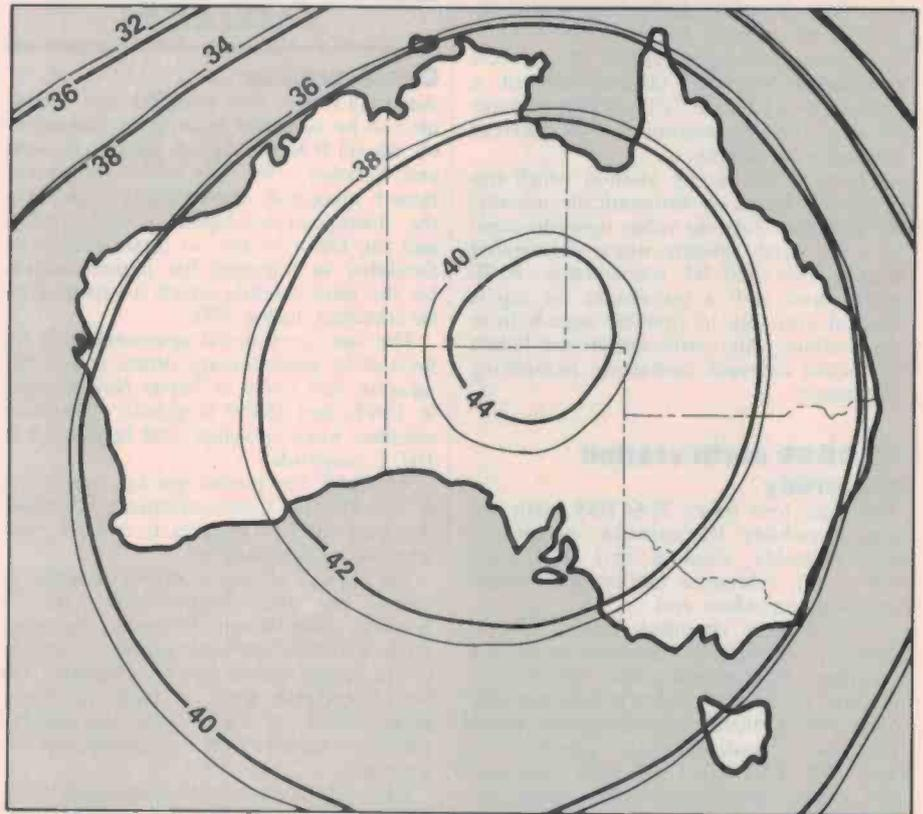
Map 1. The national A beam EIRP (dBW) from 160°E longitude showing the 30 W (thick line) coverage and the 12 W (thin line) coverage.
