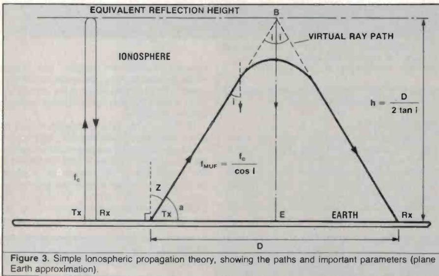
Figure 3. Simple ionospheric propagation theory, showing the paths and important parameters (plane Earth approximation).
