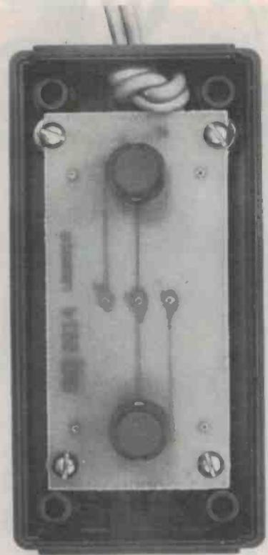
**Remote.** The remote unit is housed in a small OKI plastic case. I wired the cable to the copper side of the board, for the sake of convenience. The cable should be knotted where it passes through the case to obviate any strain on the soldered connections. Use the bare pc board as a template to mark drilling holes for the two pushbuttons.
