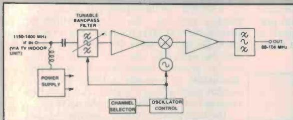
Figure 3. HACBSS single channel per carrier block translator.
