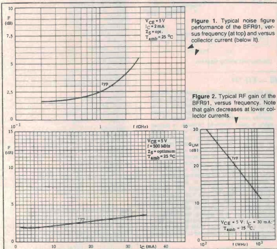
around 18 dB at 500 MHz (but this varies with bias and frequency — see Figure 2). In addition, the BFR91 has good dynamic range, achieving excellent intermodulation distortion figures. This is important, as, with this preamp being the first stage in a receiver, any distortion products produced by strong off-channel signals will be amplified by the rest of the receiver, causing interference.
