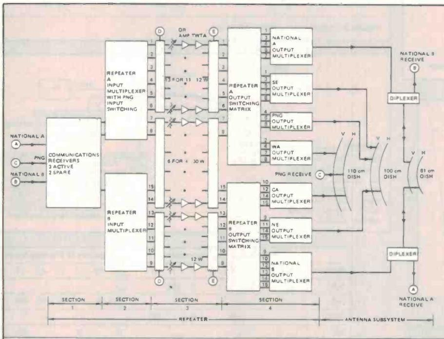
Figure 5. Block diagram of the AUSSAT communications payload.
