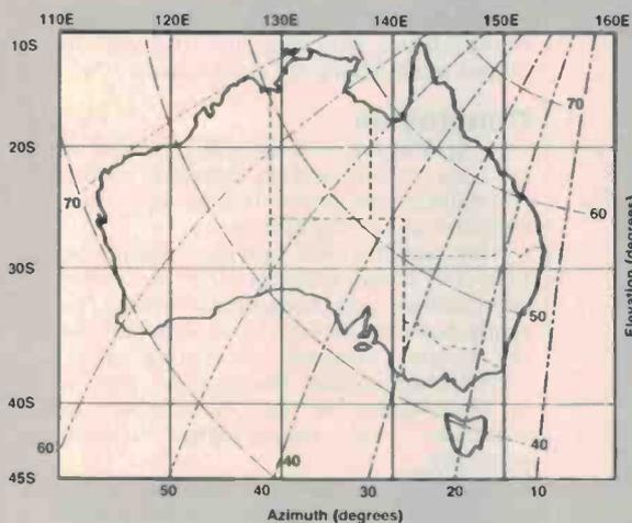
Looking at the AUSSAT spacecraft. Azimuth and elevation angles from an earth station to a satellite at 160°E. The angles for the other locations will not differ from these by more than 100.
