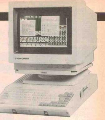
the Mitac because it comes with an electroluminescent screen as standard, but is still restricted to 240 V supply. It features an 8088 from Intel with 256K of RAM as standard, expandable directly to 512K. A single 5<sup>1</sup>/<sub>4</sub>" disk is also available as standard, with space for a second.
