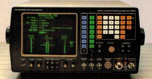
THE INCREDIBLE NEW 2955 MOBILE RADIO TEST SET FROM MARCONI
