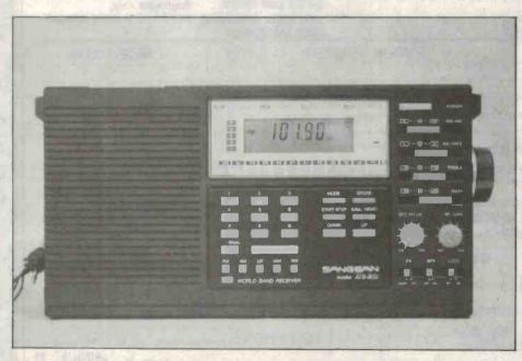
continuous coverage. The inclusion of the 150-281 kHz band is presumably for the European market as the majority of its AM broadcast stations operate in this part of the spectrum. What do you get? Well, the frequency
