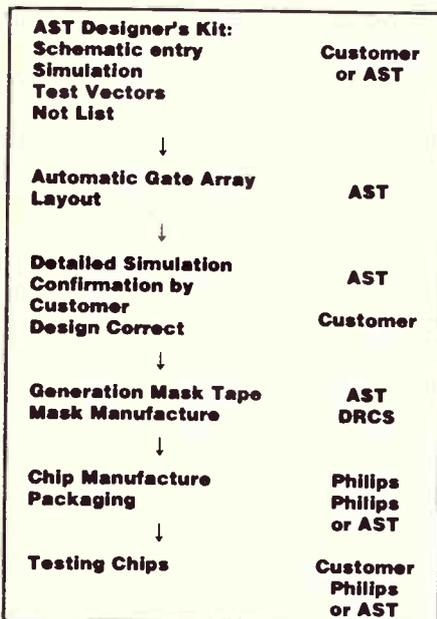
Figure 1. Steps in the production of an AST gate array.
