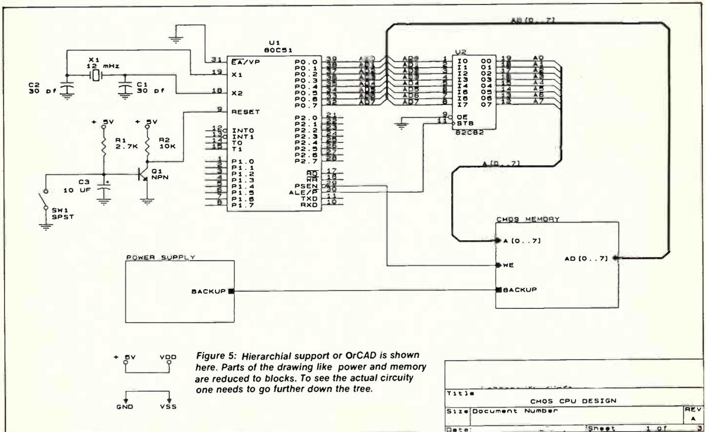
Figure 5: Hierarchical support or OrCAD is shown here. Parts of the drawing like power and memory are reduced to blocks. To see the actual circuitry one needs to go further down the tree.
