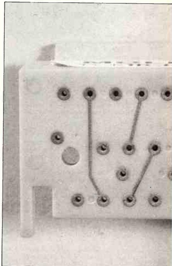
tive plating methods used for FR-4 boards can be used for thermoplastic moulded boards provided they are flat 2-D configurations. The injection moulding materials are all able to give the required 8 to 10 lbs/inch adhesion requirements for conventional boards.
