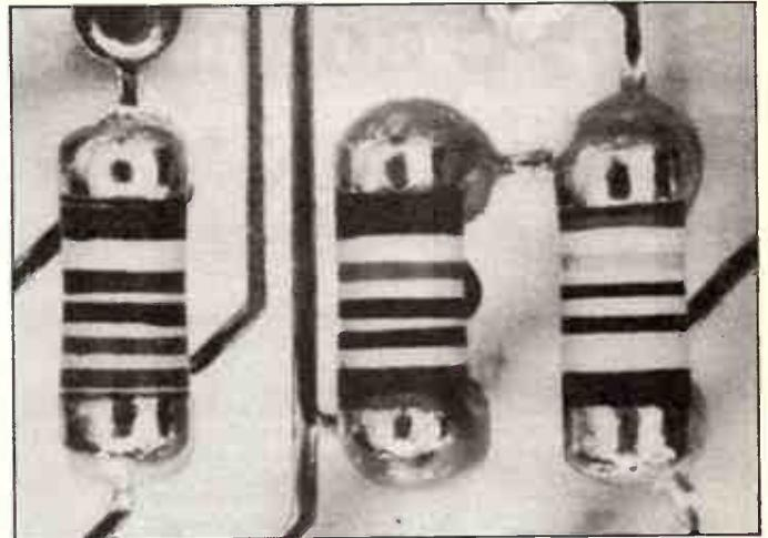
Figure 8. Example of various printed circuit patterns for MINI-MELF resistors.
