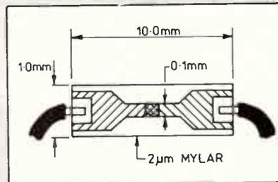
Fig 3. Thin Film Thermocouple for Propellant Studies.
