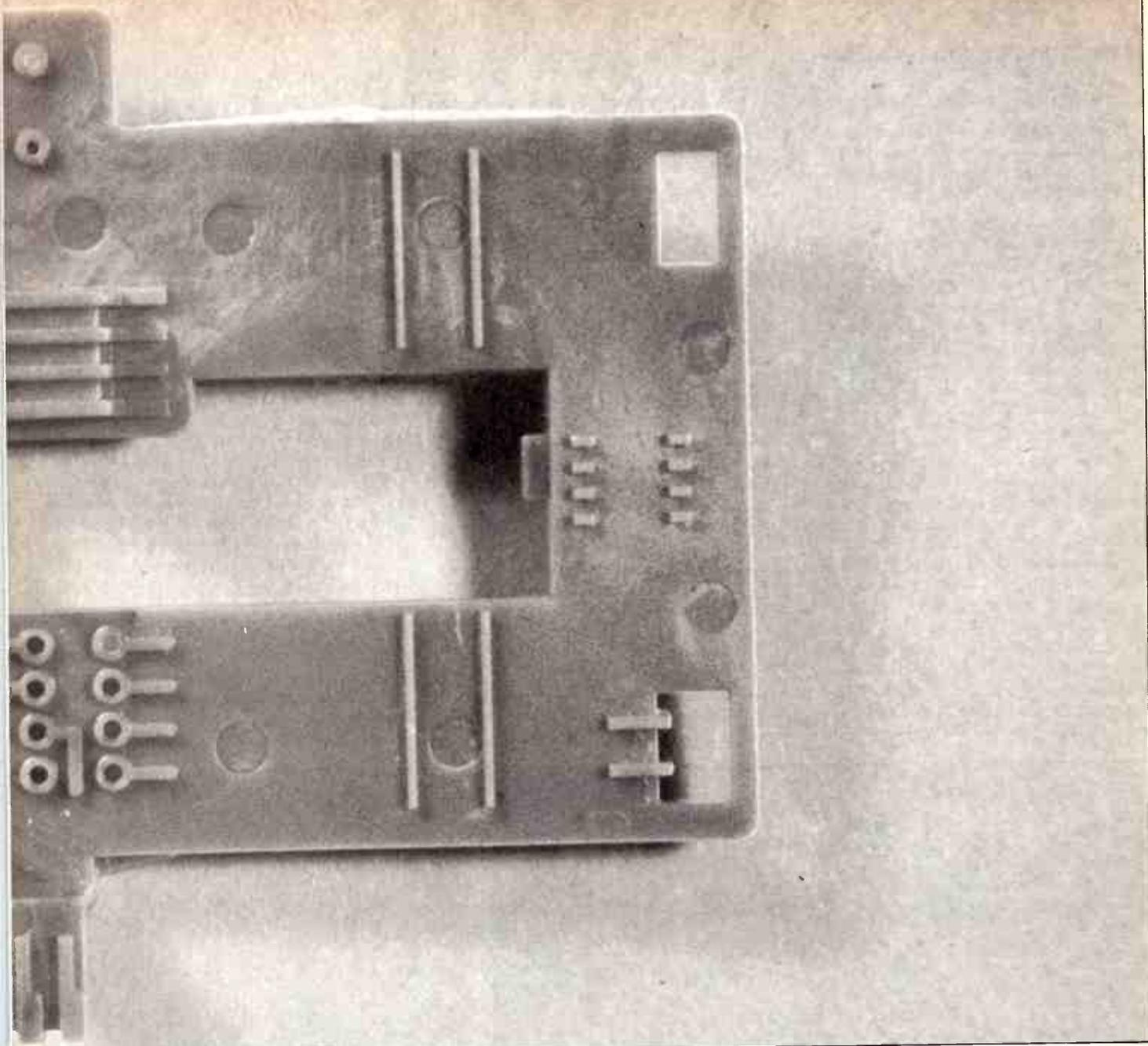
*Moulded board substrate showing detailed standups, tracks of insulation and strengthening ribs.*
