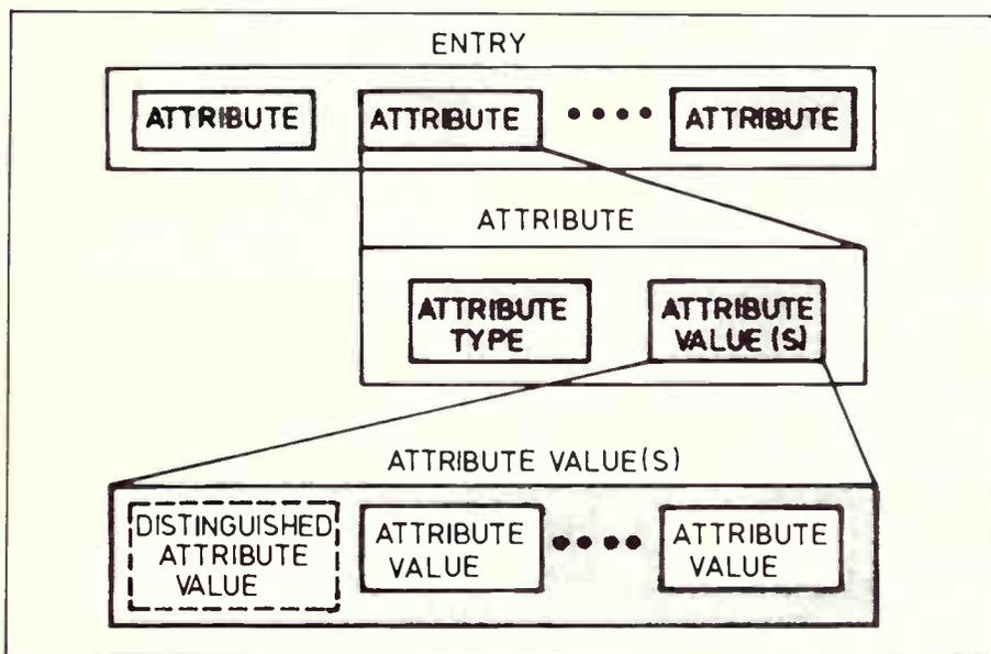
Figure 1: The structure of an entry in the proposed electronic directory.
