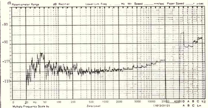
Signal to noise ratio with a one third octave band noise generator. At top reference to a 5mV input. At bottom, a 500 mV input.
