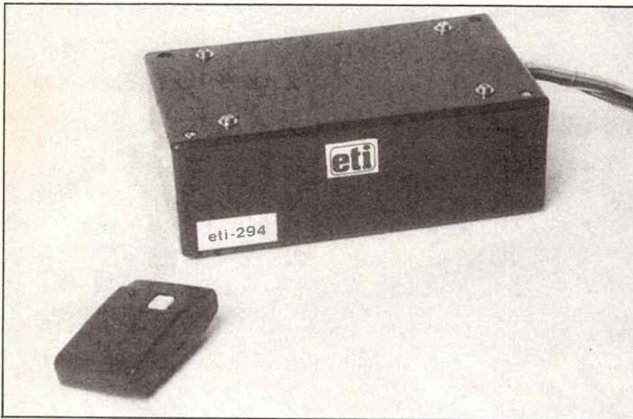
THE MORE EXPENSIVE commercial alarms includes some type of relatively insensitive 'shock detector'. The unit described here goes one better! It features "two level shock detection". Its more sensitive level can be triggered by gently knocking the vehicle and only produces a short alarm period whilst its less sensitive level can be triggered by a hard knock to produce the full alarm period.
