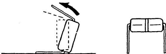
Figure 1. You may need to straighten the IC's pins. To do so, work on a metal surface, such as a small sheet of aluminium. Pick up the IC using your thumb and forefinger to grasp the ends; avoid touching the pins. Touch your other hand on the metal surface to equalise any static charge between you and the work surface, then lay the chip down on its side as shown here. Very carefully roll it towards the pins to bend the lower pins into line. Then turn it over and bend the other row of pins in the same manner.
