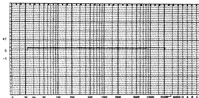
Measured frequency response with 10 dB pot (right channel) 20 Hz to 20 kHz.
