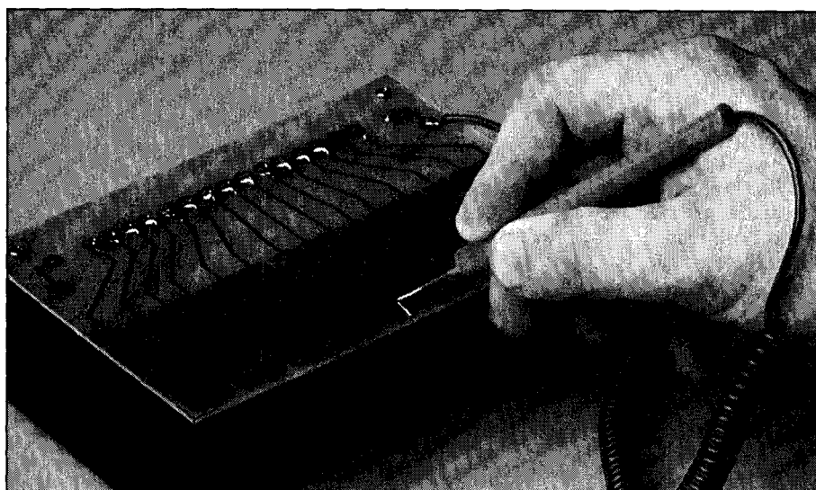
Figure 5. A stylus piano. This uses the 1202A printed circuit keyboard. The stylus connects to the module's positive rail to pull the note contact high. The spot adjacent to one lead of the piezo speaker indicates the 'active' lead. Rosc can be varied to vary the sound output characteristics.
