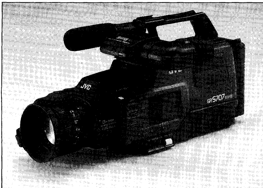
The GR5707 Camcorder displays the actual F stop selected by the user and also features time lapse and animation functions.
