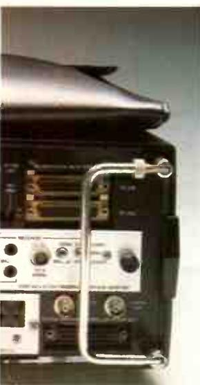
*Rear view of the Fireberd 6000 showing two plug-ins installed. The chromed handles fold out to provide protection for the rear panel.*
