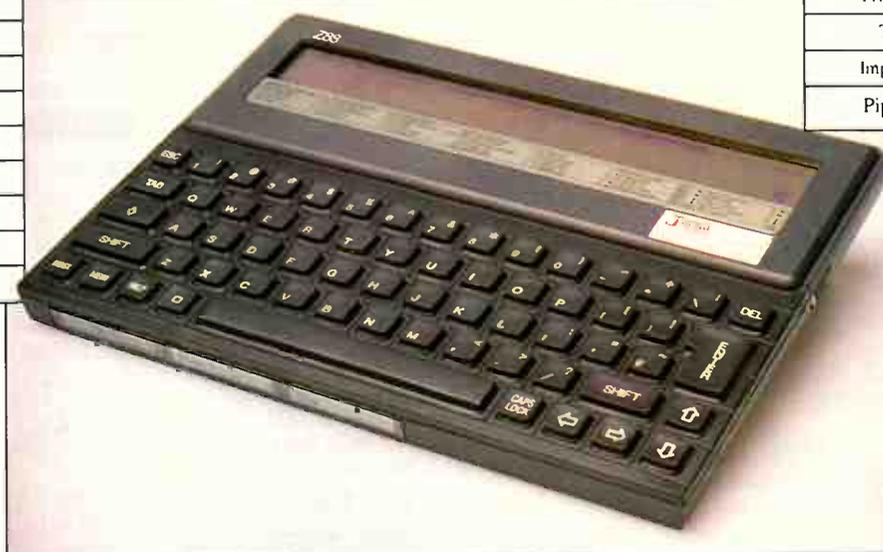
The Z88 has 32k RAM and 128k ROM built in, readily expandable up to 1.5 MbRAM. Its size is **2.5x21x30cm**, about the size of an A-4 pad. Our **LINK** software allows file transfers between the Z88 and most desktop computers. So the Z88 can be a truly **PORTABLE EXTENSION** of your desktop computer.
