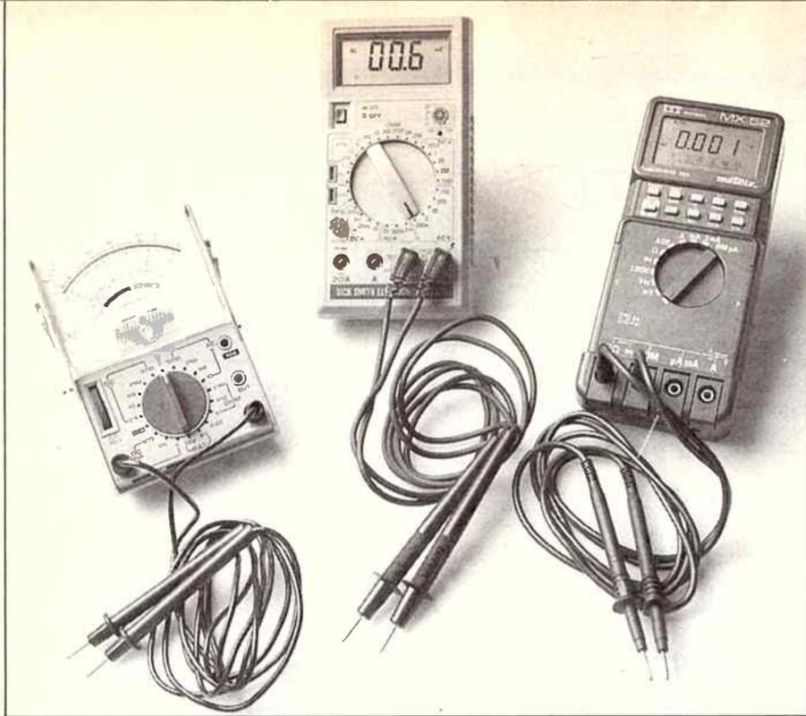
Typical multimeters in the \$40 to \$400 price range. At left is the Dick Smith analogue Q1022 meter (\$39.95), centre is the mid-priced Dick Smith 3.5-digit handheld DMM Q-1526 (\$179), and on the right is the high performance 5000-count Metrix MX52 from Elmeasco.
