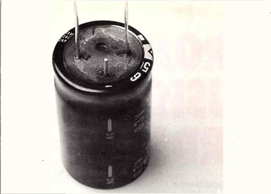
Most RB-type capacitors have a third lead, which is the very short lead you see in this photograph. This lead is used to properly locate or orientate the component, as well as provide some mechanical stability when soldered to the pc board.
