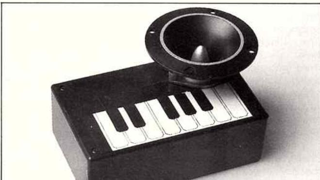
**'Portable piano' made using parts taken from a piano greeting card.**
