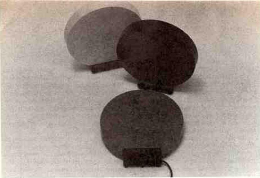
**The Terk 'pi' indoor FM antenna is about the size of a compact disc, but 28 mm thick. It is available in white, black and grey. It can be stood vertically or laid flat. It is an 'active' antenna, having a low noise amplifier as an integral part of the loop antenna inside. It is powered from a 12 Vdc plugpack.**
