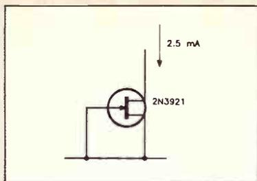
**Figure 9.14. Simple form of FET current source.**
