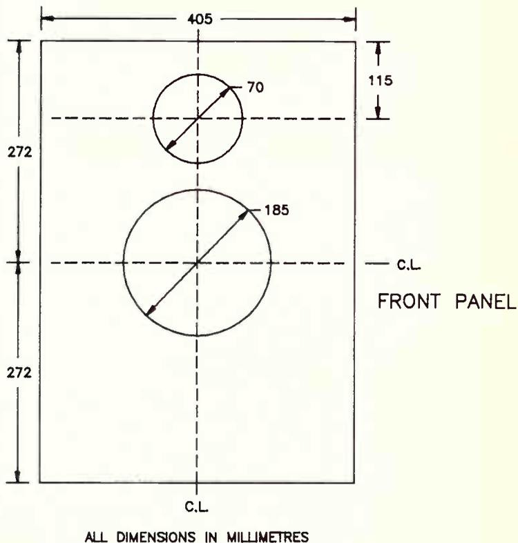
Figure 3. Showing the cutouts on the front and rear panels. The size of the rear panel hole will depend on the speaker terminal connector you get.
