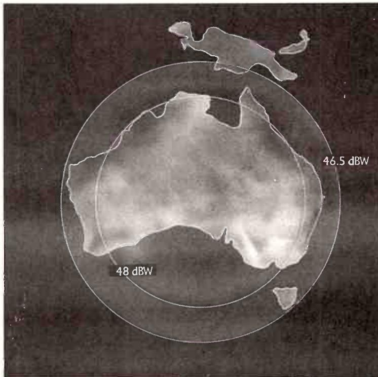
*L-Band coverage of Australia showing nominal signal strengths.*
