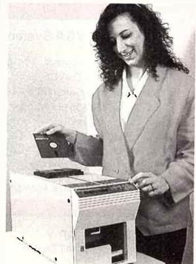
previously made copies and quickly formats blank diskettes. The internal 30Mb hard disk drive stores master images for both 3.5-inch and 5.25-inch applications.
