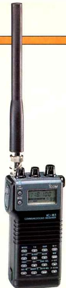
memory, band or range; dual frequency selection-keyboard or rotary tuning; 11 selectable tuning steps; 24 hour clock and timer with auto power on/off; LCD display with “S” meter; built-in NICad, or external DC supply (6 – 16V).
