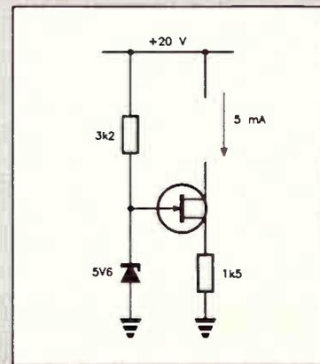
Figure 9.13. Current source using an FET.
