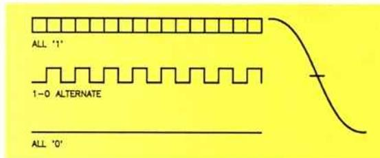
Figure 2. How the 1-bit continuous conversion process works.
