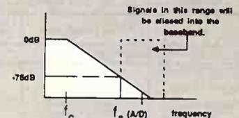
Since the filter loss is greater than 76 dB, any aliased signals will be below the 12 bit level.
