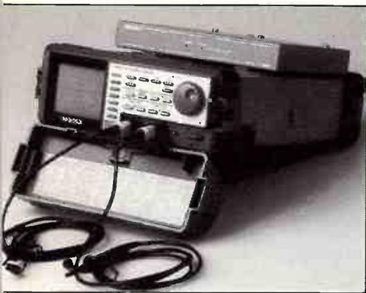
a digital-to-analog converter (DAC), the output of which then drives the vertical deflection amplifier for the cathode ray tube (CRT). The timebase controls not only the sweep, but the ADC, memory and DAC. The original signal is reconstructed point-by-point and displayed.
