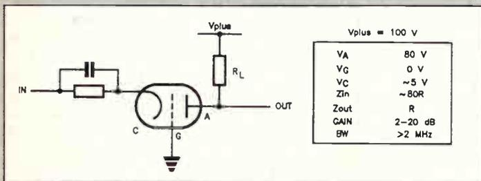
Figure 9.8. A grounded grid power amplifier.
