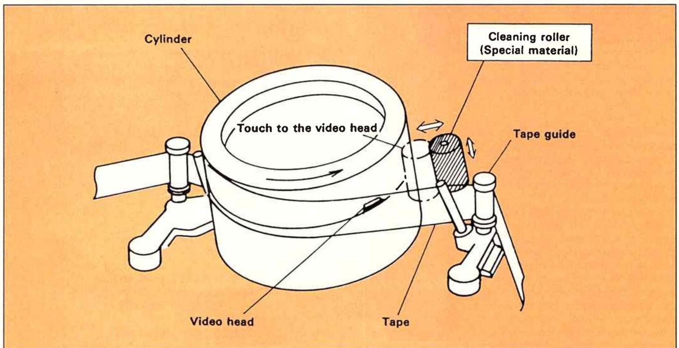
*The auto head cleaning system cleans the video heads automatically when recording or playback starts and finishes, to prevent dirt from accumulating on the heads.*
