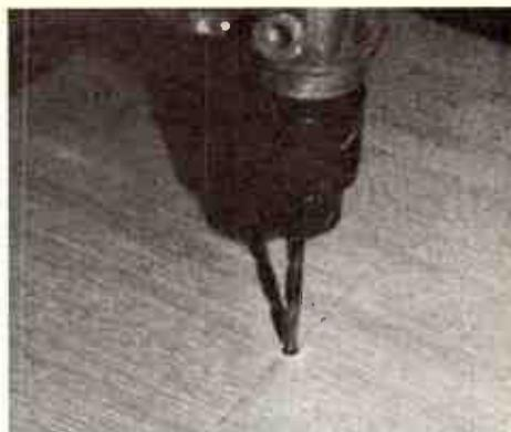
Drill pilot holes for centring the hole cutters when preparing the front and rear panels.
