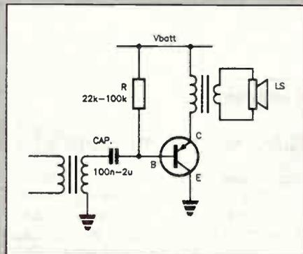
Figure 9.9. A typical single transistor power amplifier.
