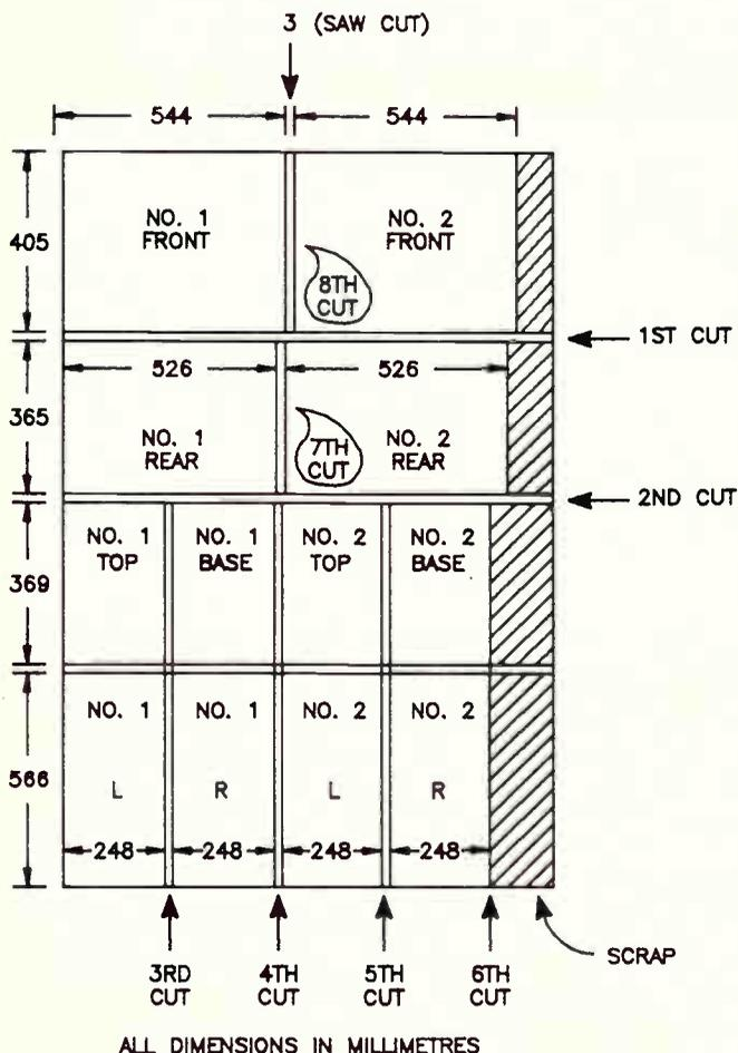
Figure 2. Cutting plan for the veneered particle board sheet.
