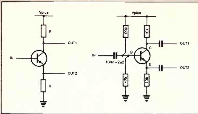
Figure 9.3 Single transistor dc and ac coupled phase splitters.
