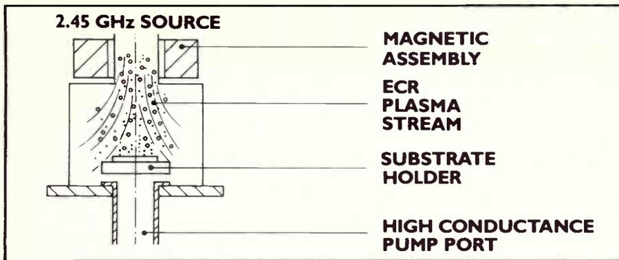
The ECR concept uses a microwave energy source in a strong magnetic field to ionise gas molecules by cyclotron resonance of the outer shell electrons.
