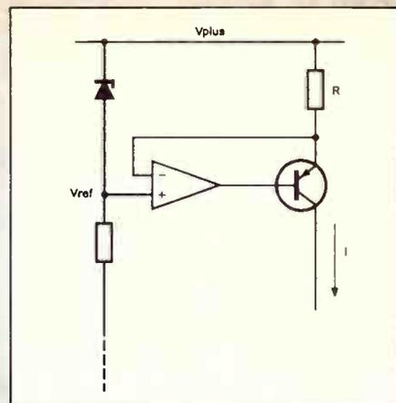
**Figure 9.16. IC-transistor constant current source.**
