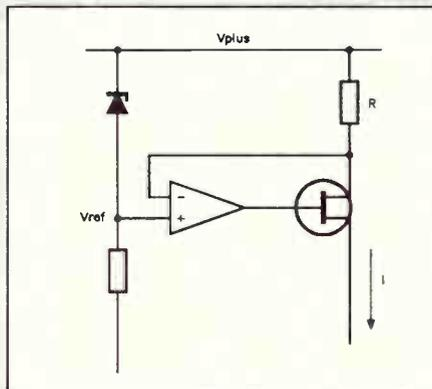
**Figure 9.17. IC-FET constant current source.**
