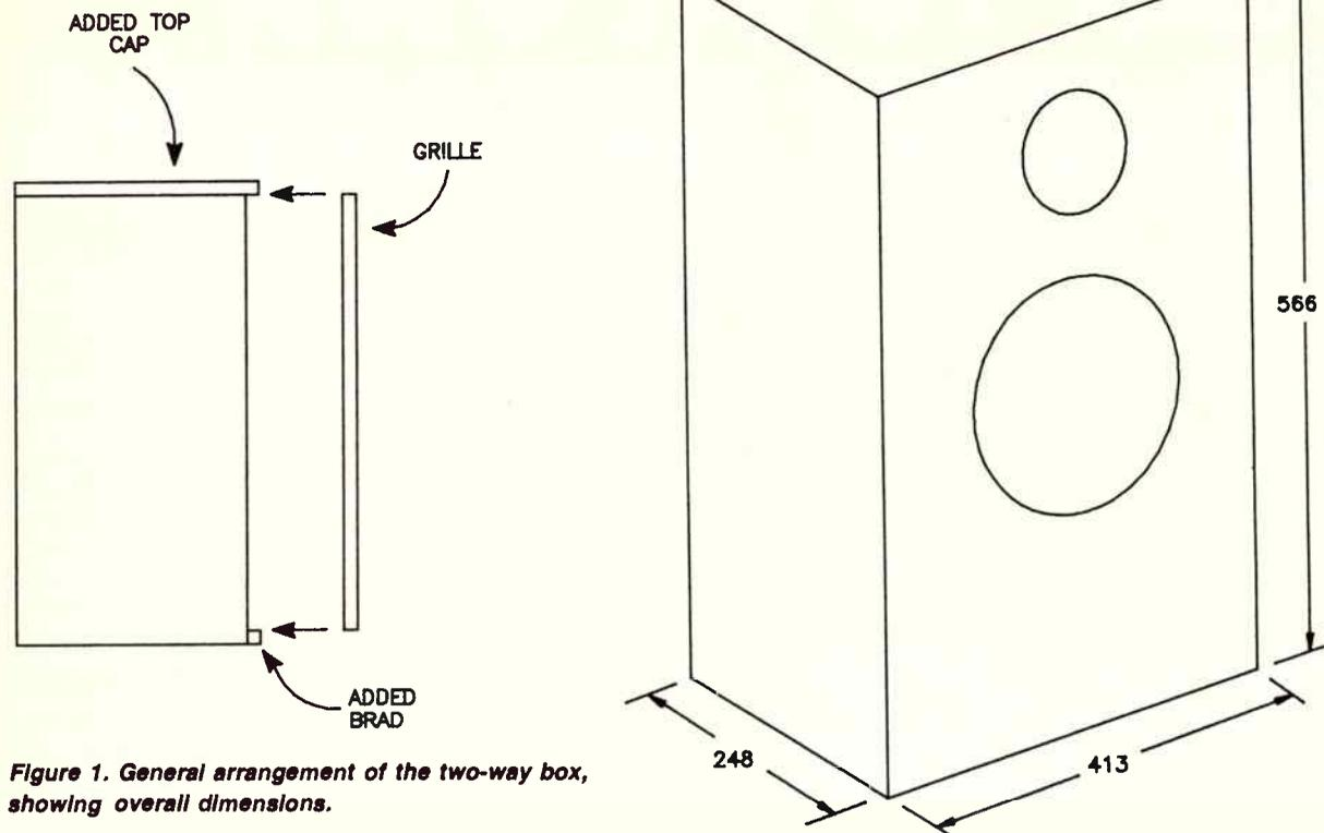
Figure 1. General arrangement of the two-way box, showing overall dimensions.
