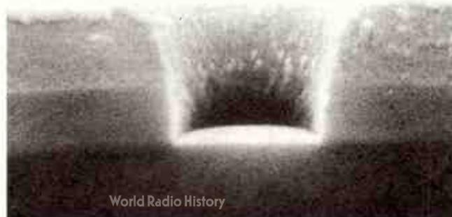
Features etched in silicon dioxide by ECR method. Processes previously requiring side wall polymerisation can now be done under polymer free conditions, thus eliminating particle and residue problems.
