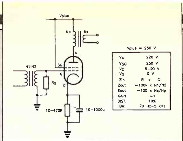
Figure 9.6. Single beam tetrode transformer coupled power amplifier.
