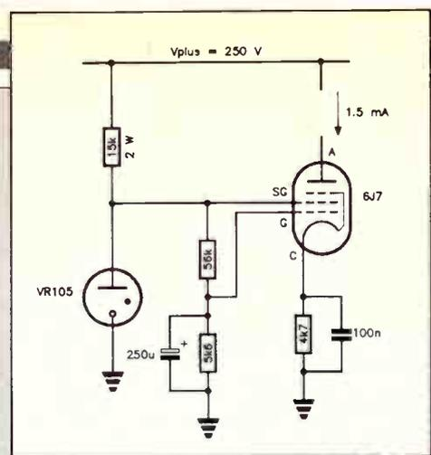
Figure 9.11. Valve current source, or constant current source.
