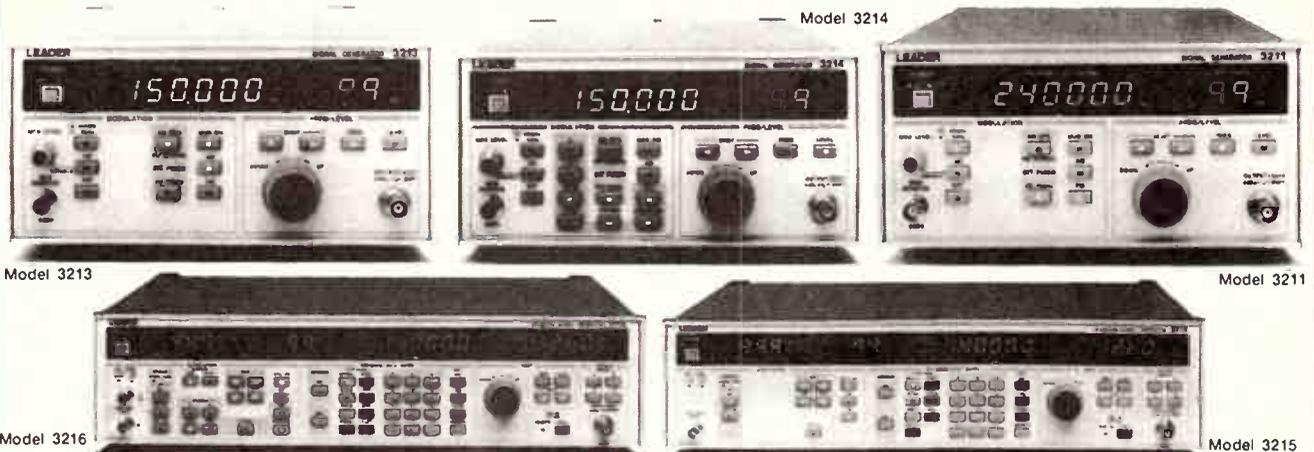
With outputs up to 140MHz (240MHz on 3211, 3213, 3214) these Leader generators use synthesizers for high stability and can be amplitude or frequency modulated (stereo on 3216)
