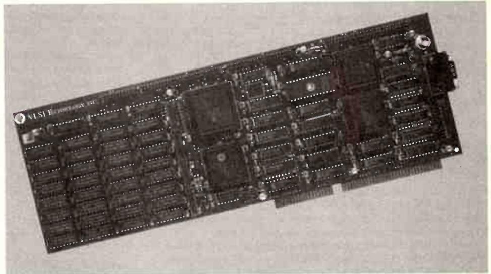
*The "Blue Streak" RISC computer card. It uses the low-cost VL86C010 from VLSI Technology, plus memory controller (MEMC) and I/O controller (IOC) devices with memory ranging from 1M up to 4M on-board. All you require is an IBM PC/AT or close compatible for a terminal. The card plugs in. Software support includes ANSI C, Fortran and assembler. A board-resident assembly debugger permits debugging of programs on the RISC itself with download capability on the target system.*
