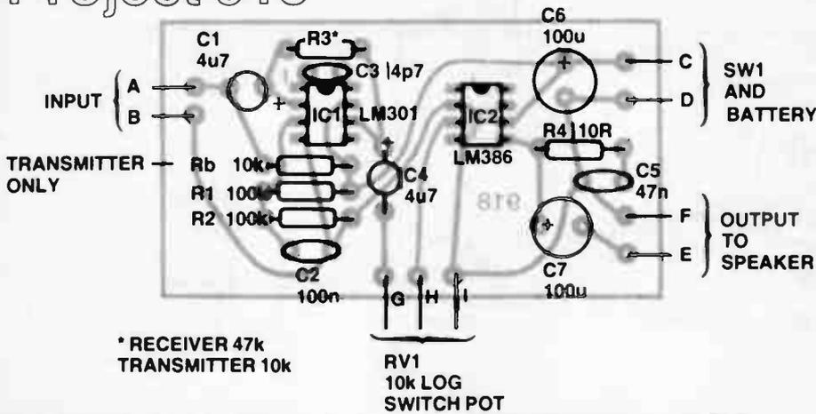
Component overlay for the amplifier. Note that Rb is not needed in the receiver amplifier and that the value of R3 differs between the transmitter and receiver.
