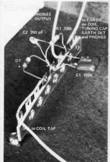
The components for our simple crystal set were mounted on an eight-lug tag strip screwed to the baseboard.
