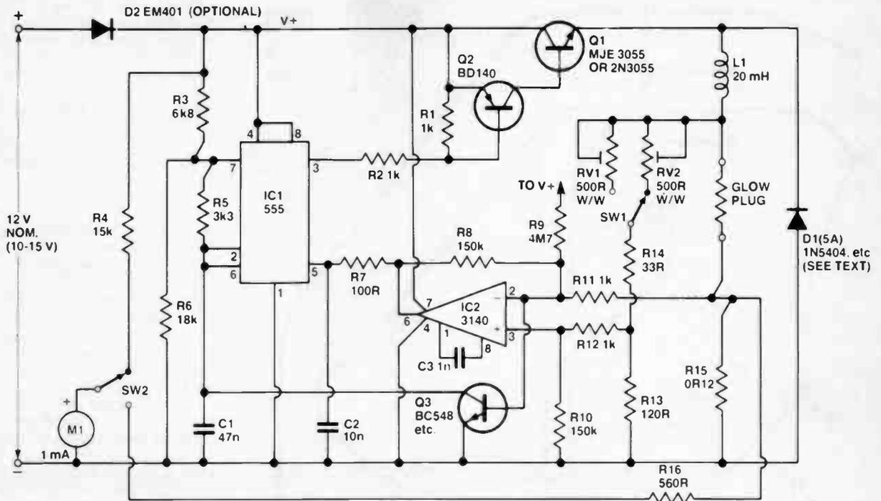
( $I_L$ ) flows, is sensed by Q3 which provides current-limiting.
