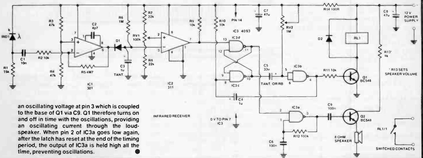
an oscillating voltage at pin 3 which is coupled to the base of Q1 via C9. Q1 therefore turns on and off in time with the oscillations, providing an oscillating current through the loudspeaker. When pin 2 of IC3a goes low again, after the latch has reset at the end of the timing period, the output of IC3a is held high all the time, preventing oscillations.
