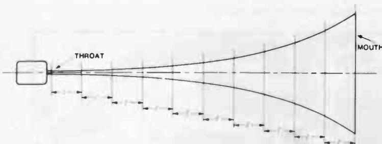
Figure 1. A straight horn has the width of the throat growing exponentially larger with increasing distance from the driver
