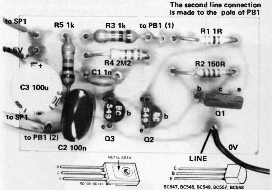
The second line connection is made to the pole of PB1
