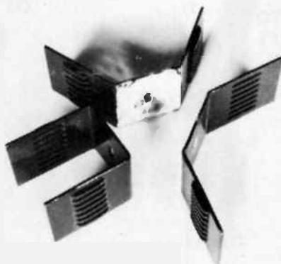
The heatsink we used for Q2 was made up from two 'flatpack' heatsinks, Dick Smith No. H3402, bent as illustrated and mounted back-to-back on the transistor. This ensures they fit in the case. Use plenty of silicone heatsink compound to get good thermal conduction. The unmodified heatsink is shown at lower left.
