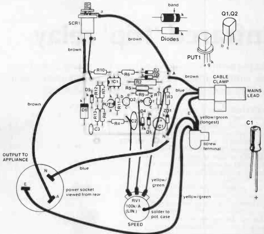
**Overlay and wiring diagram.** Follow this to assemble the pc board and wiring up of the external components. The pc board pattern is on page 90.
