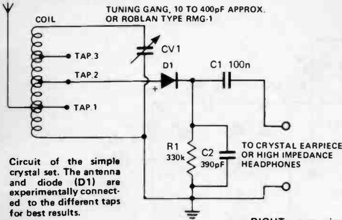
Circuit of the simple crystal set. The antenna and diode (D1) are experimentally connected to the different taps for best results.
