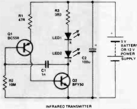
current through the LEDs is about one amp, but the average current is only about one milliamper.
