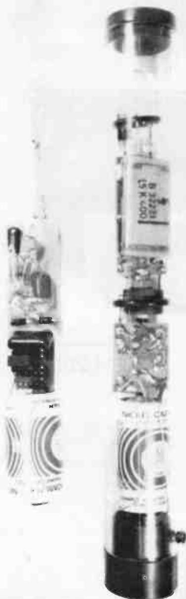
Two versions of the Flasher. On the left, one from a junked photo flashgun; on the right, from over-the-counter parts.
