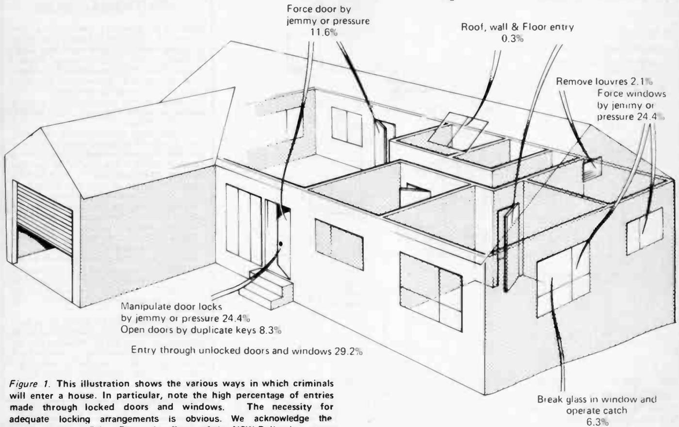
Figure 1. This illustration shows the various ways in which criminals will enter a house. In particular, note the high percentage of entries made through locked doors and windows. The necessity for adequate locking arrangements is obvious. We acknowledge the assistance of the Crime Prevention Dept. of the NSW Police in making these statistics available.
