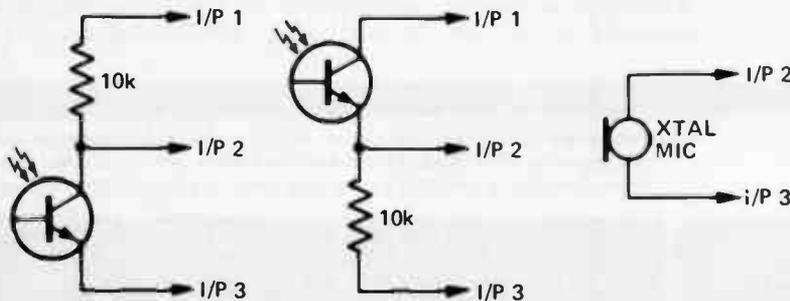
Use phototransistors, type FPT100 or TIL78 or similar
