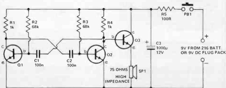
collector will be the opposite phase to that on the other collector (while one collector is up, or 'high', the other collector is down, or 'low').
