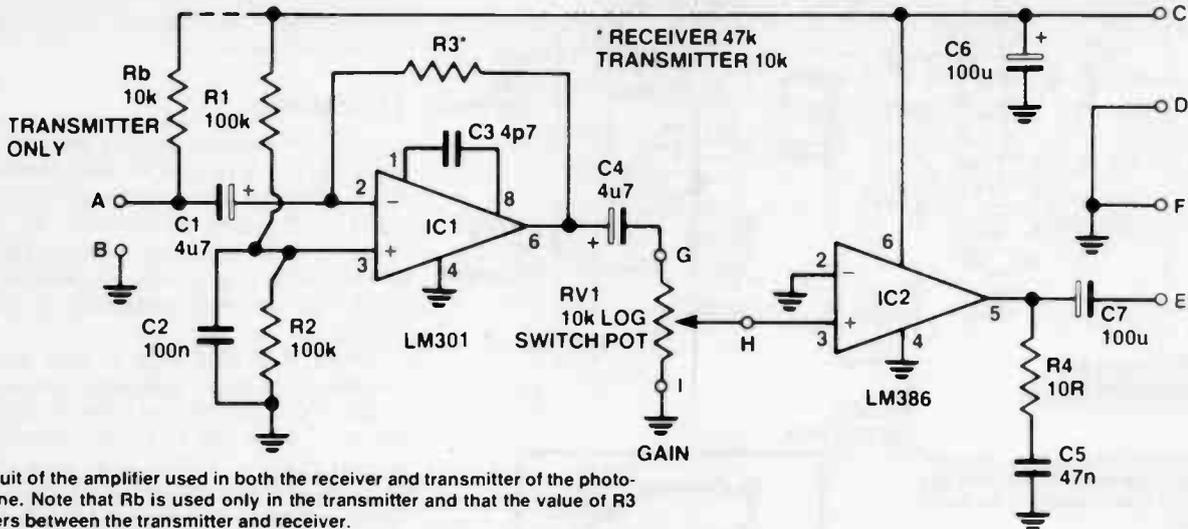
Circuit of the amplifier used in both the receiver and transmitter of the photophone. Note that Rb is used only in the transmitter and that the value of R3 differs between the transmitter and receiver.
