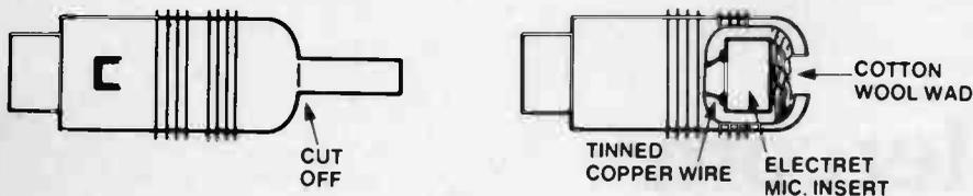
**Making the microphone.** A DIN plug is modified as shown to house the electret mic insert.
