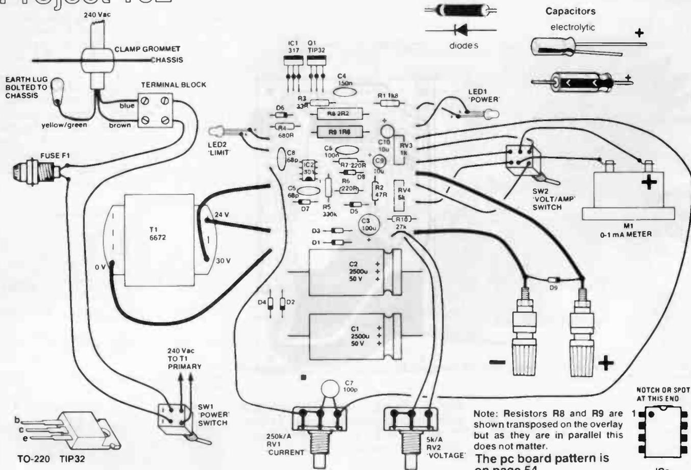
Note: Resistors R8 and R9 are shown transposed on the overlay but as they are in parallel this does not matter. The pc board pattern is on page 54.
