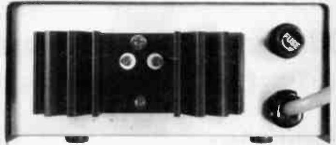
View of the rear panel showing heatsink and mains fuse placement.
