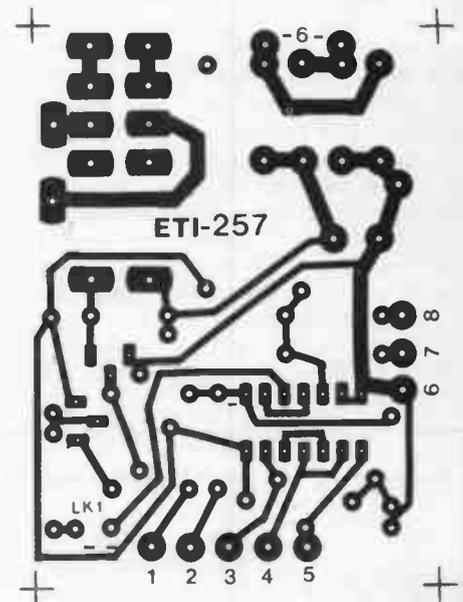
The relay driver board is simple, yet versatile. The external input/output pins are located around the edges of the board.
