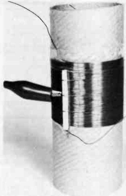
We wound the coil for these projects on a former cut from a cardboard mailing tube. The matchstick is slid under each of the turns to be tapped. Clean the enamel from the wire at each tap to get a good connection.
