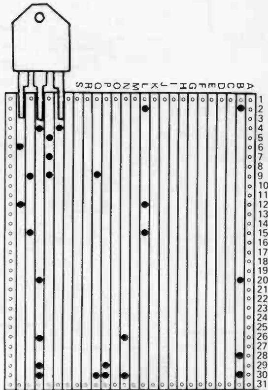
Veroboard solder connections — note no break holes are required in this board.
