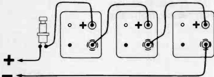
**Battery holder wiring.** If you use a dozen AA cells, as I did, this is how the battery holders are wired up to provide 18 volts.
