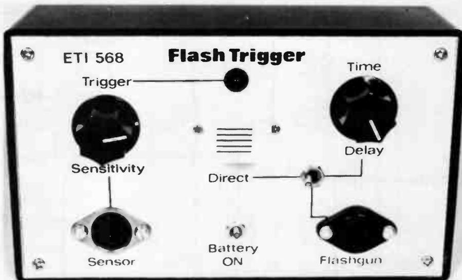
The prototype was housed in a 'jiffy' box measuring 160 mm long by 95 mm wide by 50 mm deep. The front panel was dressed up with a Scotchcal transfer.
