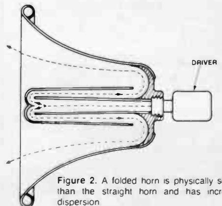
Figure 2. A folded horn is physically smaller than the straight horn and has increased dispersion
