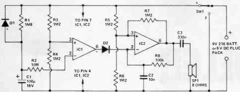
The second op-amp IC2 is used as a gated audio oscillator. Positive feedback, sometimes called hysteresis, is provided by R7 and negative feedback by the network R8 and C2. The positive input is again held at half the supply by R5 and R6.
