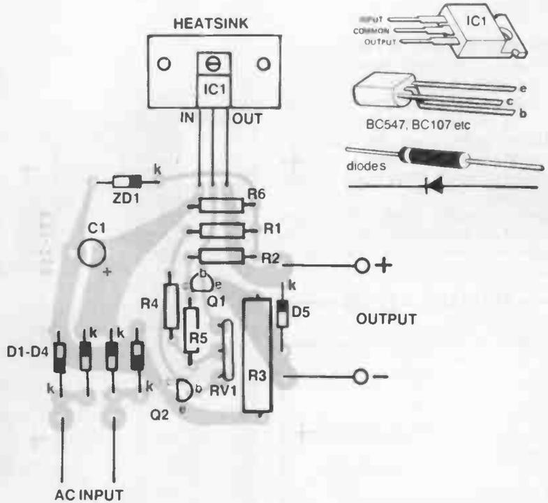
Construction is best tackled by mounting all the resistors, diodes and transistors on the pc board first — leaving R3 till last as it's a bulky item. Watch the orientation of the diodes and transistors as usual. Mount C1 next. Mount IC1 last of all and then attach a small heatsink to it.
