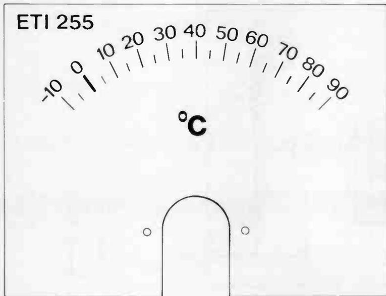
Full size artwork for meter scale covering -10 C to +90 C. Note that the limit for the LM3911 is +85 C.
