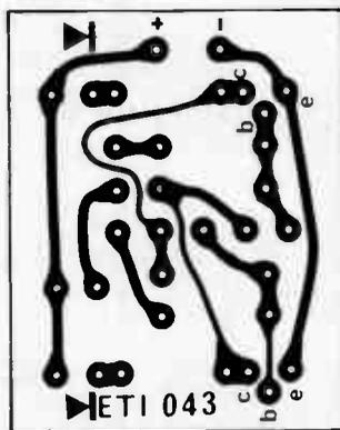
Fig. 4. Printed circuit board layout – full size 40 x 50 mm.
