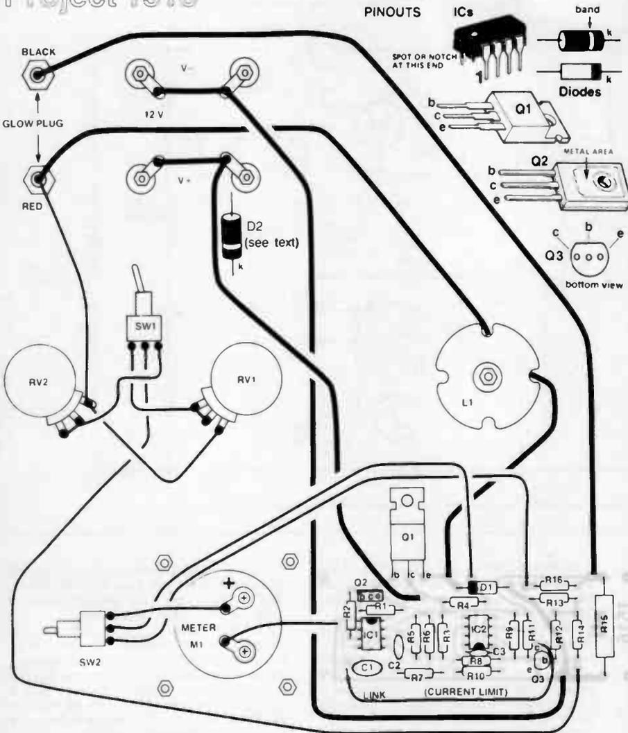
**Component overlay and wiring diagram.**
