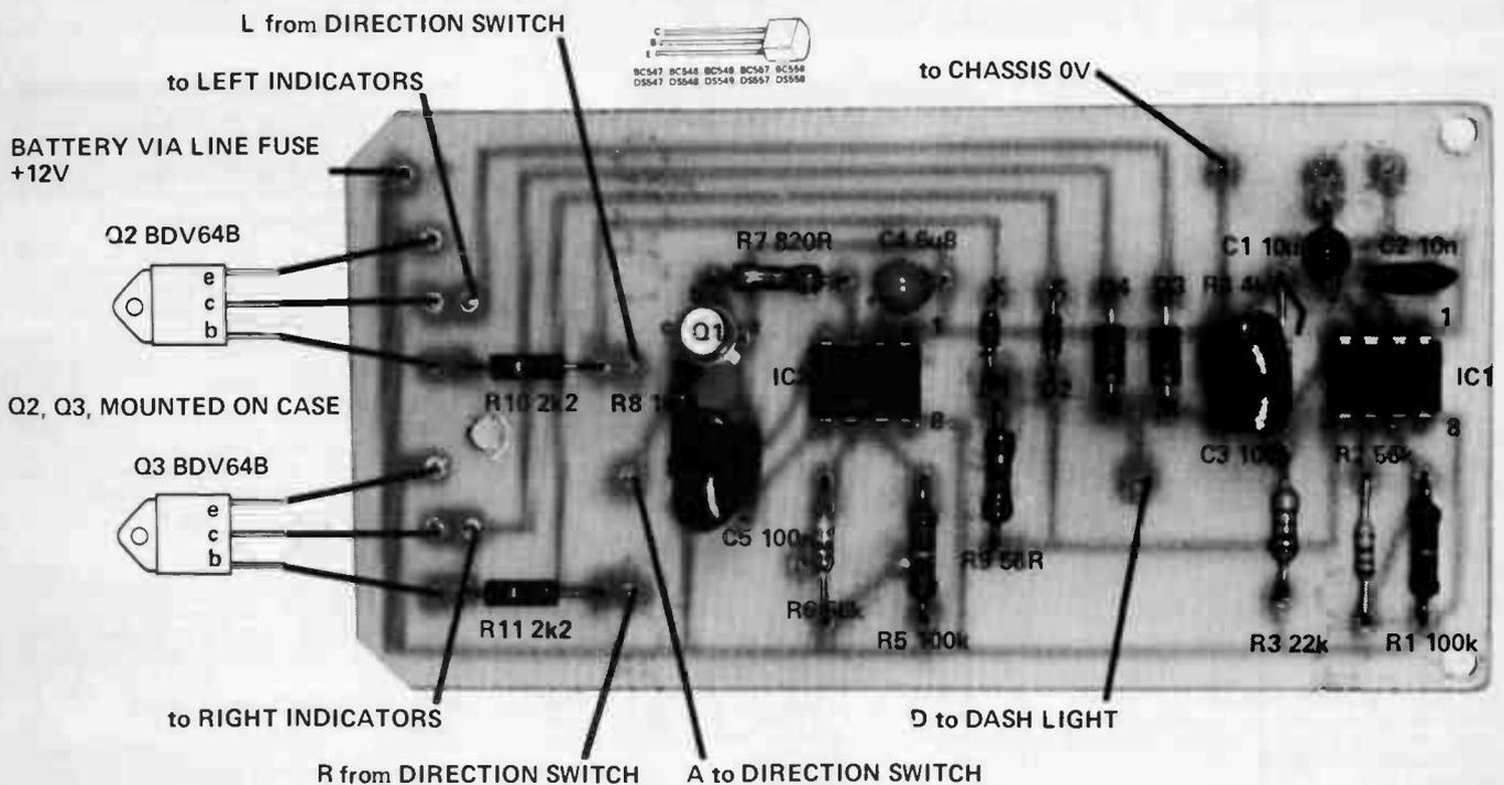
Component overlay and external component connections.
