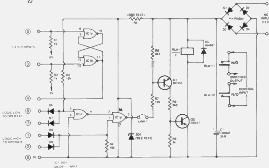
Circuit diagram of the relay driver board. Note that the rectifier diodes may be any of a range of types, such as 1N4001-2-4, etc. or EM401, EM402, etc. A variety of common relays will fit the pc board.
