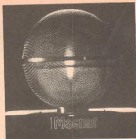
In the latest version of the ionophone tweeter loudspeaker, the ion cloud is formed at the tip of an electrode, as shown on the left. Modulation applied to the sustaining voltage produces sound waves in the range 4kHz and upwards. The sound source is enclosed in a metal mesh ball, as at right.
