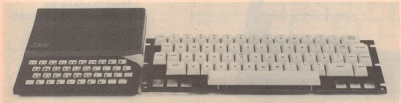
Now the ZX81 sports a new keyboard. Note that the keyboard is bigger than the entire computer, however!
