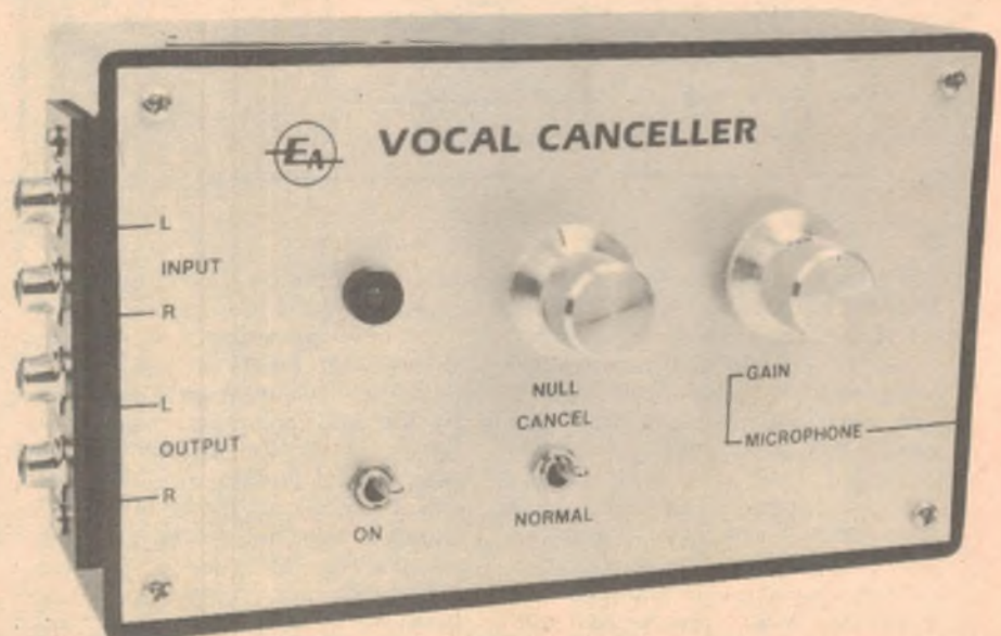
Vocal Canceller cancels the lead vocal and lets you substitute your own voice.
