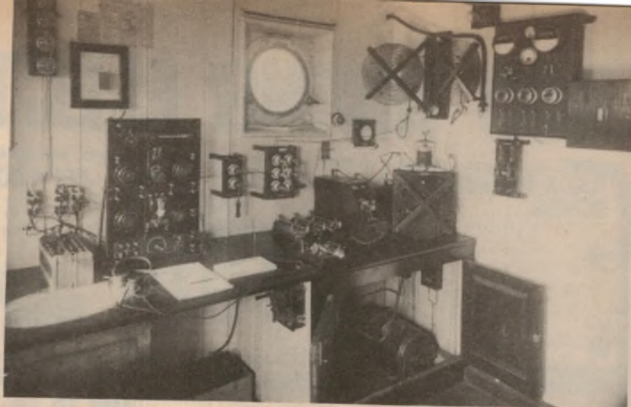
Spark transmitters were widely used in Australian merchant ships. Pictured above is the radio cabin of S.S. "Burwah", fitted with an AWA ½kW quenched spark set.
