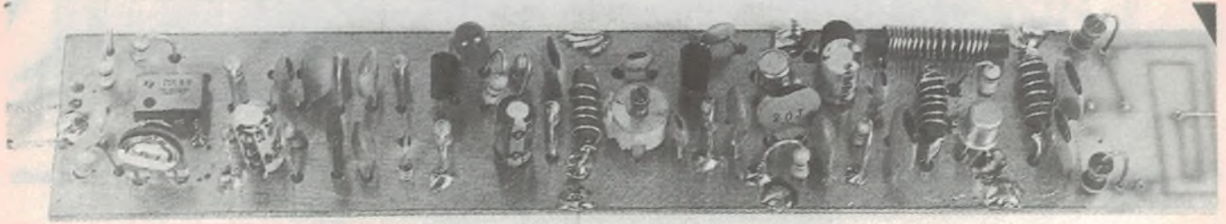
The prototype showing the component side of the PCB, with the shield removed. Capacitor C20 was mounted on the underside in this unit, but will mount next to L3 on the supplied PCB.
