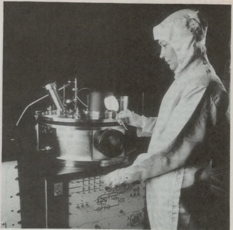
Placing a silicon wafer into the equipment which deposits a layer of PZT (lead-zirconate-titanate) onto the existing semiconductor underlayers.
