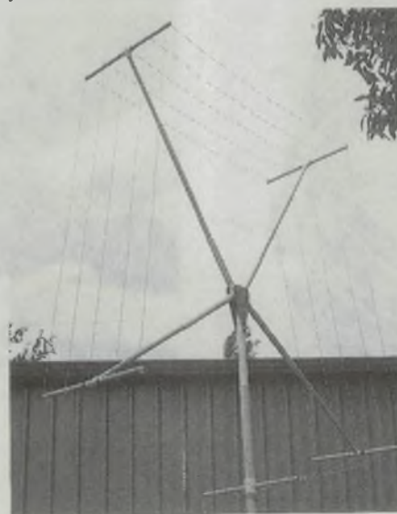
Fig.3: The author's pentagonal tuned loop, design to maximise L/R ratio.
