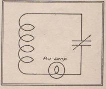
The schematic diagram of the wave meter.
