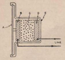
Fig. 15. Simple Carbon Type Microphone.
