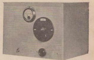
The front view of the oscillator, showing the main tuning control, power switch, and modulation switch.
