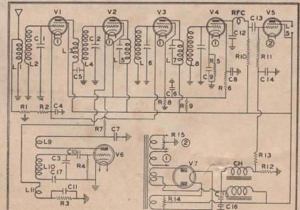
The schematic diagram of the Radiokes Simplified Super-Het.
