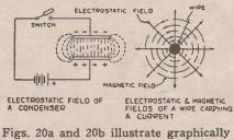
how radio waves are produced and radiated.
