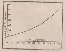
An idea of the calibration curve of the finished instrument is furnished by this illustration. minium box is available, it will suffice. Shielding, however, is not essential, because a high degree of accuracy is impossible with this type of meter. The dimensions are  $3\frac{1}{2}$  inches high, 4 inches wide by  $5\frac{1}{2}$  inches long.
