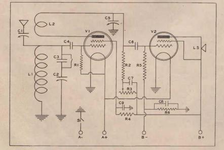
The schematic diagram which shows the circuit arrangements of the allwave receiver.
