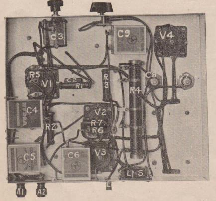
Neat wiring and convenient lay-out is a feature of the receiver as shown by this under chassis view. can be seen in the picture showing the underneath view of the finished set. Another window must be cut to take the dial. This, however, can only be worked out after the Stromberg-Carlson condenser has been mounted. A small spacing washer, about half an inch in length, serves to keep the bracket of the dial in place. This also can be seen from the pictures of the finished set.
