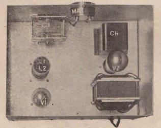
Looking inside the chassis of the finished oscillator we notice that plenty of room has been left around the coil so that no damping will be experienced.
