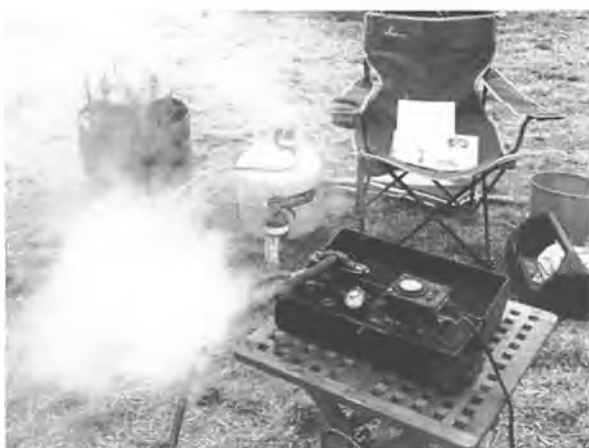
The steam powered battery charger in operation at the Echuca "Steam Fest", powered by LPG.
