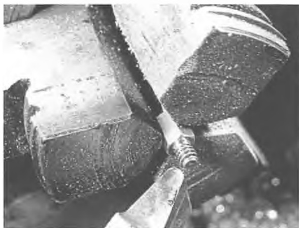
Turning off the threads of a brass stand-off as used in computers boards.
