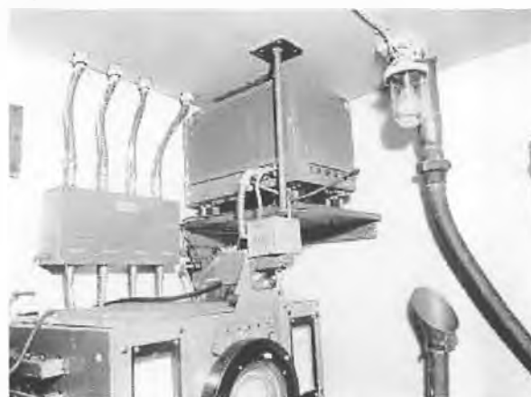
Another view of the HF/DF shipboard office with the FH4 receiver at the bottom and the FH4 power supply on the shelf. The four fat cables egressing from the deckhead are the coaxial cables for the forward/aft (F/A) and port/starboard (P/S) antenna loops. The large box with the eight cable connections is a junction box which interconnects the four coaxial cables from the FH4 to the loop antenna cables.
