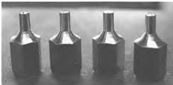
Key pivots turned up on the lathe and ready for use.
