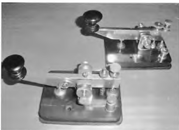
The two versions of the Levenson No 1 straight key. Nearest the camera is the 1940s model with the 1930s model, which had the coiled spring, in the background.
