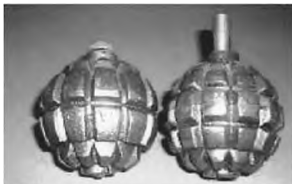
Photo 3 - 1913 German Kugelhandgranate with and without a fuze. This weighed 2 kg. The casing was machined cast iron.
