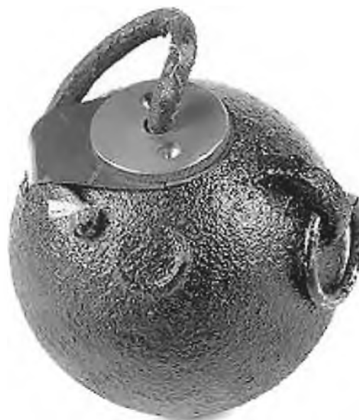
Photo 2 - The Standard Turkish Hand Grenade. Inspired by the Chinese and based on German technology, it employed low cost manufacture as evidenced by the minimal amount of machining of the casting. Initially the explosive used was probably mainly gunpowder with nitrate of baryta and potassium perchlorate as used in some German grenades, changing later to 100 gm of TNT.
