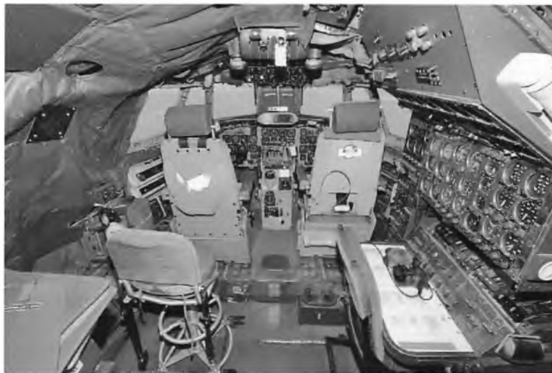
A Connie cockpit with the two Pilots' seats in the background, supernumerary to the left and Flight Engineer position to the right.
