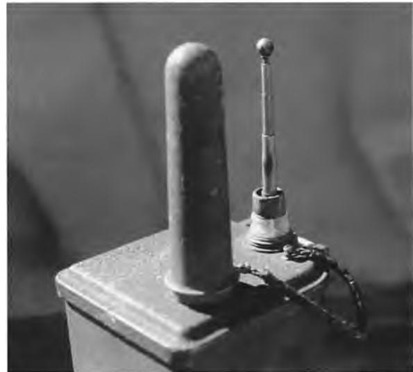
The antenna protection cap stowed and the whip antenna ready to be extended to its full length of 40 inches (101.6 cm).
