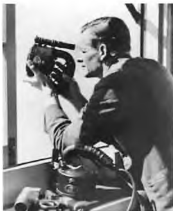
A hand held Aldis signal lamp being used.
