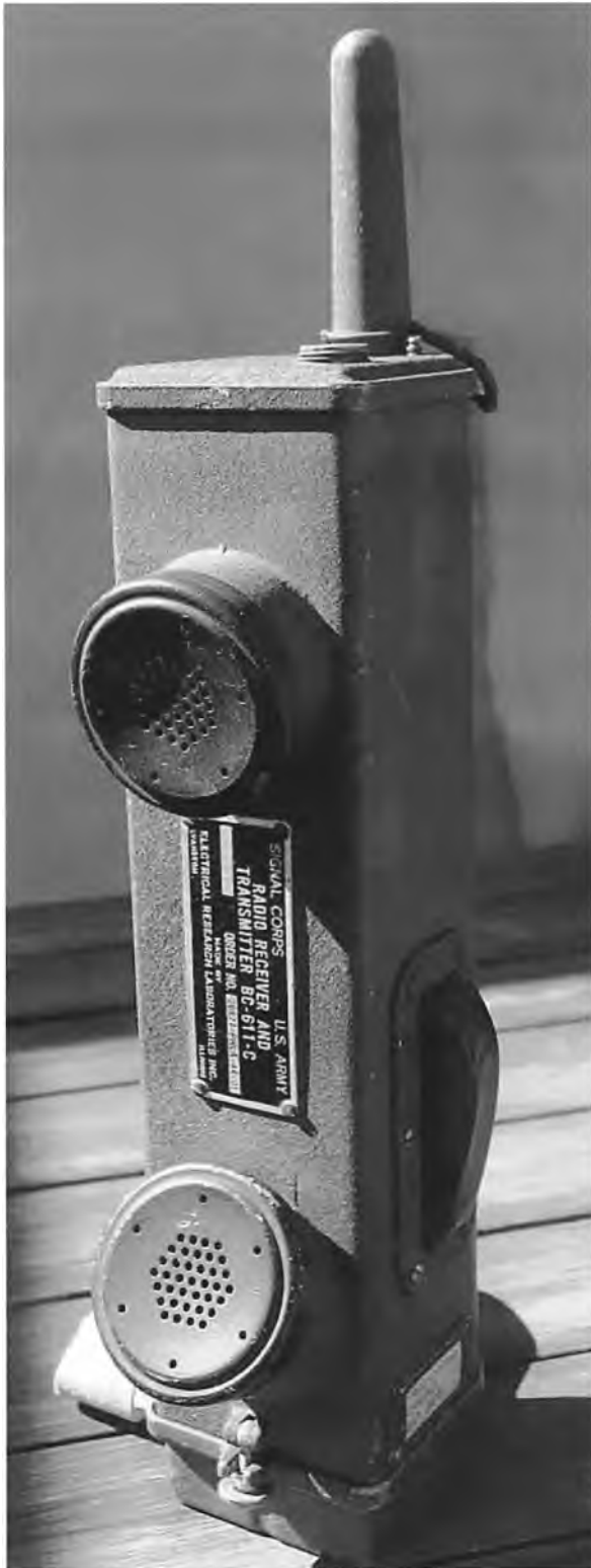
The BC-611-C walkie talkie No 13868 made by Electrical Research Laboratories Inc in Evanston, Illinois in 1944.
