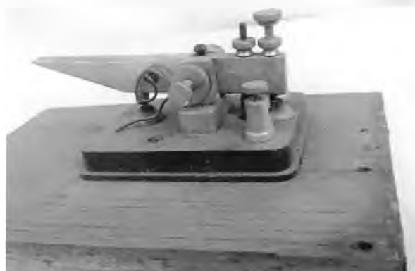
The 1930s Levenson No 1 straight key before restoration.
