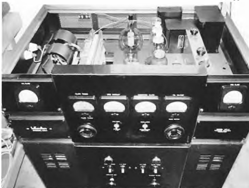
A Hallicrafters HT-4 AM/CW transmitter with the top cover removed. Note the presence of only one plug-in tuning unit.
