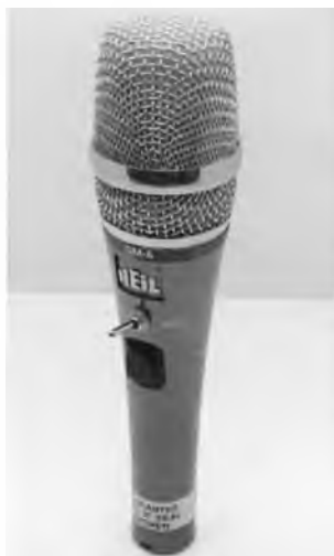
A Heil GM5 Goldline Dynamic Microphone with switchable elements between the full range HC-4 element for local high quality contacts and the restricted range HC-5.1 element, designed to be ideal for SSB DX contacts.
