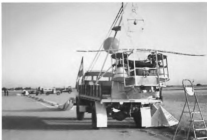
The Hibal payload and balloon laid out. Note the motor fan units either side of the payload. The payload is attached to the balloon via a cargo parachute. The launch trailer can be seen at the far end.
