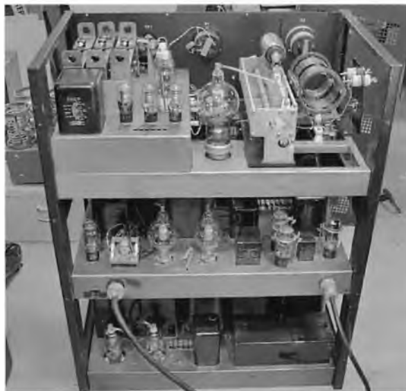
A rear view of a BC-610 with the panelling off. At the top is the RF deck with three plug-in tuning modules at top left; the modulator is on the middle deck; and the power supply is on the lower deck.
