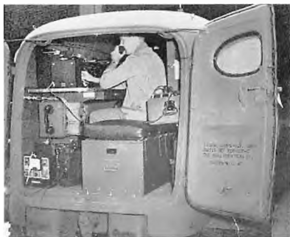
A SCR-299 installation in a Chevrolet K-51 panel van. Note the box seat containing spares and tools, etc.
