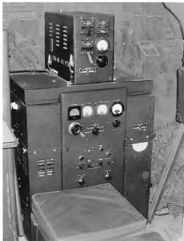
A vehicle mounted BC-610 with a BC-729 ATU above. Note the 'spares-box' operator's seat.
