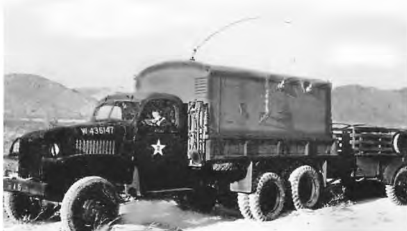
A shelter mounted version of the SCR-299 on a 2.5 ton lorry and redesignated SCR-399.
