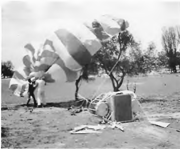
The payload has landed and strong winds have dragged the payload until the parachute entangled a tree. A fire has occurred on this occasion but fortunately there was not enough fuel to cause real damage.
