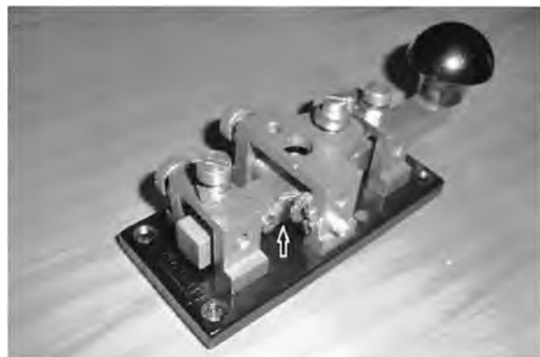
A WT8AMP Morse key with a braided brass grounding strap.
