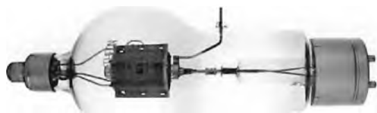
An Eimac 250TH which replaced the RK63 PA tube.
