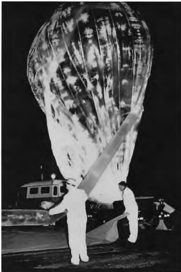
Filling the balloon - note the balloon bubble - the balloon is under a roller on the launch trailer.
