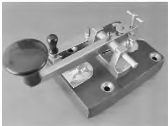
A NSW Government Railways key with its trademark crossbar and butterfly wingnut to adjust and tighten the backstop adjustment screw.
