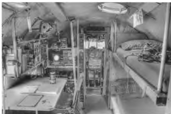
This photo shows the location of the Radio Operator, the Navigator and the crew bunks in the cabin. Note the astrodome in the top of the fuselage to enable the Navigator to take 'shots' of celestial bodies with a sextant.
