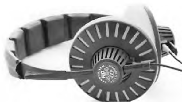
Sennheiser 'open architecture' headphones similar to the HD414 first sold in 1967.
