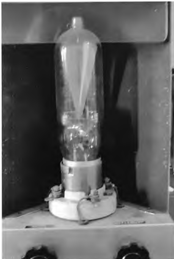
The Type AV 43 CRT tube with power applied. The partially obscured knobs are 'Focus' and 'Deflection'. In colour, the lightish grey elongated triangle of light commencing from roughly the centre of the glass portion of the tube envelope and proceeding to the top right, is a vivid green.
