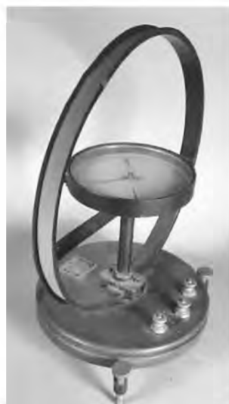
Figure 3 - A vintage tangent galvanometer by Milvay.
