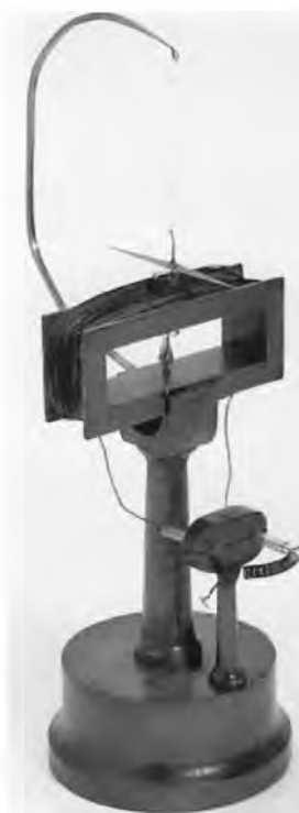
Figure 1 - The Schweigger multiplier galvanometer.
