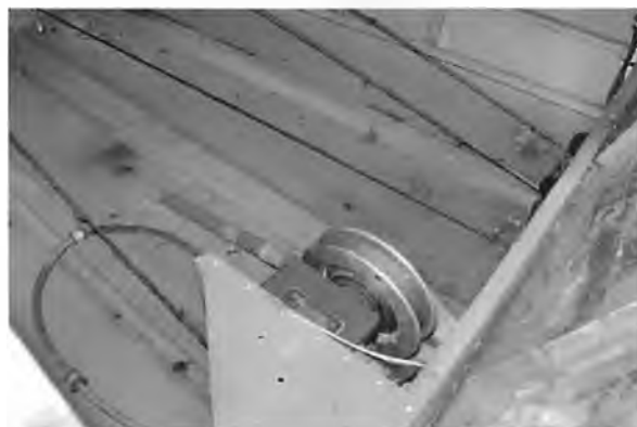
The Southern Cross antenna reel and Bakelite insulator tube.
