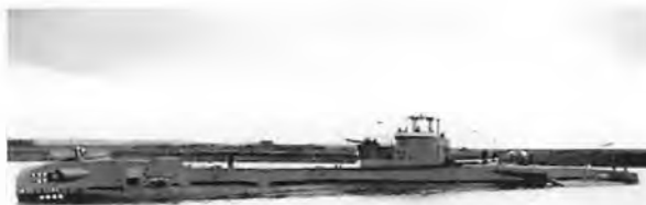
HMS Telemachus was 84.3 m in length and 1,560 tons submerged. Launched in 1943, she was diesel powered, had a range of 8,330 km at 20 km/h surfaced, and carried 17 torpedoes.
