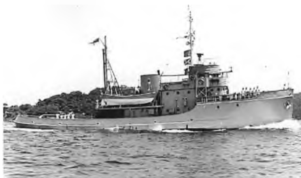
HMAS Sprightly was 44 m in length and had a top speed of 16 knots (30 km/h).
