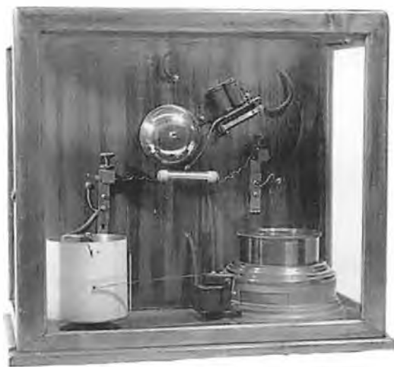
An early Popov receiver with ink recorder to record lightning strikes.
