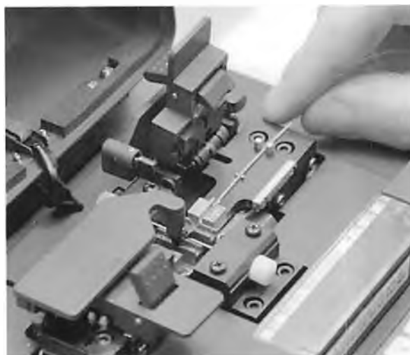
Figure 9 - Preparing an optical fibre end for splicing with another fibre end.
