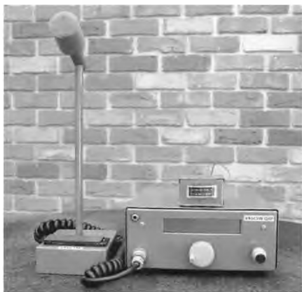
The QRP rig complete with home brew matching microphone and 'S' meter.
