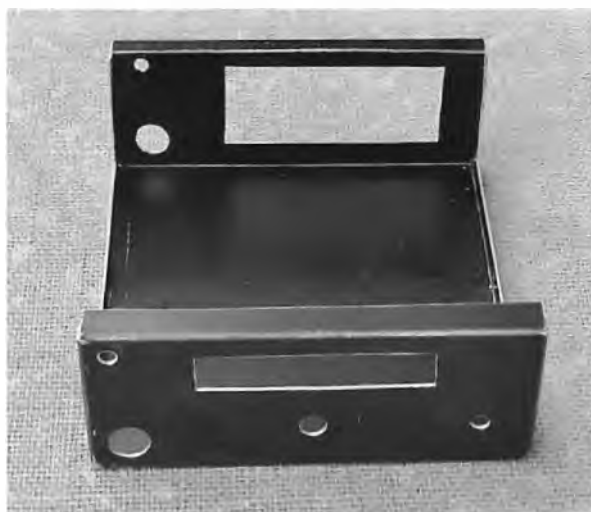
The home brew case constructed by the author for the 'little mouth, big ears' QRP transceiver.
