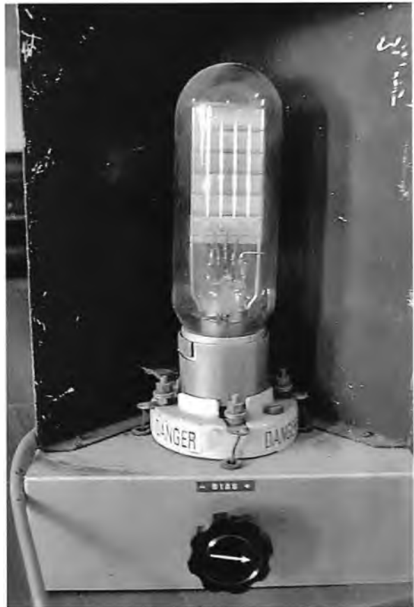
The Type AV 25 Triode with power applied. The knob at front is labelled 'Bias'. In colour, the rectangle of light in the top part of the glass envelope is a bright green and the four vertical bars are a brilliant green.
