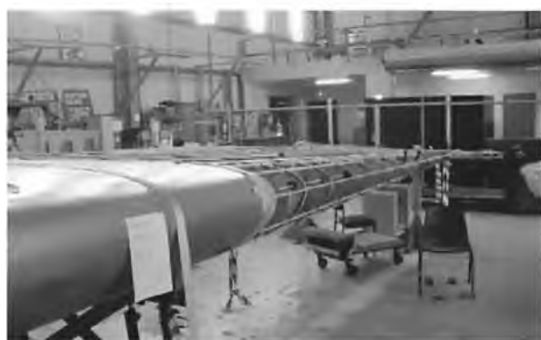
The Southern Cross replica's right wing under repair at HARS.
