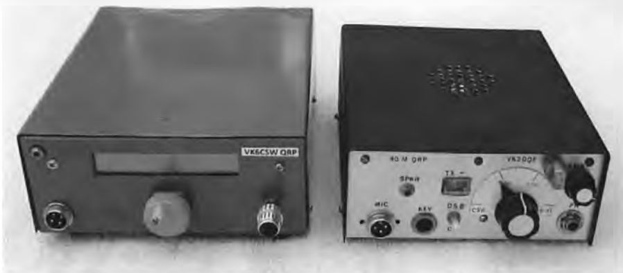
The author's homebrew 40 m SSB and DSB rigs alongside each other.
