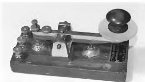
A Navy Morse key 'liberated' from the junk box at the training school at HMAS Cerberus in 1955. The broken knob skirt needed to be replaced. It still works very well.
