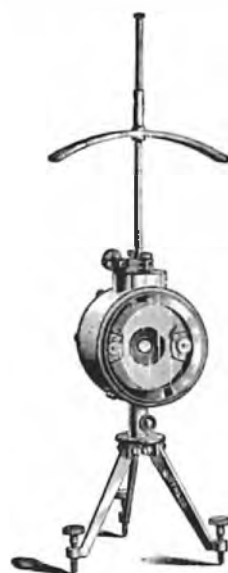
Figure 5 - Thomson mirror galvanometer as used on the first transatlantic cable. Note the bar magnet to cancel the earth's magnetic field.
