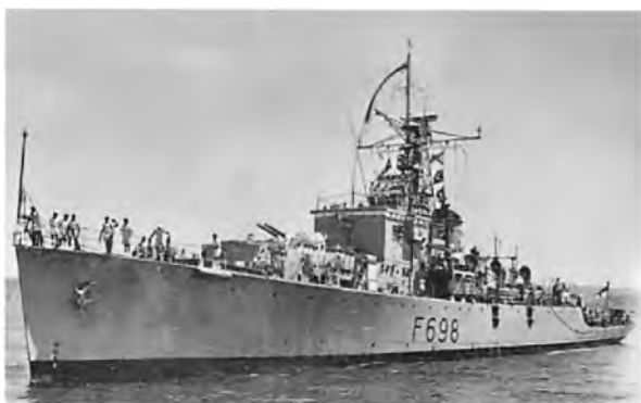
HMAS Condamine, 2,200 tons, 92 m long, 19.5 knots (36.1 km/h) top speed, 4 x 4 inch (100 mm) guns, 3 x 40 mm Bofors, 4 x 20 mm Oerlikons, 1 x Hedgehog and 4 x Depth Charge Throwers.
