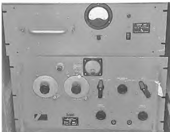
A crystal locked R1392 airband receiver, which replaced the R1132, with power supply above.
