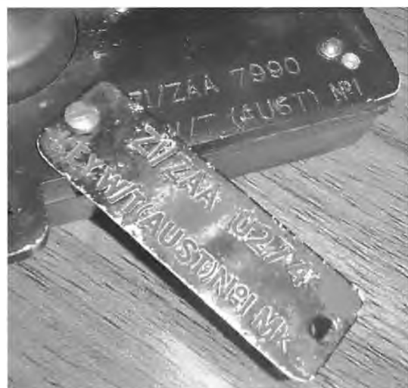
An original Z1/ZAA 7990 key showing how the metal plate changing it to an 0274 key was mounted.
