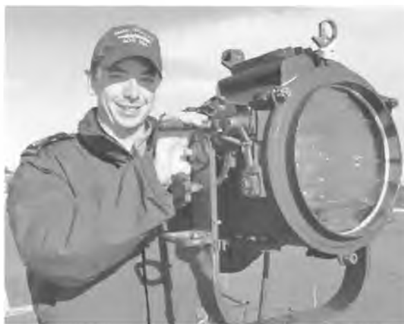
A typical large Naval, pedestal mounted, shutter operated Aldis lamp aboard HMAS Success , the Australian-built Durance -class multi-product replenishment oiler serving in the Royal Australian Navy since the 1980s.
