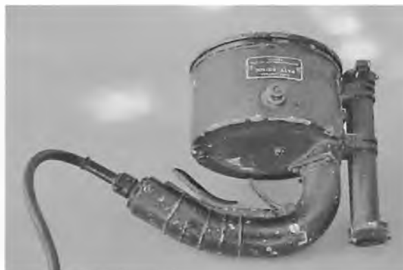
A typical Aldis lamp used by the Merchant Marine. Note the two 'triggers' on the handle.
