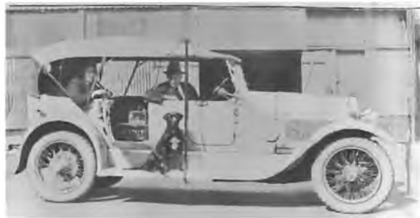
A 1923 Lancia Trikappal. The police were showing the 7-stage receiver with a tuning condenser they were using for short range transmissions. The antenna was a piece of wire hung over the pole clamped onto to the running board.
