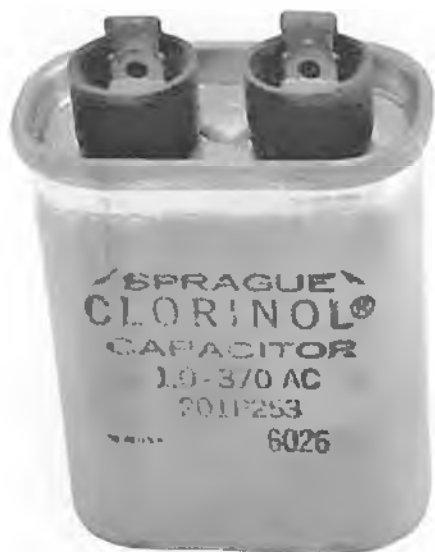
A typical Sprague Clorinol capacitor which used PCB oil!
