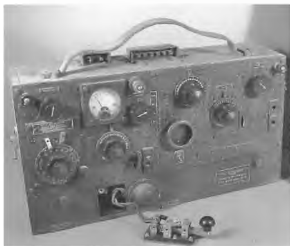
An AWA FS 6. Wireless sets of this kind were used by the military to communicate with personnel over longer distances than smaller portable units were capable of. They were normally carried in specialised radio vehicles or transported by a small number of men who would then establish a base or relay station. There is provision for a microphone in addition to the Morse key.
