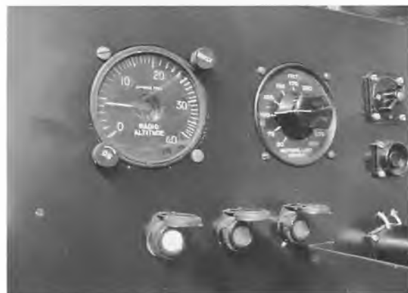
An APN-1 radio altimeter showing height readout, altitude limit selector switch, and warning lights beneath.
