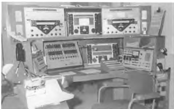
Aeradio radio room on Thursday Island - note the flightstrip board and AWA receivers CR-6B and CR-3D. The large sliding window was to the right.
