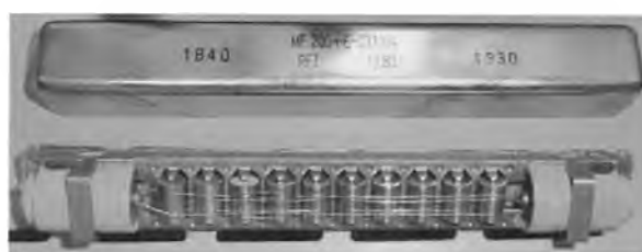
Fig 6. Mechanical filter from a telephone carrier system using torsional resonator elements.
