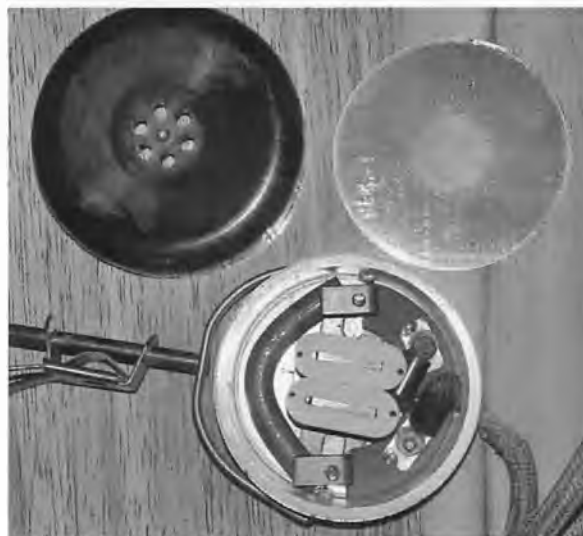
A close look at the components of an earpiece of the Cannon-Ball Master headphones.
