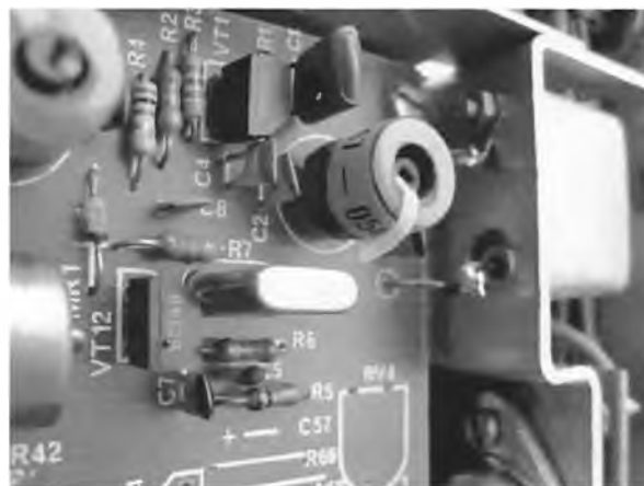
The wiring to the second mixer of the radio with the 29.80 MHz crystal filter at the far right.
