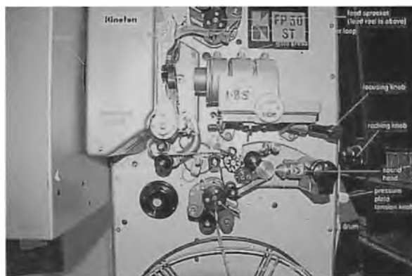
Projector assembly with sound on film.
