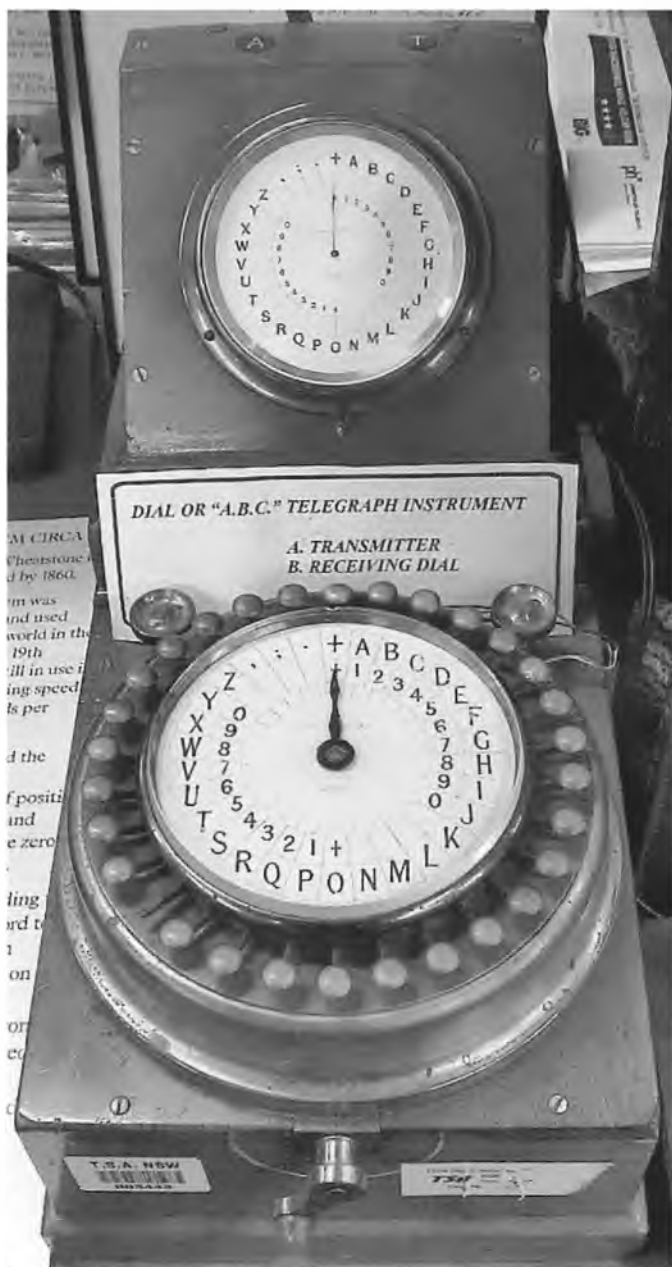
The Wheatstone ABC electric pointer Telegraph on display at the Telstra Museum in Bankstown, NSW.
