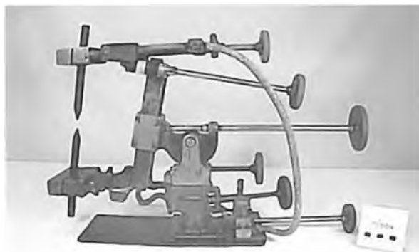
Early carbon arc 1920-1930 era (removed from the projector).
