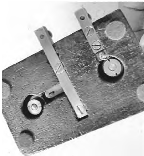
The underneath of the Morse hand key after full restoration.
