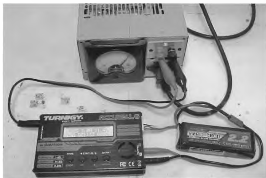
The author's Turnigy Accucell 6 multifunction charger charging a 2.2 Ah 20C nanocell battery using his homebrew DC supply. Note the main charging leads and the smaller balance leads
