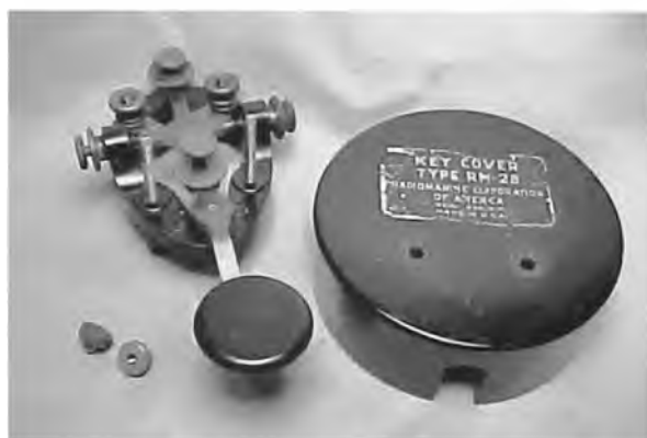
An RCA RM-28 Morse key with cover as used on the Tjibantjet
