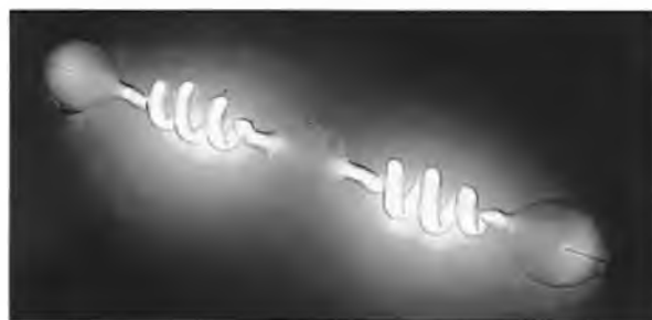
Fig 2. The centre globe of this Geissler tube is made from uranium glass and glows green under discharge.
