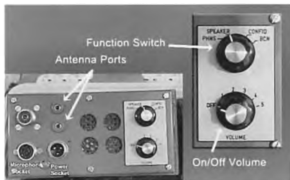
The HeyPhone control panel with an internal speaker between the connectors and the rotary controls.
