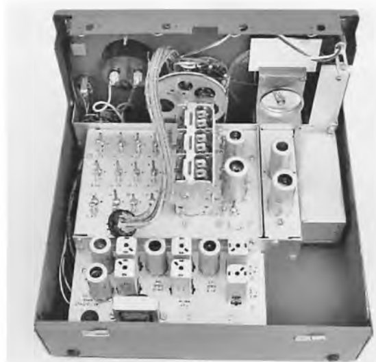
A top of chassis view of the Sprague 500 - note the many trimmer and inductance adjustments.
