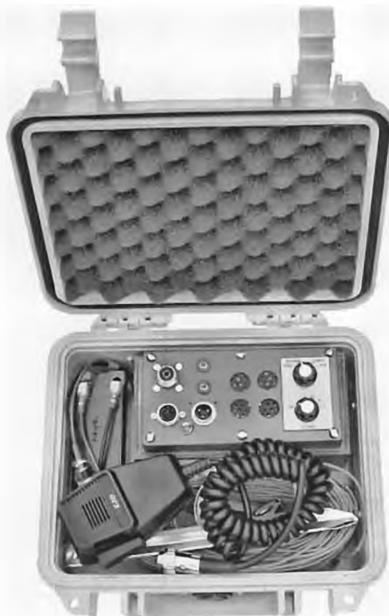
HeyPhone, battery, microphone, and earth antenna wire, etc, all packed in a waterproof Pelicase.
