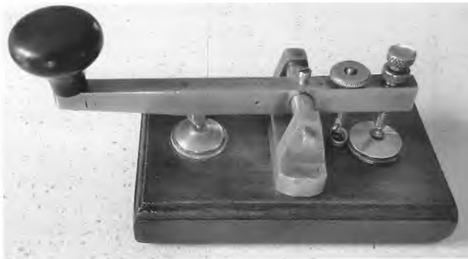
The fully restored Morse hand key.
