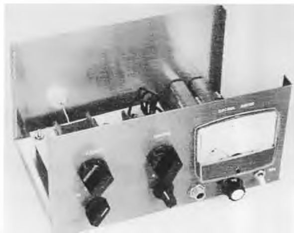
Field strength meter picture (ARRL Handbook).
