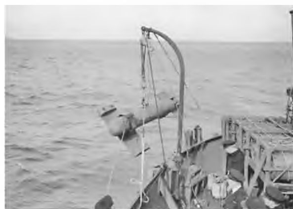
One of a pair of underwater mine clearing paravanes, similar to those installed on HMHS Tjitjalengka , being lowered for a sweep.
