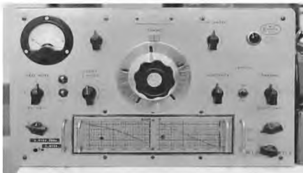
A Kingsley AR7 receiver identical to that used by the Australian Special Wireless Group.
