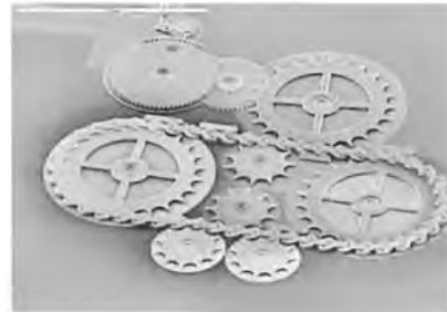
Figure 2a. The chain in this MEMS gear set is thinner than a human hair. Total width is less than 1 mm.
