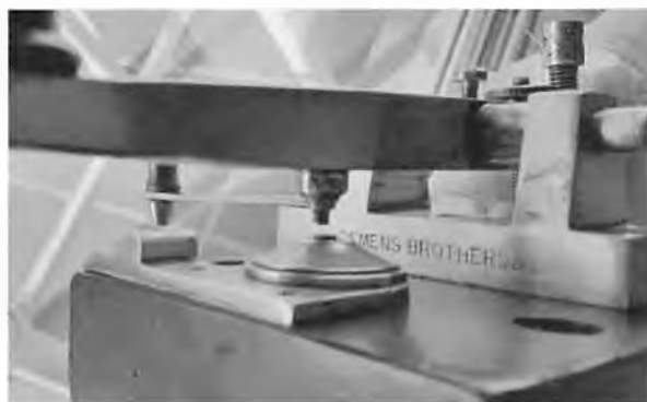
A close-up of the fulcrum of the rare, pre 1880 Morse key, stamped with 'SIEMENS BROS & Co'.
