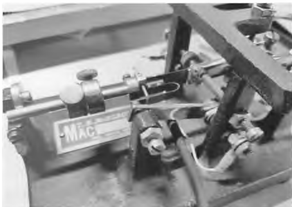
Dot spring stabiliser on a McElroy T-bar Mac bug key.
