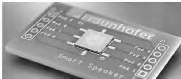
Figure 10. Fraunhofer, the German research institute is developing both piezo and capacitive (electrostatic) all-silicon MEMS-speakers. Its CMOS-compatible MEMS speaker is based on electrostatic bending.
