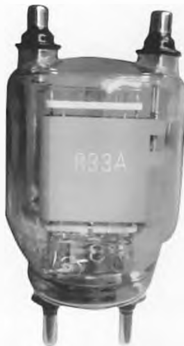
A photo of an 833A transmitter tube similar to the one given to the author by Noel Ferguson, then VK3ZGZ, around 1960.
