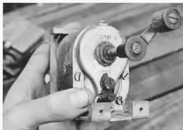
The magneto from a 1940s British Army Field Telephone Type F Mk II which the author found in his box of miscellaneous wireless 'goodies'.
