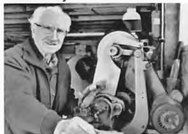
John Daniel making a brass terminal screw for my Siemens Bros & Co Ltd key.
