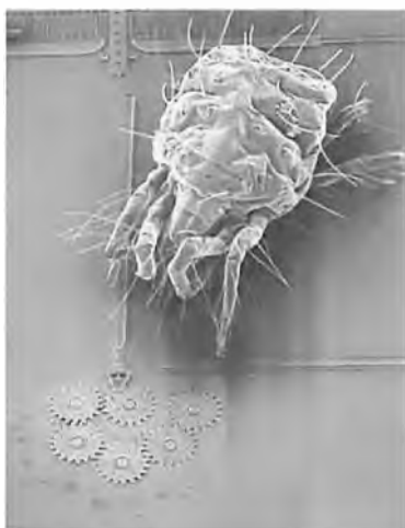
Figure 2. A gear chain with a dust mite approaching.
