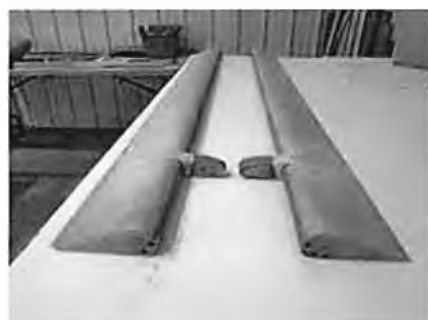
Fig 5a. Internal mass balances on the control surfaces.
