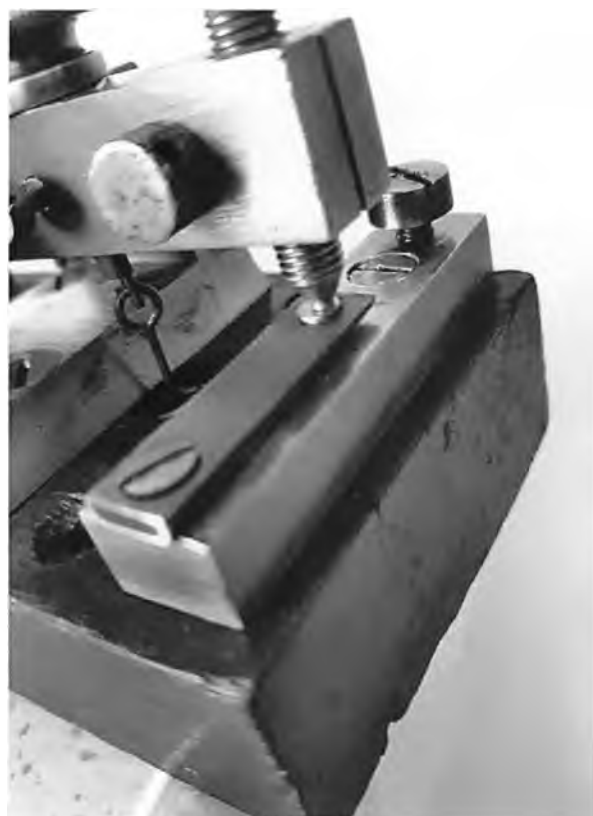
A closer look at the rear contacts of this key sitting on a stiff metal leaf spring.
