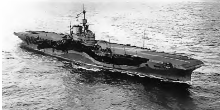
HMS Formidable , a WWII Illustrious class aircraft carrier of 23,370 tons, carried 36 - 54 aircraft and had a top speed of 30.5 knots (56.5 km/h).
