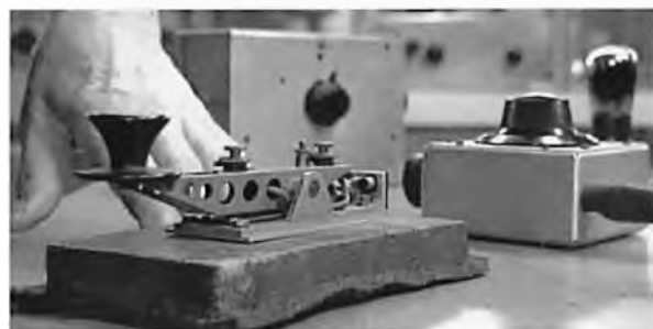
An NSF key used by the Dutch resistance in WWII.
