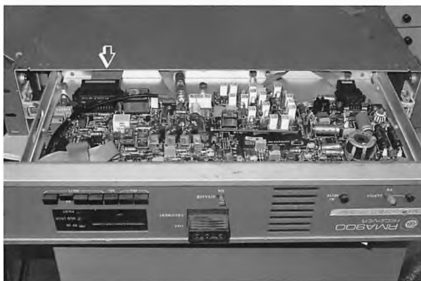
A view under the chassis of an AWA RMA 900 Receiver. This one is very similar to the one used by K-Rock and Bay FM as a Studio Link. Much of the offending signal was radiated by the ribbon cable at top left.
