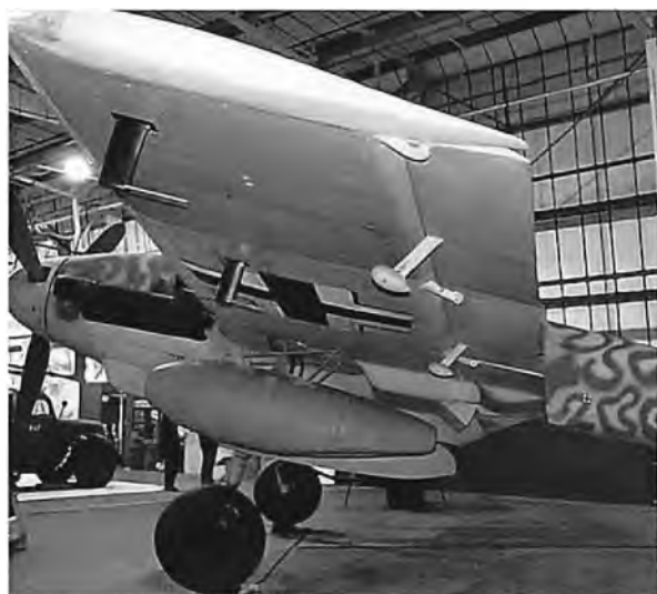
Fig 5. External aileron mass balance on a Messerschmitt Bf 110.
