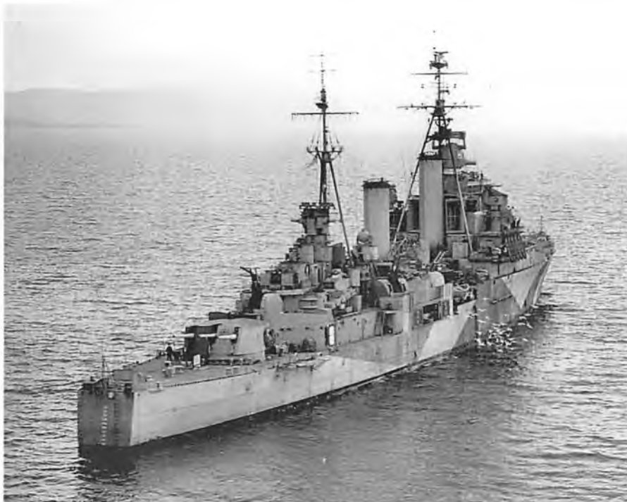
HMS Swiftsure , a WWII Minotaur-class light cruiser of 8,800 tons had a top speed of 31.5 knots (58.3 km/h) and an armament including three triple six inch naval guns and five dual four inch guns.
