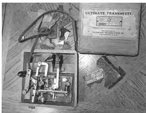
Amateur pot metal model Ultimate 73 bug No 13968 totally disintegrated.
