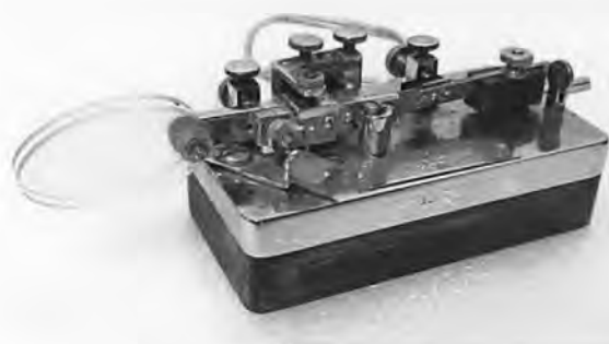
An Ultimate 73 in-line model bug.
