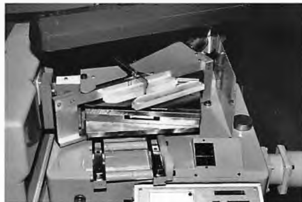
A cultured quartz bar mounted in an X-ray machine ready for an X-ray diffraction measurement. You can see the cultured quartz bar. The bar is mounted on a base on which it will be cut, and held in place with a clamp arrangement.
