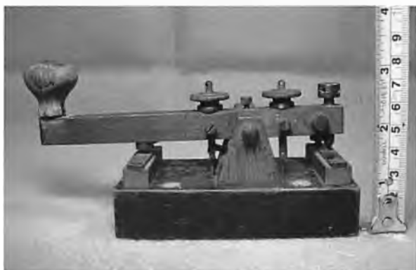
Herman's rare Russian Morse key as received, dirty and with a busted wooden knob.
