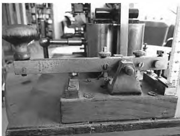
A similar small Russian key as part of an inker telegraph set from the beginning of the 1900s. Note the hole for the missing retainer ring.
