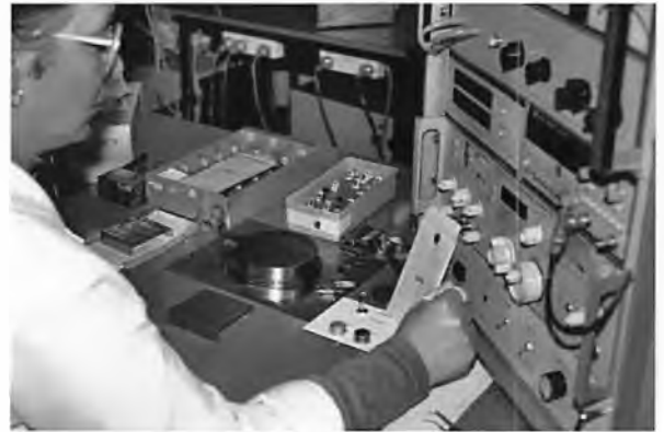
A close up an 'Evaporator' that places the final 20% of silver on the quartz blank. Here the operator can be seen looking at the customer's order and ensuring the required frequency (and tolerance) is achieved.
