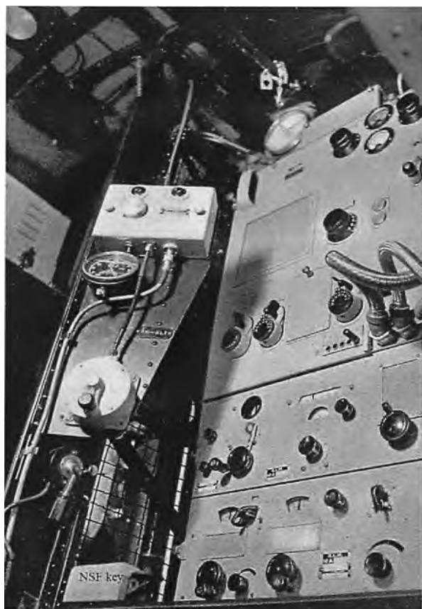
1937 NSF radio equipment VR35 in DC-3 Torenvalk, PH-ALT.
