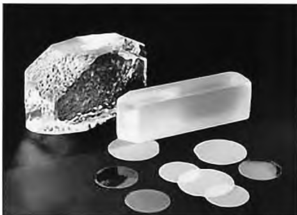
An example of a cultured quartz bar, with finished quartz crystal blanks in the foreground.
