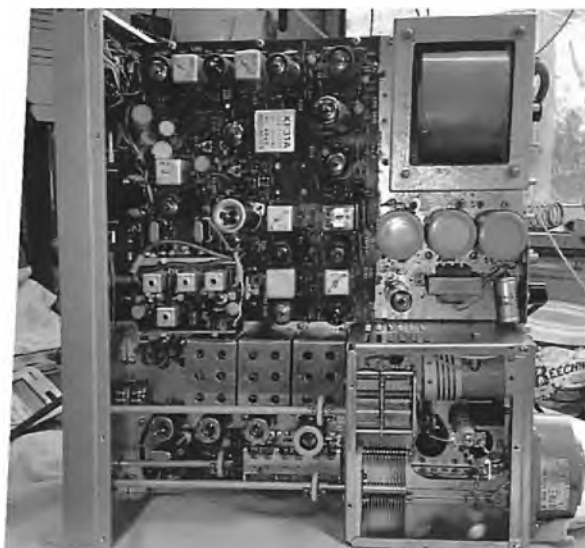
A view of the top of the chassis construction of the restored FTDX570. Again a very typical 1970s layout.
