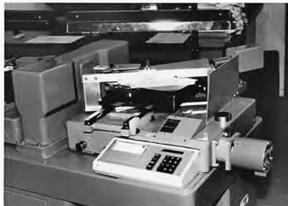
Another view of the same machine, with the keypad for control and stepper motor on the right-hand side.
