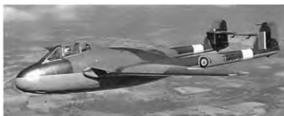
Fig 6. A de Havilland Vampire. The mass balances under the elevator are clearly visible.
