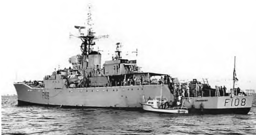
HMS Londonderry (F108) was a Rothesay or Type 12 class anti-submarine frigate in service from 1960 to 1984. She was 110 m long with a beam of 12 m and a top speed of 30 knots (56 km/h). Armament was twin 4.5 inch (British) Mark 6 guns, a Sea Cat GWS-20 SAM, two 20 mm Oerlikon guns, a Limbo A/S mortar Mark 10, and a Westland Wasp HAS 1 helicopter.
