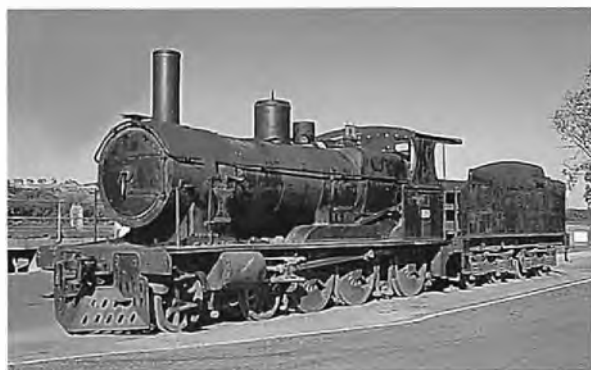
An early Rx steam locomotive (broad gauge) displayed at the Murray Bridge Wharf and built by Islington Workshops in South Australia. It is of a similar design to that used on the narrow gauge Ghan line in the early days.
