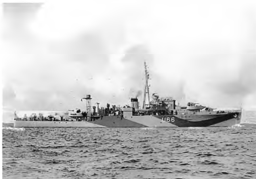
HMS Starling (U66) was a WWII Black Swan class sloop, reclassified as a frigate in 1947. She was credited with sinking 14 U-boats during WWII. Her armament included six 4 inch AA guns, four by two pounder (British) 40 mm AA pom-poms, twelve 20 mm Oerlikon (Swedish) AA guns and eight depth charge throwers. She had a top speed of 20 knots (37 km/h) and was captained during the Battle of the Atlantic by the famous Captain F J Walker until his untimely death in July 1944.
