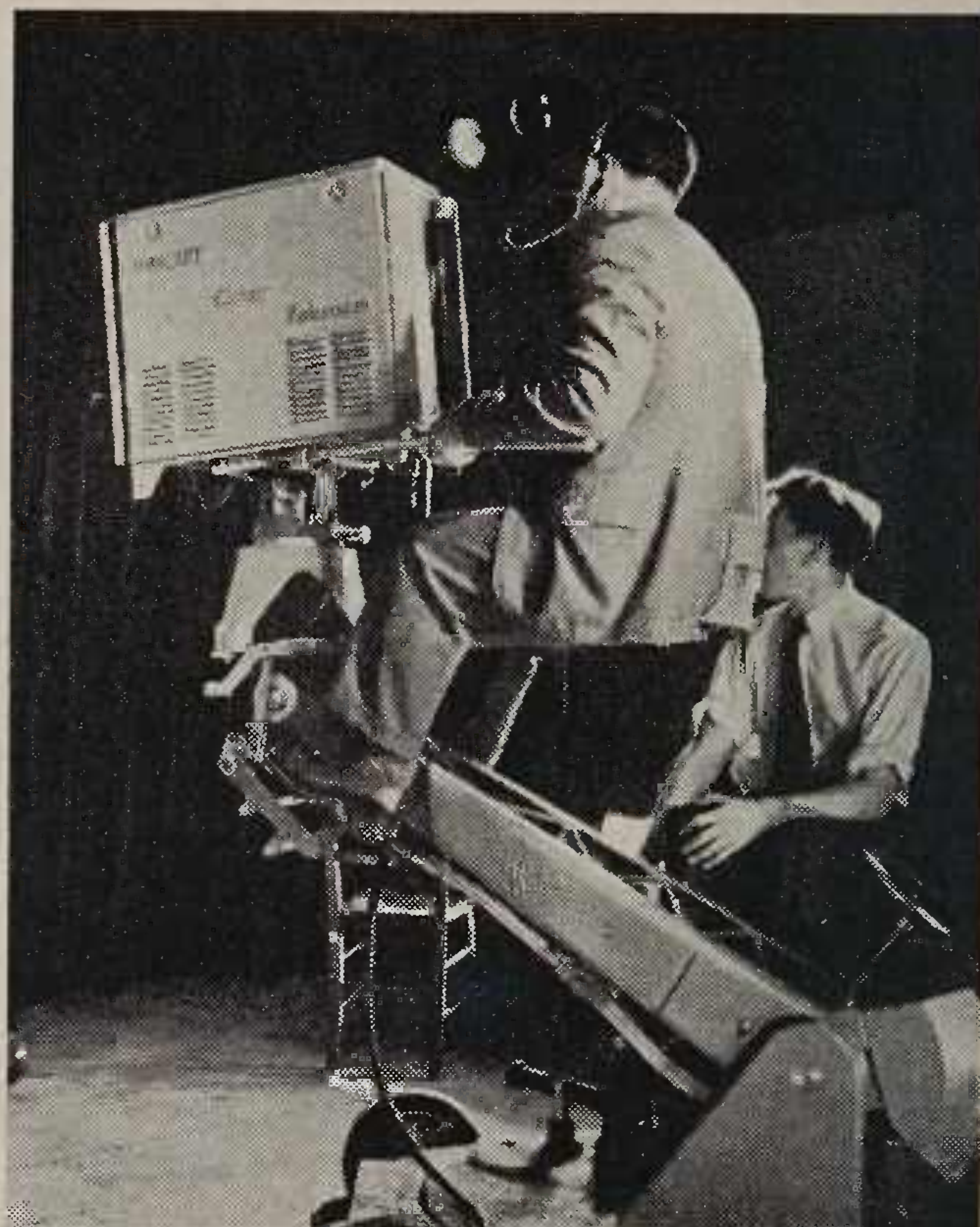
Another view of one of the Colour Cameras which were specially developed by the Marconi Company for the demonstration. Being experimental equipment, it does not include a view-finder, but its small size is noteworthy, in that it includes the two camera tubes necessary for generating the colour.
