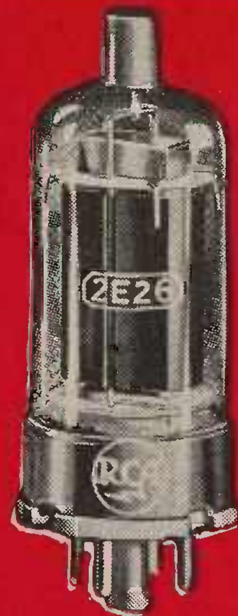
RCA-2E26 Beam Power Tube. Up to 40 watts ICAS input on cw; 27 watts phone. Full input up to 125 Mc; reduced input up to 175 Mc. Well-suited for mobile services. A 6AG7 drives it; a pair of 6V6-GT's, or a 6N7, modulates it.
