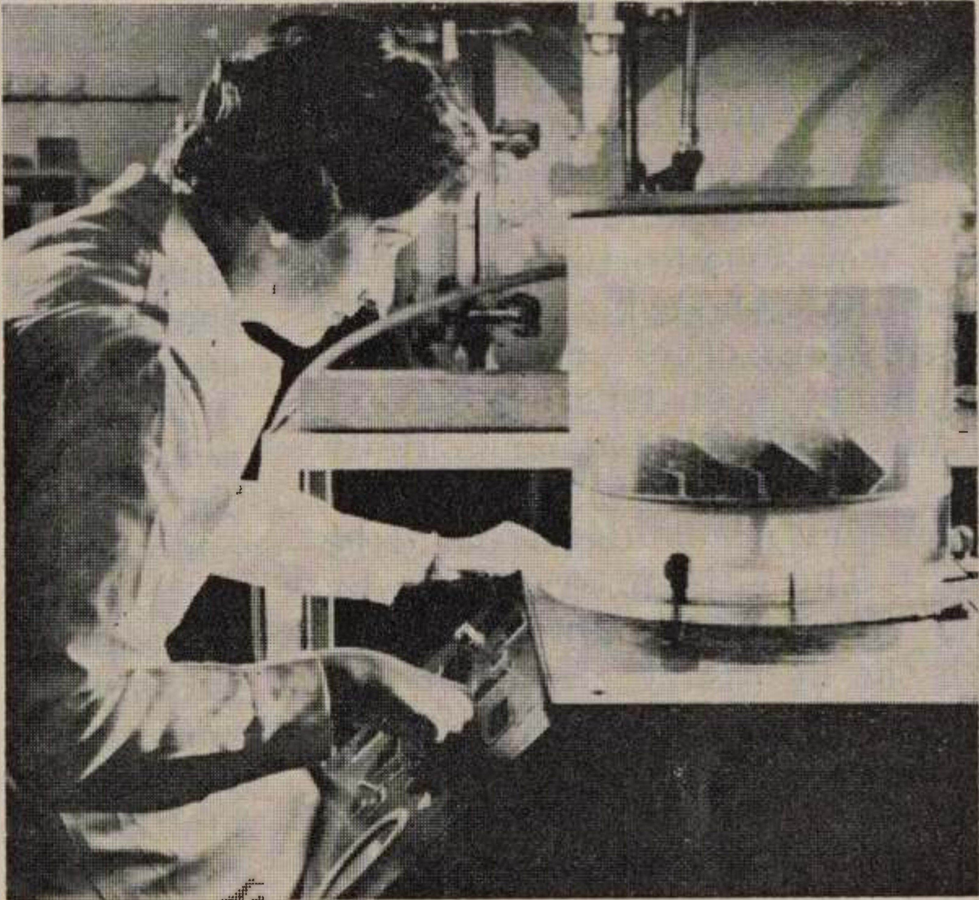
relay cans being checked for air leaks.
