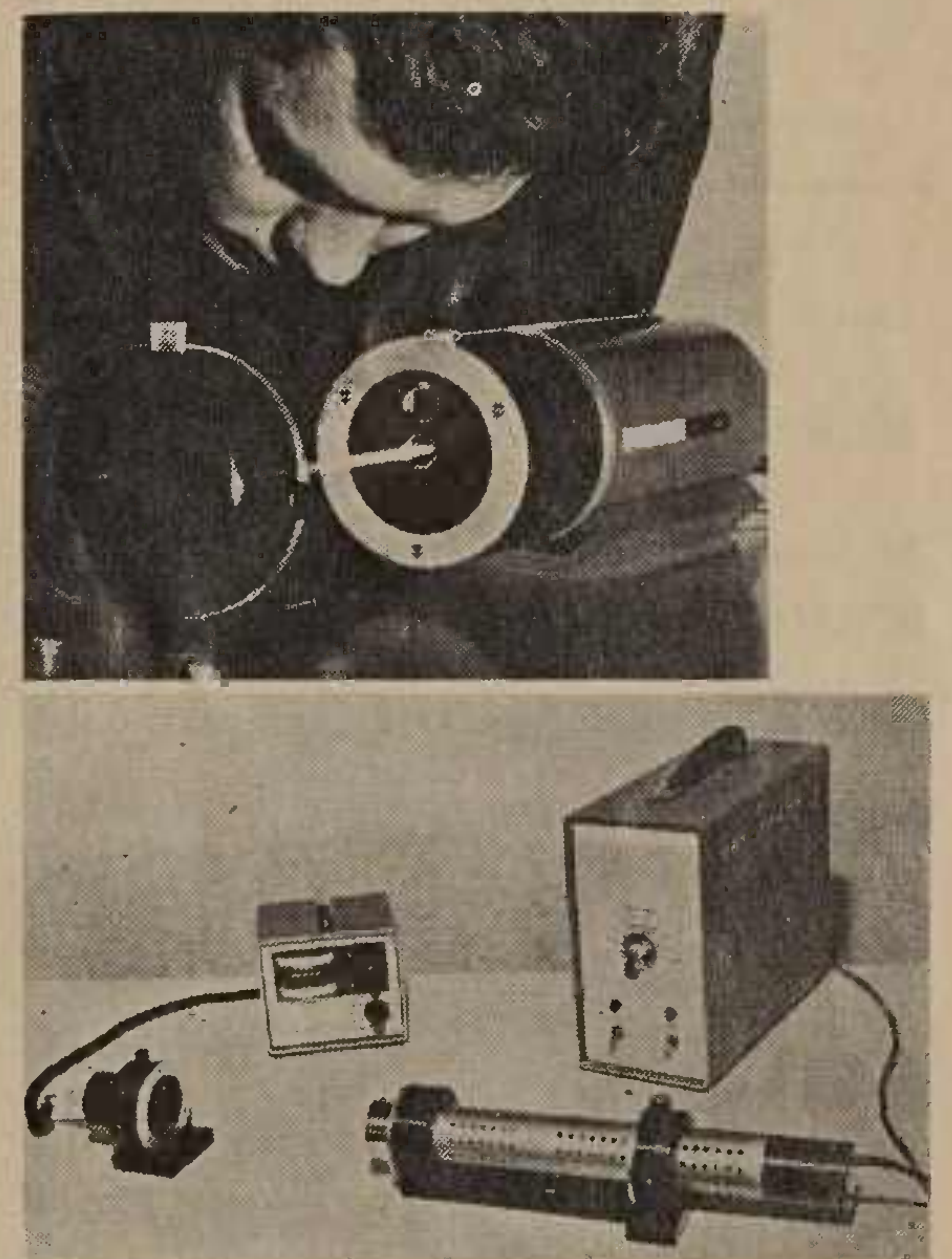
Top: Pilkington Perkin-Elmer's laser interferometer. A beam from the laser (right) is returned from the retro-reflector (left) to the interferometer contained in the laser housing and linear displacement is indicated on a digital counter.
