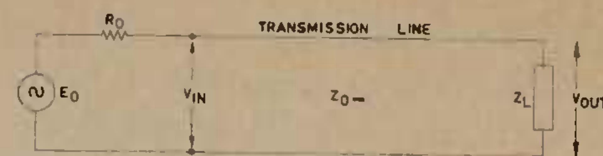
Figure 1: A correctly terminated cable. Z_L = Z_0
