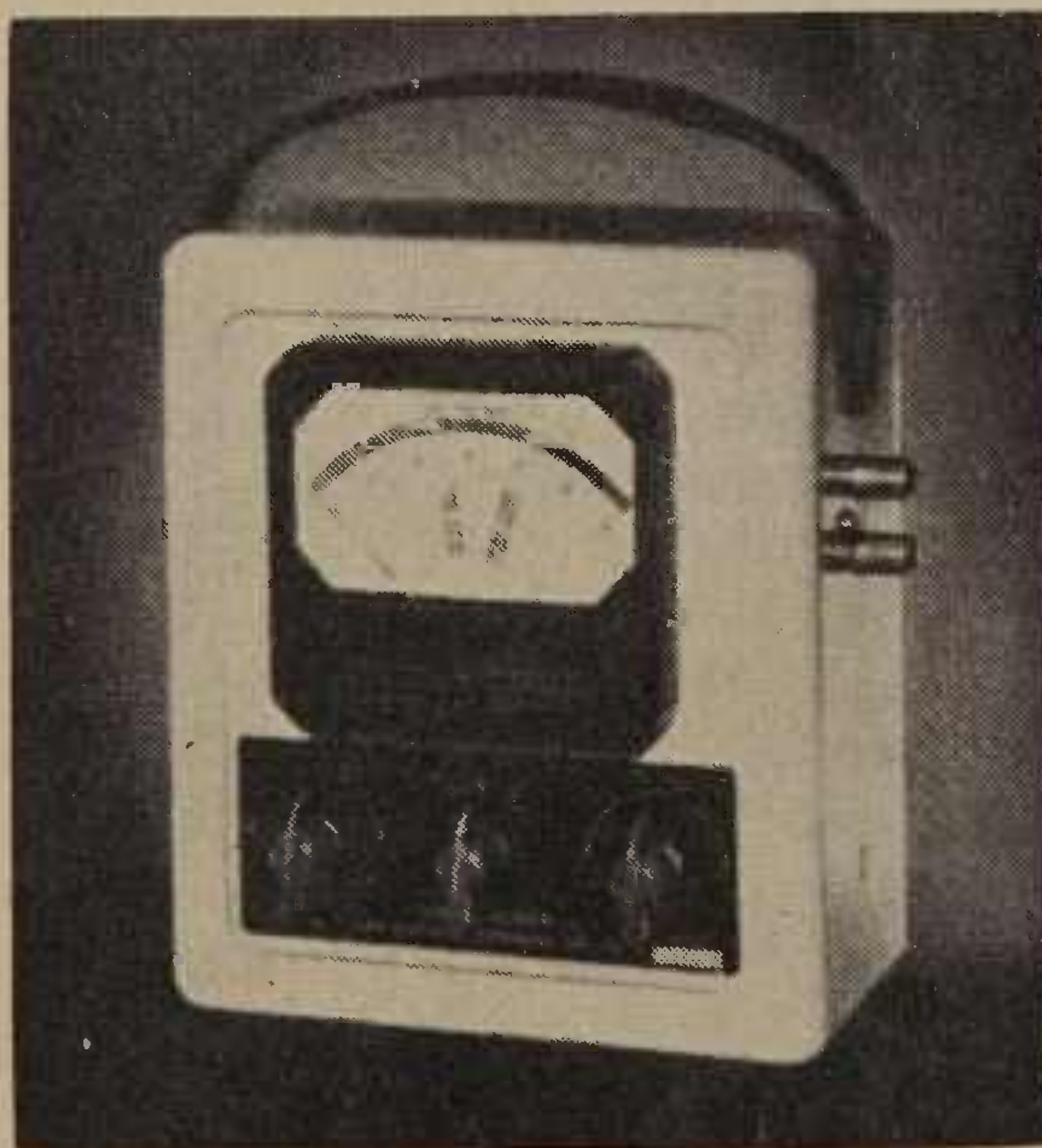
An individual test instrument—an exhaust gas analyzer.
