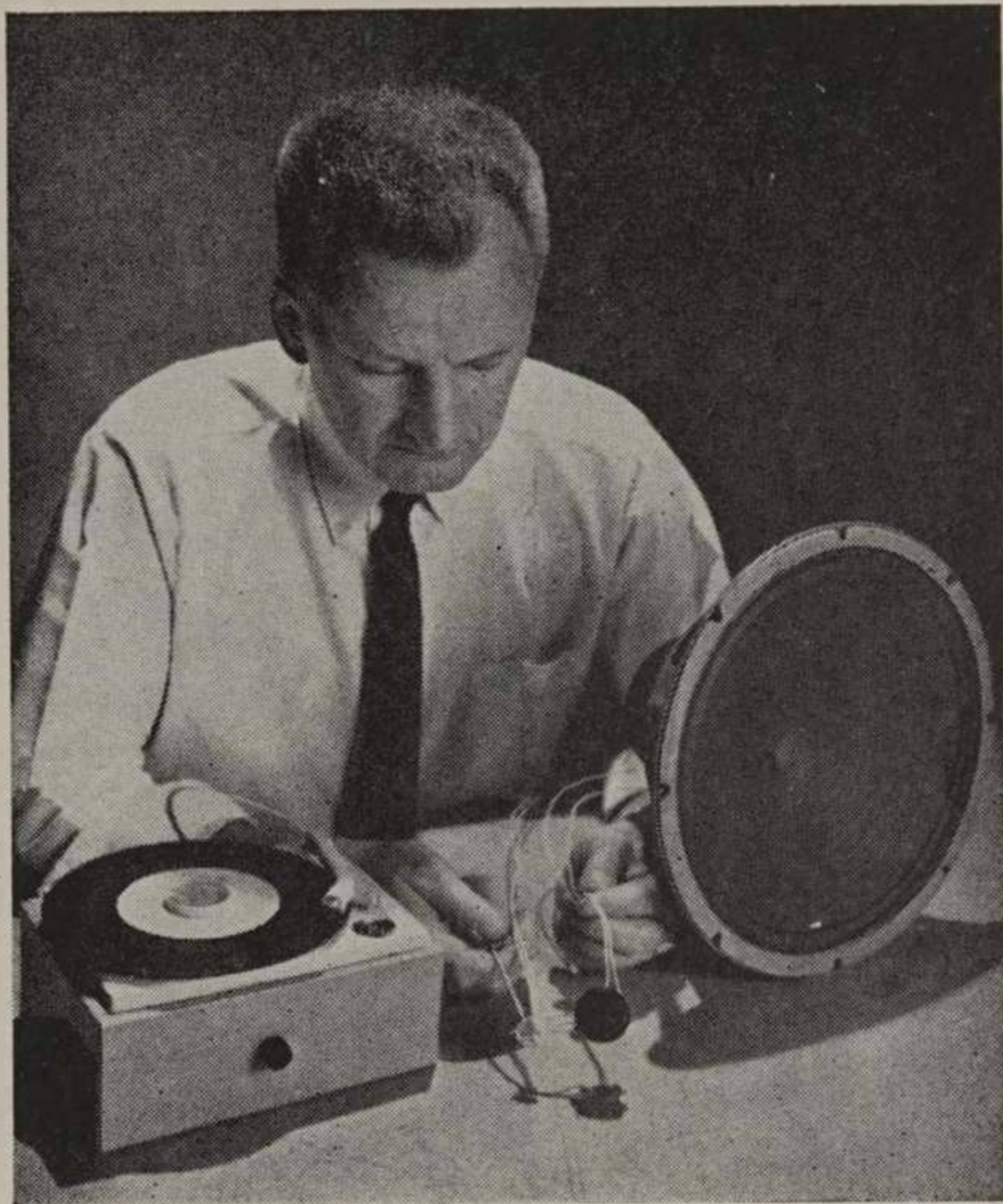
Demonstration of molecular electronic function block as audio amplifier in conventional phono system. Frequency range is 0 to 20,000 cycles, output is 5 watts when heat sink is used. Amplifier itself (at right in black mounting) is tiny device whose volume is about 0.001 cubic inch. Device to the left is a molecular electronic pre-amplifier.
