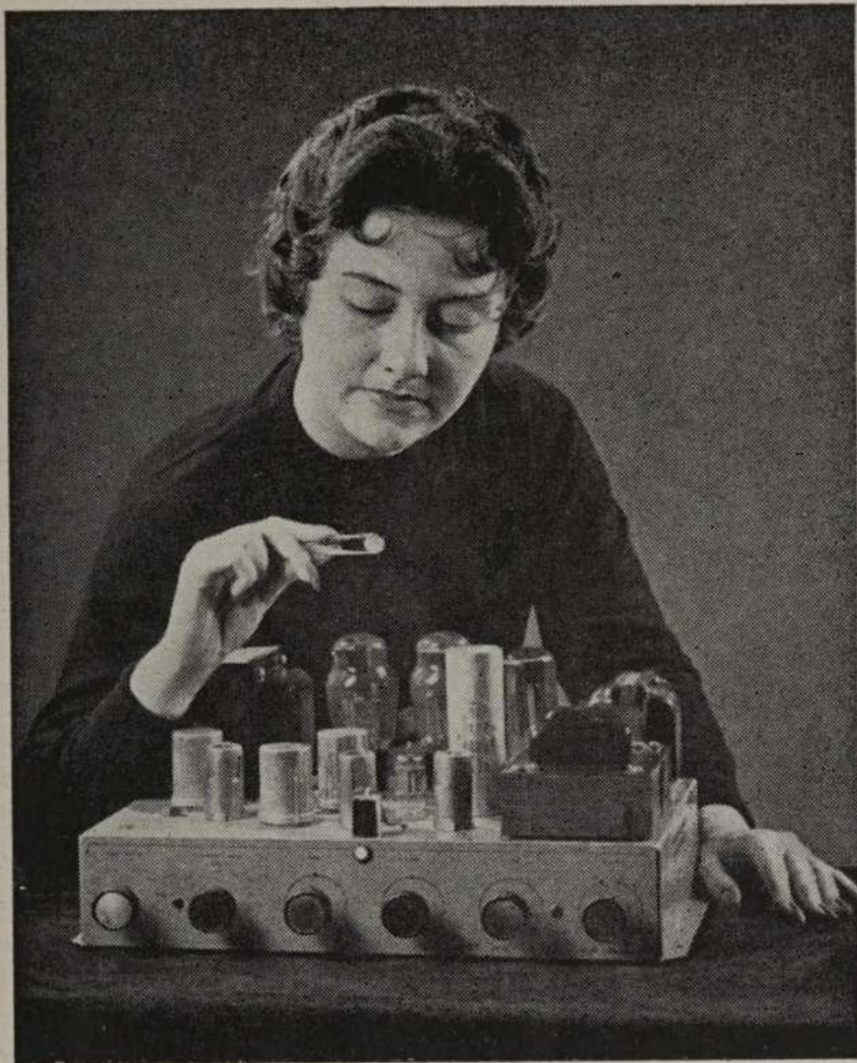
The button-like object, smaller than a United States 10-cent piece, being held with a pair of tweezers, is actually a molecular electronic amplifier which performs the same function as the conventional amplifier on the table.
