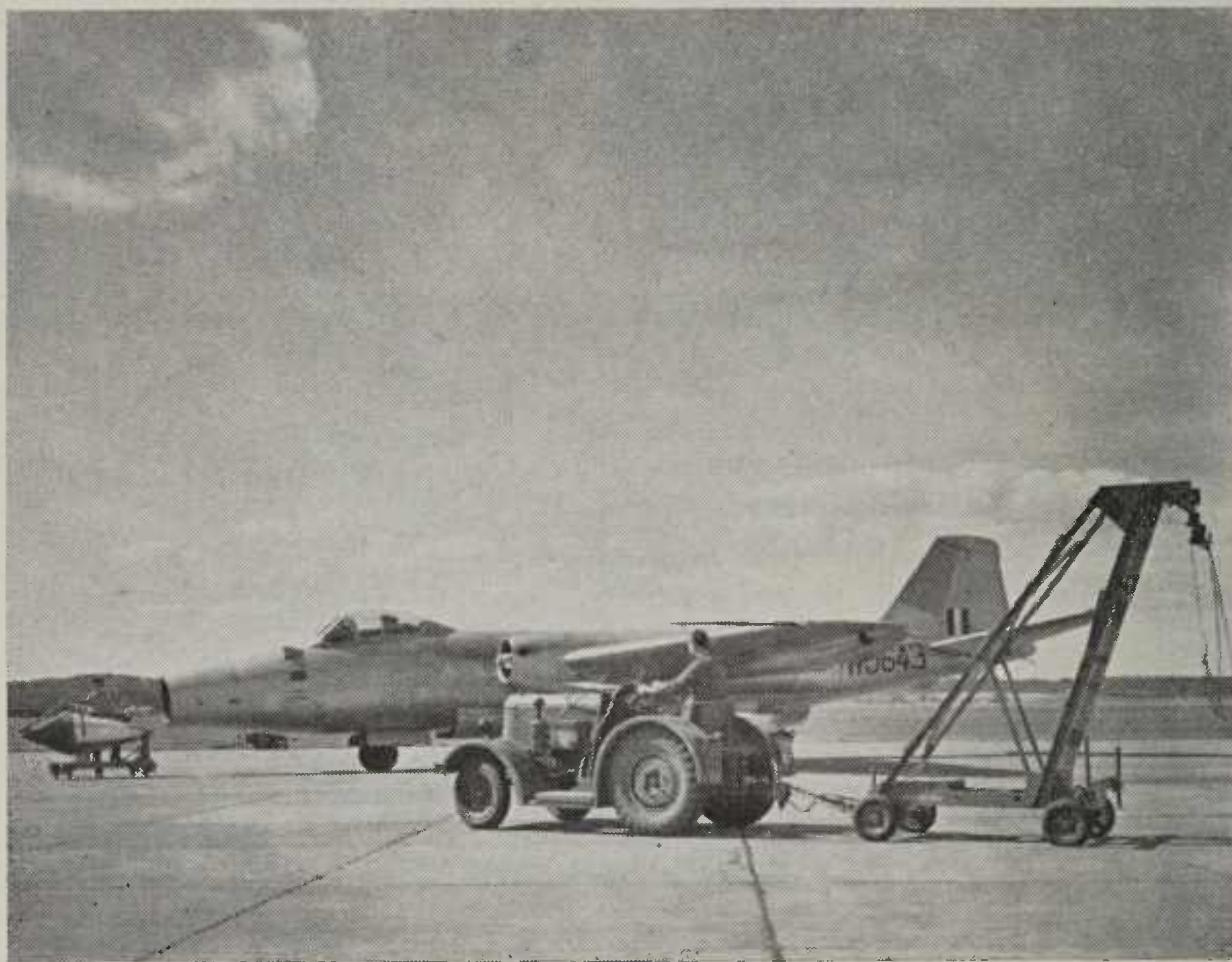
Ferranti airborne radar and fire control equipment known as AIRPASS was on view to the public for the first time when the annual Flying Display and Exhibition of the Society of British Aircraft Constructors was held at Farnborough, Hampshire, England. AIRPASS being loaded into the nose of a Canberra for test.
