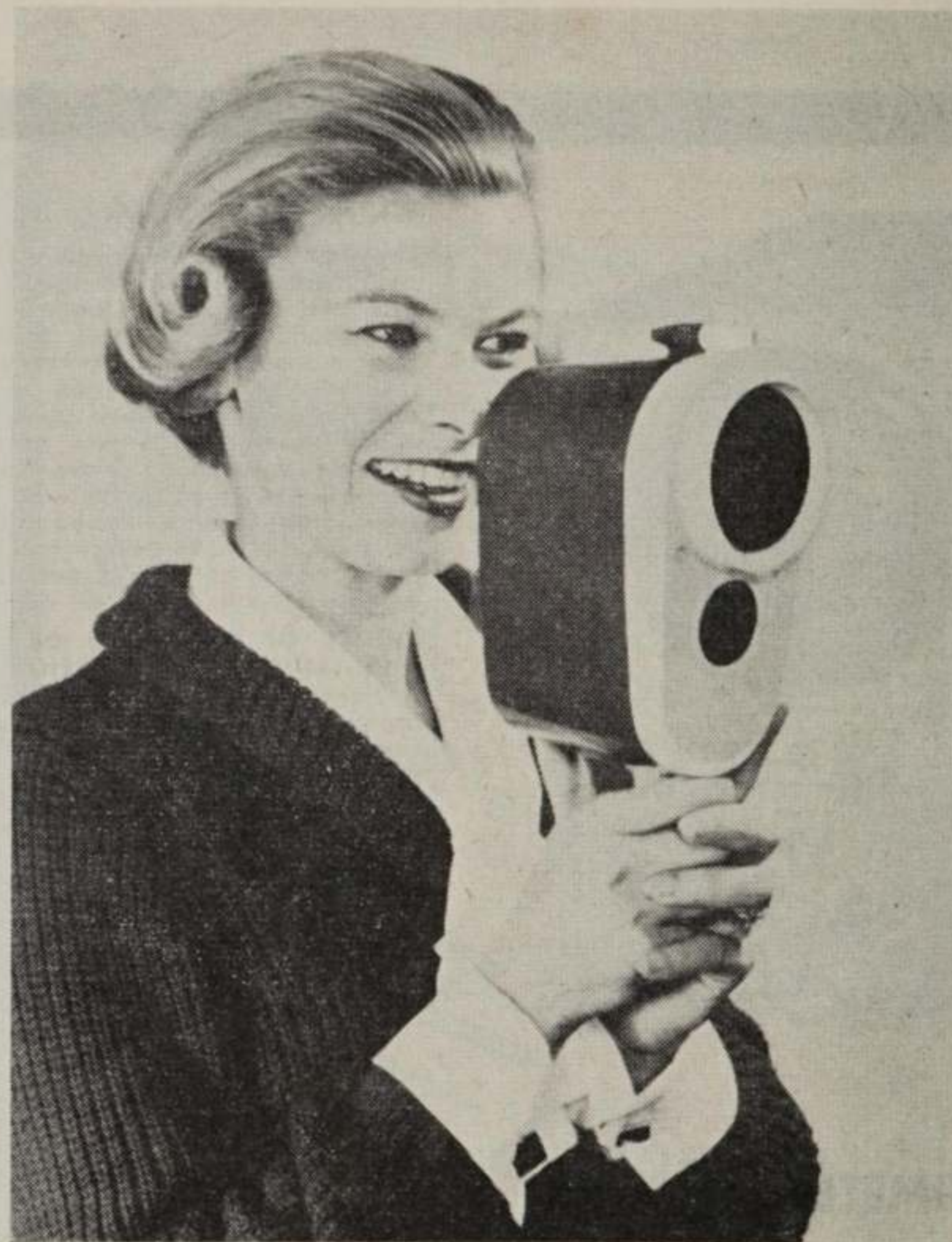
New Infrared Industries, Inc. Infraphone uses invisible infrared ray to send telephone-like conversations hundreds of yards without wires. Instrument is completely "solid state", utilizing a fully-transistorized, printed circuit amplifier and semiconductor infrared sensing element. It operates on ordinary flashlight batteries.
