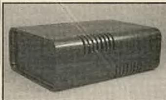
Cleverly designed, this box uses two identical pieces which just snap together to make the box, i.e. does not require any screws for fixing. Includes generous ventilation slots and posts for mounting PCB's etc. Incorporates speaker recess. Includes front and rear panels. 135 x 93 x 47mm
