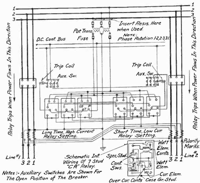
FIG. 2A—PROTECTION FOR A PAIR OF PARALLEL LINES
