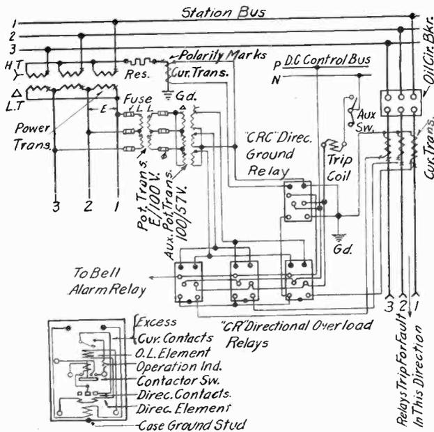
FIG. 11—DIRECTIONAL OVER-LOAD AND DIRECTIONAL GROUND PROTECTION
