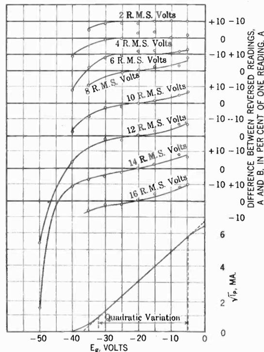
FIG. 13—VARIATION OF WAVE-FORM ERROR WITH BIAS
