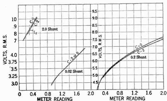
FIG. 7—SAMPLE CALIBRATION VACUUM TUBE VOLTMETER
