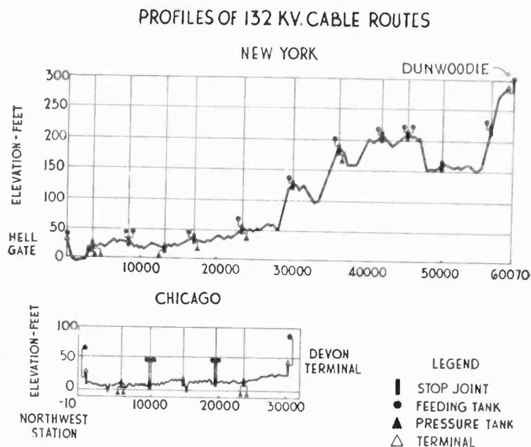
FIG. 9—PROFILES OF 132-KV. CABLE ROUTE
