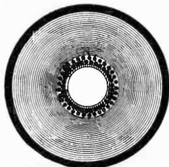
FIG. 1—HOLLOW CORE CABLE
