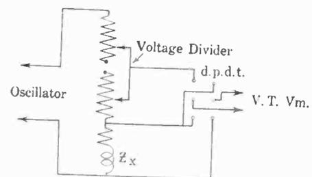
FIG. 11—COMPARISON OF IMPEDANCES USING VACUUM TUBE VOLTMETER
