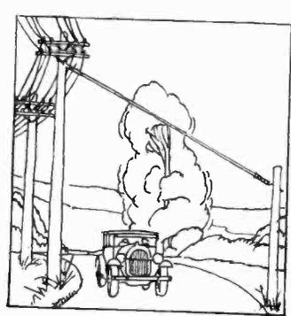
The Gould Clamp can be furnished with shorter lengths of rods where it is desired to attach guys to a tree or guy stud.
