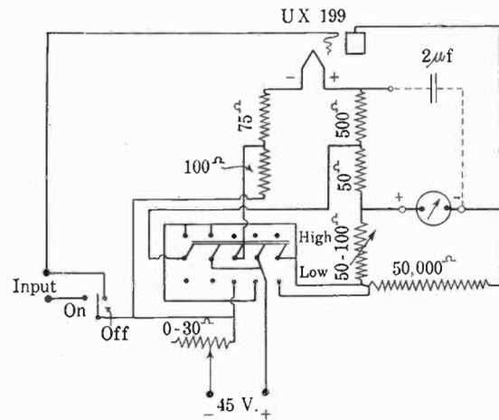
FIG. 3—WIRING DIAGRAM OF ASSEMBLED VOLTMETER
