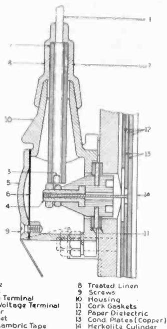
FIG. 3—CROSS-SECTION DRAWING SHOWING METHOD OF BRINGING OUT TERMINAL FROM CAPACITANCE TRANSFORMER
