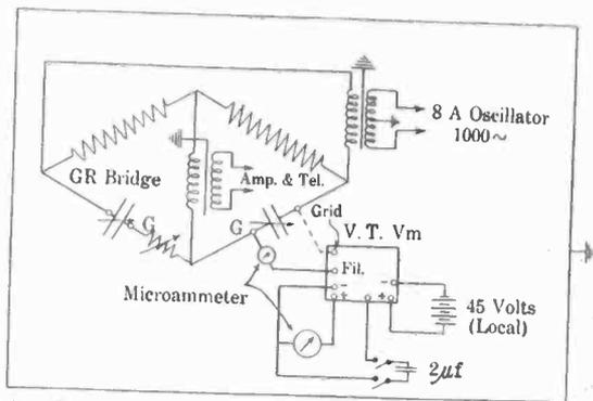
FIG. 10—SCHEMATIC DIAGRAM OF IMPEDANCE BRIDGE
