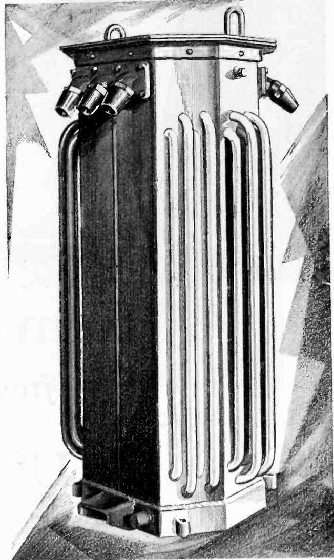
Wagner Subway-type Transformer assembled showing cable-entrance flanges and brass terminal bushings. Wiped joints are made between the lead sheaths of the cables and these bushings. Pressed copper terminals are sweated to the ends of the cable and bolted to studs on terminal board.
