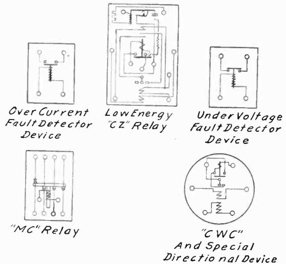
FIG. 15B—INTERNAL WIRING DIAGRAMS
