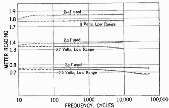
FIG. 9—FREQUENCY CHARACTERISTIC OF VACUUM TUBE VOLTMETER
