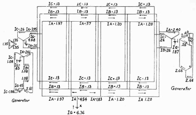
FIG. 7—FAULT-CURRENT DISTRIBUTION DIAGRAM
