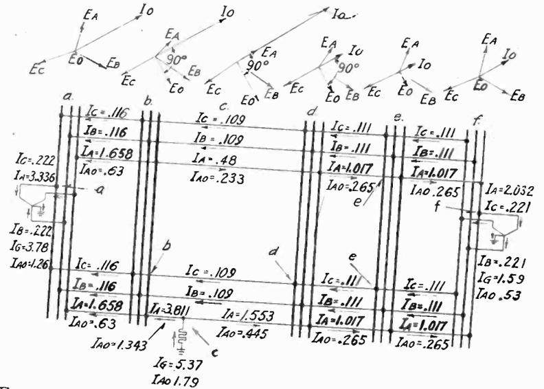
FIG. 10—CURRENT DISTRIBUTION AND VECTOR RELATIONS EXISTING WITHIN RELAYS
