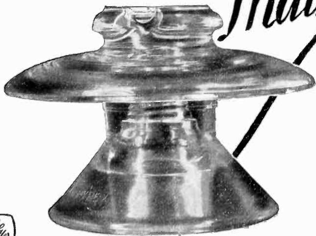
—the logical insulator, representing the TRUE fusion of materials resulting in a non-porous dielectric possessing unalterable uniformity of structure, high in puncture strength and wet flashover, low temperature rise—a rugged one-piece, non-crazing insulator unaffected by any atmospheric condition and one that can be visually inspected clear through to the pin.
