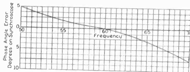
FIG. 12—SYNCHROSCOPE CHARACTERISTIC
