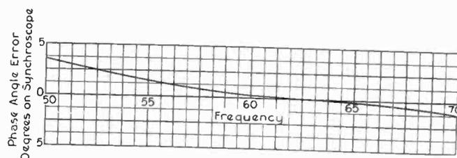
FIG. 13—SYNCHROSCOPE CHARACTERISTIC
