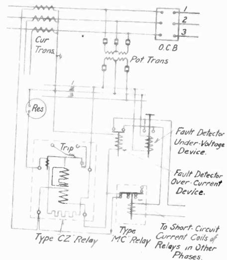
FIG. 4—APPLICATION OF IMPEDANCE RELAYS FOR PROTECTING SYSTEMS WHERE FAULT CURRENT IS LESS THAN FULL-LOAD CURRENT
