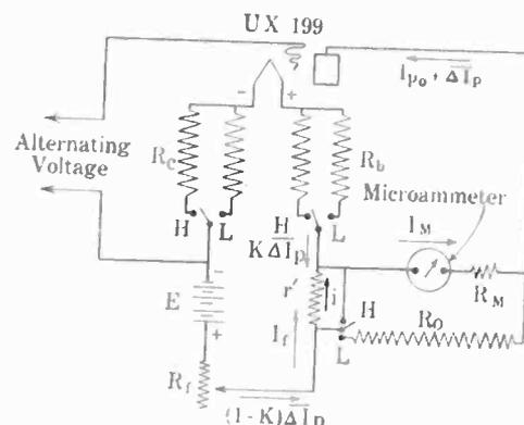
FIG. 1—SCHEMATIC DIAGRAM OF VACUUM TUBE VOLTMETER
