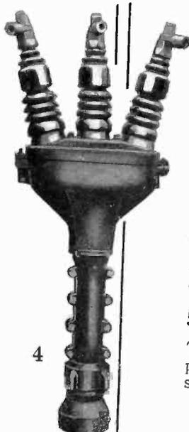
1. A porcelain waterproof enclosure for an S/C fuse. Wiping sleeve connection for lead cable. Designed for manhole use.
