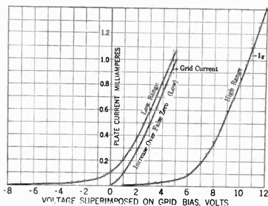
FIG. 14—STATIC CHARACTERISTICS OF VACUUM TUBE VOLTMETER
