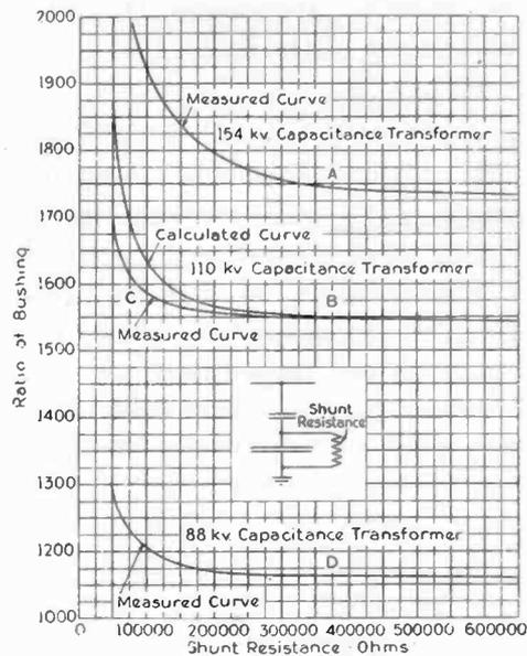
FIG. 9—RATIO CHARACTERISTICS OF CAPACITANCE TRANSFORMERS
