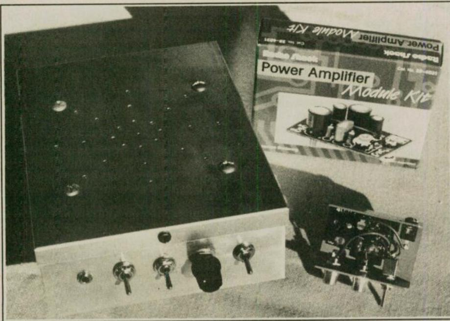
**Radio Shack's Power Amplifier Module Kit is the heart of both the Audio Ratchet, left, and the tiny No Frills Audio unit, right.**
