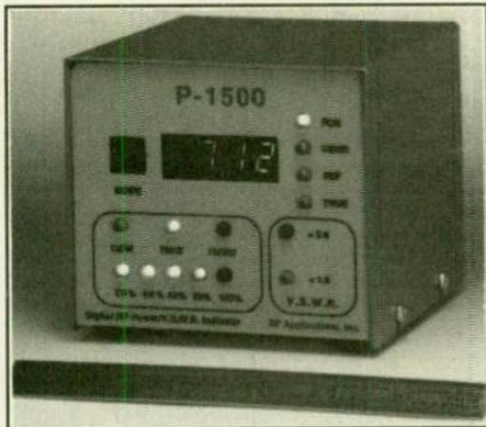
can be displayed. Using a built-in sensor, the P-1500 automatically selects from three ranges (0-120 W, 0-750 W, and 0-1500 W), so there are no range switches. Frequency coverage is 1.8 to 30 MHz. The P-1500 continuously monitors V.S.W.R., and there are indicators to signal V.S.W.R. over 3.0 and less than 1.5 (even when V.S.W.R. is not selected on the display).
