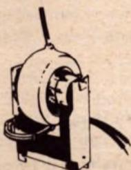
We have thousands of flyback transformers for TV sets, and have worked out an interesting modification of them so that using a pair of power transistors and a few resistors you can build a 12 volt D.C. powered oscillator converter providing an output of 18,000 volts. With this high voltage output you can perform many interesting experiments and demonstrations, such as a jacobs ladder... or
