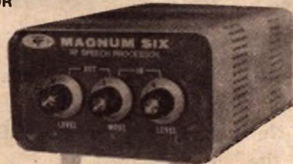
■ The human voice is a "raspy" signal with high peaks and long, low valleys. If used to modulate an SSB transmitter directly, the low power of the valleys limits the average power output to 12-15% of the transmitter's PEP rating. Operating above this level, the peaks overdrive the transmitter, cause band splatter and poor quality.
