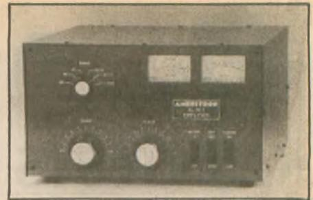
10/12 meters operation requires presentation of valid Amateur license.) A Pi-Network tuned input circuit matches the tubes to 50 ohm excitors. It lets even the fussiest solid state rig perform flawlessly with the Ameritron AL-811.
