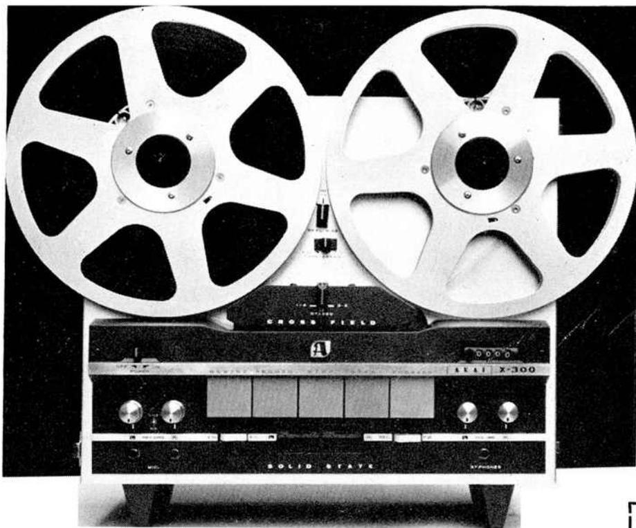
The Akai X 300 is a 4 track stereo/mono studio-type tape recorder. It has 4 heads – erase, record, playback/monitor, and Crossfield; and 3 motors – one hysteresis synchronous direct drive capstan, two torque for fast forward and rewind. It has two speeds – 3¾ ips which will give you 30 to 18,000 cps  $\pm$  3db; and 7½ ips which will give you 30 to 24,000 cps  $\pm$  3 db.
