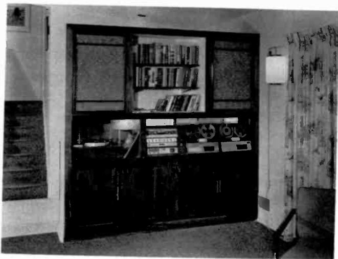
Room divider installation. Behind it is an entrance hall. Installation includes stereo amplifier, stereo tuner, 2 speakers, 2 tape transports and stereo record/playback pre-amplifier. At the flick of a switch, tape recordings can be made from stereo records, stereo FM broadcasts, stereo tapes or stereo microphones. The unique preamplifier (Knight-Kit®) permits sound-on-sound recordings.
