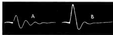
Fig. 27. Shock tests showing effect of magnet. (A) A 10-inch loudspeaker unit with a 10,000-gauss magnet. (B) Same as for part A but with a 14,000-gauss magnet.
