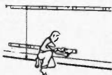
3. SPIKE 2"x3" BACK SUPPORTS TO WALL WITH 16D COMMON NAILS
