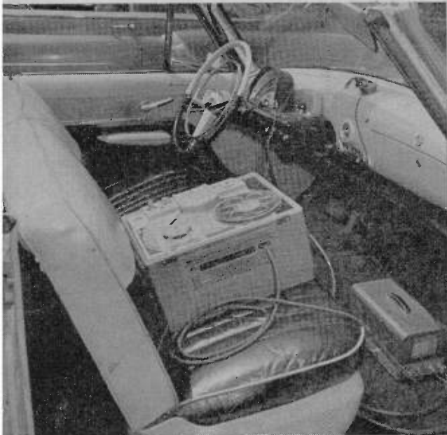
Recorder uses 110 volt current from converter connected to car battery.
