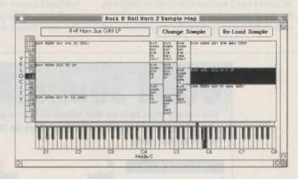
SampleCell's keyboard mapping window. Velocity zones (maximum of three) are shown as vertical stacks. When you play your MIDI keyboard, the screen keyboard will show the note in inverse video. The screen keyboard can also be used to trigger playback.
