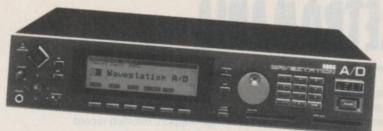
Korg's Wavestation is now available as a rack-mount. The "A/D" in the device's name refers to the fact that it contains analog inputs for external audio signals. These signals can be used as waves by the synth engine and processed through the effects section.
