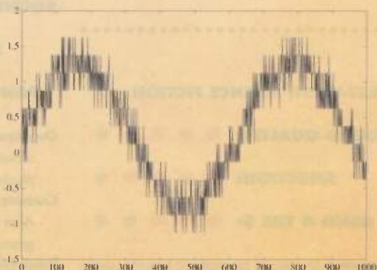
Fig. 4. Quantized dithered signal. The sharp edges of the quantization distortion (Figure 2) have now disappeared.
