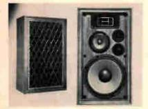
tweeter; response 35-20,000 Hz (reference not stated); 500 Hz and 4500 Hz crossover frequencies; mid-range and tweeter controls on front panel; 8 ohms impedance; 60 watts (dynamic) maximum input power;  $26'' H \times 12^{3}4'' W \times 15'' D$ ; walnut; individual speaker connections to manufacturer's multi-amp system; weight 37 lbs; \$189.00.
