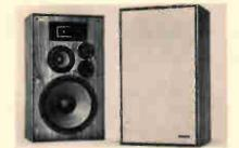
horn-type tweeter; response 35-20,000 Hz (reference not stated); 500 Hz and 4500 Hz crossover frequencies; mid-range and tweeter controls on front panel; 8 ohms impedance; 60 watts (dynamic) maximum input power;  $26'' H \times 15'' W \times 113/4'' D$ ; oiled walnut; individual speaker connections to manufacturer's multiamp system; weight 35 lbs; \$189.00.
