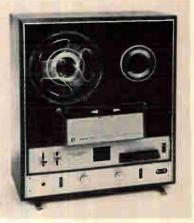
30-20,000 Hz (reference not stated); VU meters; auto reverse; auto shutoff; pause; soundon-sound; sound-with-sound; counter;  $17^{3}/_{4}$ " H x 16" W x 6 $^{3}/_{4}$ " D; 30 lbs; \$219.95.
