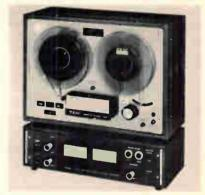
Hz at  $\pm 3.0$  dB; wow & flutter 0.12% at 7<sup>1</sup>/<sub>2</sub> ips; S/N 50 dB; VU meters; auto reverse; auto shutoff; pause; counter; solenoid operation; separate tape transport and electronics cabinets; monitoring; also available with 4 heads for 4 channel operation, 4 VU meters, 3 cabinets (\$695.00); 16<sup>3</sup>/<sub>4</sub>" H × 17<sup>1</sup>/<sub>2</sub>" W × 7<sup>1</sup>/<sub>4</sub>" D; 46 lbs; \$535.00.
