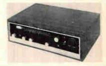
QR-500 will include both a 4-channel "decoder" and a 4-channel "synthesizer." The decoder will be used to de-matrix 4-channel broadcasts while the synthesizer will be used to convert standard stereo broadcasts, discs and other 2channel program sources into a synthesized 4 channel program.
