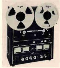
heads; response 30-22,000 Hz at  $\pm$ 2.0 dB; wow & flutter 0.04% at 7<sup>1</sup>/<sub>2</sub> ips; S/N 56 dB; braking; four VU meters; auto shutoff; pause; sound-onsound; bias adjustment; counter; remote (optional extra); dust cover; monitoring; solenoid operation; 22" H × 17<sup>5</sup>/<sub>9</sub>" W × 10" D; 61 lbs; \$1595.00.
