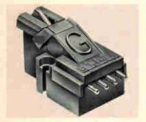
special stylus with 0.3-mil spherical tip contacting groove walls; tracking force  $0.7 \rightarrow 2.0$  g; channel separation nominally 35 dB at 1000 Hz; stylus replacement # F1/S; price \$75.00.
