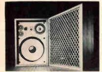
per mid-ranges, 3" cone tweeter, and two dometype  $3\frac{1}{2}$ " tweeters; response 20-23,000 Hz (reference not stated); 600, 5000, 10,000, and 15,000 Hz crossover frequencies; mid-range and tweeter controls; 8 ohms impedance; 80 watts (dynamic) maximum input power;  $24\frac{1}{2}$ " H  $\times$  17" W  $\times$  11<sup>1</sup>/4" D; walnut; weight 49 lbs; \$214.95.
