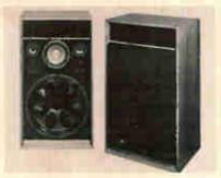
upper mid-range, and two 2" tweeters; re-sponse 20-20,000 Hz (reference not stated); 400, 1000 and 5000 Hz crossover frequencies: mid-range and tweeter controls; 8 ohms impedance 100 watts (peak) maximum input power; 295/16" H × 175/16" W × 153/8" D; walnut; weight 57 lbs; \$299.95.
