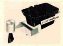
stylus 0.3 x 0.7 mil elliptical; tracking force  $3/4 \rightarrow 13/4$  g; channel separation nominally 30 dB; special feature: Dustamatic brush, stylus replacement # DIV-AME; price \$49.95.
