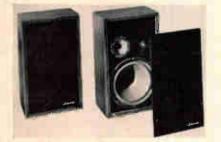
sion 31/2" tweeter; response 28-22,000 Hz (reference not stated); 600 Hz and 5000 Hz crossover frequencies; mid-range and tweeter controls; 8 ohms impedance; requires 10 watts (dynamic) driving power; 60 watts (dynamic) maximum input power; 24" H × 14" W × 9" D; oiled walnut; weight 36 lbs; \$129.95.
