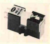
frequency response 10-24,000 Hz at  $\pm 2$  dB; three interchangeable styli assemblies  $-0.3 \times 0.7$  mil elliptical, 0.3  $\times 0.9$  mil elliptical, and 0.6 mil spherical; tracking force  $\frac{1}{2} \rightarrow \frac{1}{4}$  g; 15° tracking angle; channel separation nominally 30 dB from 50-15,000 Hz; compliance 50  $\times 10^{-6}$  cm/dyne; IM distortion less than  $\frac{1}{2}$ % 400-4,000 Hz at 14.3 cm/sec; Price \$100.00.
