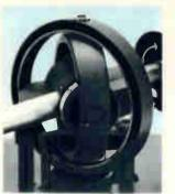
Unique gyroscopic gimbal suspension centers and balances tonearm within two concentric rings. All four pivots have identical low-friction, hardened steel-point bearings. Vertical friction less than 0.007 gram, horizontal friction less than 0.015 gram.
