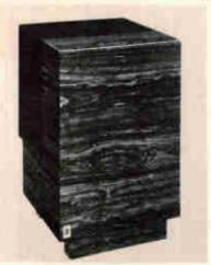
and two wide dispersion  $2^{1}/2^{n}$  tweeters; frequency response 28-18,000 Hz (reference not stated): mid-range and tweeter level controls; 6 ohms nominal impedance; 60 watts (dynamic) maximum input power; dimensions 25" H × 16 $^{1}/_{4}$ " W × 16 $^{1}/_{4}$ " D; walnut formica finish; features reflecting from wall sound dispersion with acoustic lens; approximate weight 75 lbs; price \$300.00.
