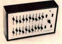
controls with ±12 dB variation; two-channel design with switchable input sensitivity 350 mV to 1.4 V rms; HD less than 0.5%; IM distortion less than 0.2%; S/N better than 60 dB; maximum output 4.5 V; 7%" x 12" x 12" x 3%" D; \$225.00.
