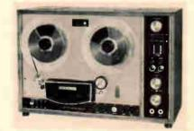
Hz (reference not stated): wow & flutter <0.07% at 7½ ips; S/N >50 dB: VU meters; auto reverse; auto shutoff; pause; echo effects; sound-on-sound; sound-with-sound; counter; solenoid controls: monitoring;  $141/_2$ " H × 21" W ×  $101/_2$ " D; 40 lbs: \$459.95.
