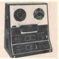
30-25,000 Hz at  $\pm$ 3.0 dB; wow & flutter 0.09% at 7½ ips; S/N 55 dB; VU meters; auto shutoff; pause; counter; monitoring; slanted upright base; also available as a two-track (7½ & 3¼ ips) 4 channel Model 366-4-\$499.95; 167/16" H x 14<sup>13</sup>/16" W × 8<sup>5</sup>/16" D; 22<sup>1</sup>/2 lbs; \$239.95.
