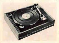
manual/changer combo; variable speed; cueing control; tracking angle adjustment; 0.05% wow;  $0 \rightarrow 6\frac{1}{3}$  g stylus pressure adjustment; removable cartridge shell; overhang adjustment; elapsed time indicator;--42 dB rumble;  $9\frac{1}{2}$ " Hx 14 $\frac{1}{2}$ " Wx 12 $\frac{1}{2}$ " D; molded base \$5.95. \$225.00.
