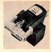
quency response 20-20,000 Hz (reference not stated); stylus 0.7 mil spherical; tracking force  $1 \rightarrow 3$  g; channel separation nominally 22 dB at 1000 Hz; compliance  $18 \times 10^{-6}$  cm/dyne; (Model STS-244-E has 0.2  $\times$  0.8 mil elliptical stylus at \$35.00); price \$24.95.
