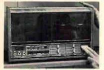
flutter 0.25%; hysteresis motor; S/N 45 dB; supplied with mikes; supplied with speakers; VU meters; counter: eject button; tone controls; pause; monitoring; mike & line inputs; phono input; dust cover; also available without tuner as Model 87–\$219.95;  $10^{1/a''}$  H ×  $13^{3/a''}$  W ×  $6^{3/a''}$  D; walnut; \$299.95.
