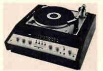
mag. cartridge; diamond stylus; Dustamatic brush; 35 W/channel continuous sine-wave into 8 ohms with both channels driven at 0.5% THD; 57 W/channel dynamic power at 8 ohms; 75 W/channel into 4 ohms; power bandwidth 18-30,000 Hz; response 13-70,000 Hz  $\pm$ 1.5 dB; AM-Stereo FM tuner section with 1.8  $\mu$ V FM sensitivity for 30 dB quieting; capture ratio 2.5 dB (IHF); main/remote speaker switch; control center 171/4" x 8" x 18" D; without speakers; oiled walnut cabinet; \$349.95
