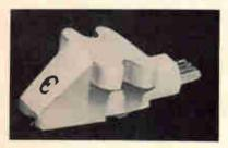
tracking force  $1.0 \rightarrow 2.0$  g;  $15^{\circ}$  tracking angle; channel separation nominally 30 dB at 1000 Hz; compliance 25 × 10 ° cm/dyne; requires 12volt dc power supply (\$19.00); price \$36.00.
