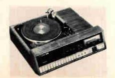
FM receiver section (their Model 714A); Starr cassette recorder/playback; recorder response 50-10,000 Hz; control center  $211/2^{"} \times 67/8^{"} \times$  $191/2^{"}$  D; has mike input; (Model 911A without cassette recorder \$499.00); walnut; \$650.00
