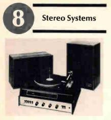
stylus; 16 W/channel dynamic power amplifier; AM-FM tuner section with 1.6  $\mu$ V FM sensitivity for 20 dB quieting; pair of EMI speaker systems; power bandwidth 25-30,000 Hz; response 10-100,000 Hz  $\pm 1$  dB; speaker cabinets  $16^{1/4''} \times$  $11^{1/4''} \times 8^{1/4''}$  D; 8" woofer &  $3^{3/6''}$  tweeter; control center  $9^{7/6''} \times 16^{5/6''} \times 16^{5/6'''}$  D; dust cover optional; \$329.50
