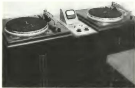
Fig. 2 — Dubbing and playback tables, mounted on special rubber cups and cork sheeting to eliminate building vibration.
