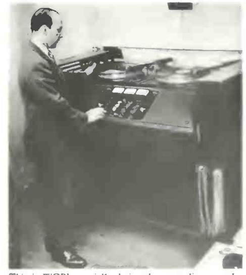
This is WOR's specially designed re-recording console, with which it is possible to make disc "copies" which are actually superior in quality to the original.
