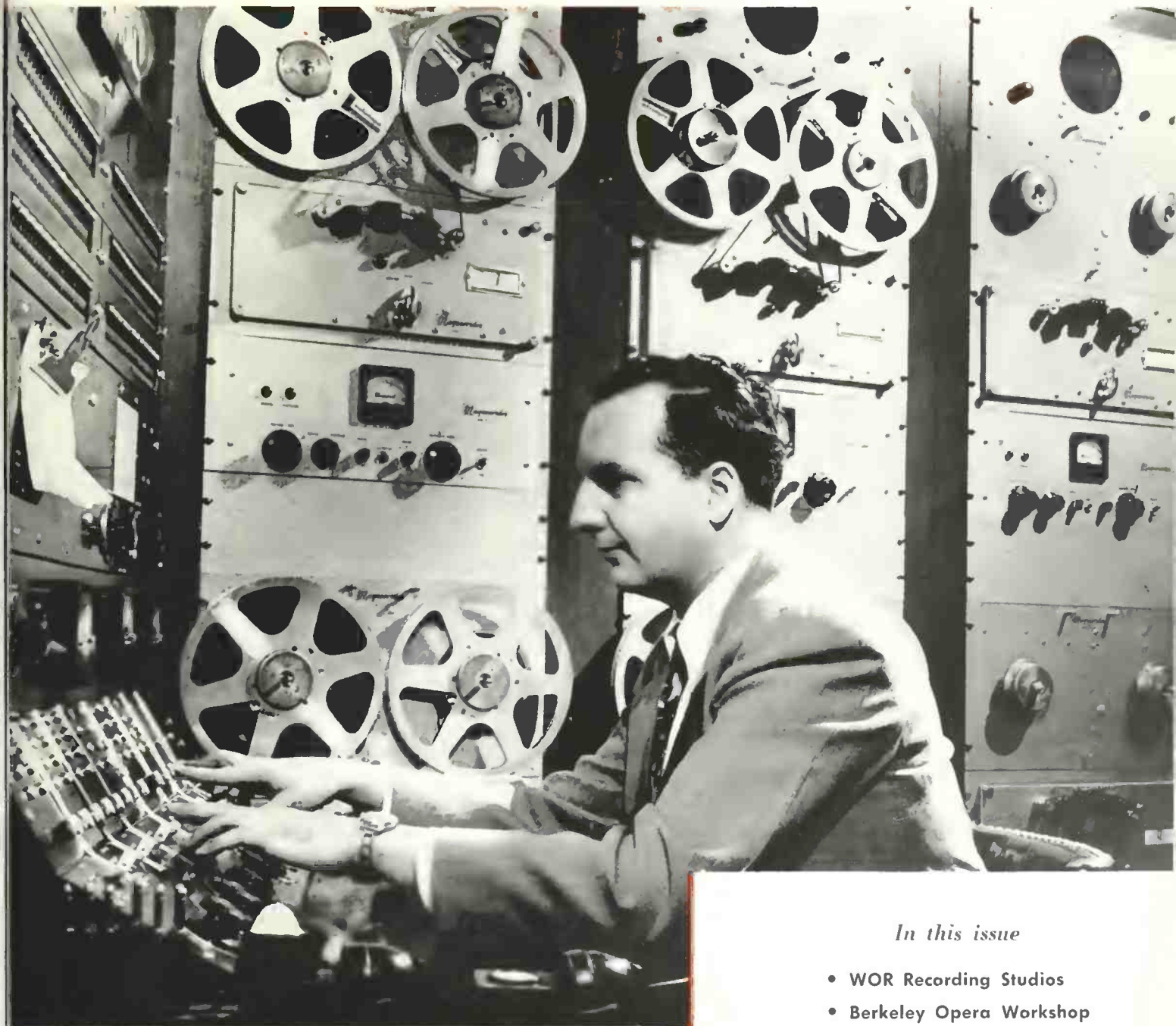
A portion of the "Mutual Room" at WOR Recording Studios, showing 6 of the 12 rack-mounted Magnecorders and the specially designed central control panel for all machines. Here every Mutual program is taped and re-transmitted one hour later during daylight saving time. Story on Page 2.
